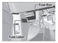
Fuse locations are shown on the label on the outer side of the side panel cover. Locate the fuse in question by the fuse number and label number.
