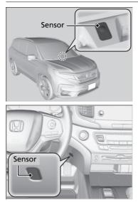
The automatic climate control system is equipped with sensors. Do not cover or spill any liquid on them. This page intentionally left blank.
