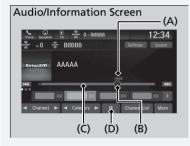
(A): Shows how much time the replayed segment is behind the real-time broadcast
