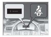
The seat belt system includes an indicator on the instrument panel to remind the driver or a front passenger or both to fasten their seat belts.
