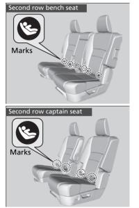
**1.** Locate the lower anchors under the marks.
