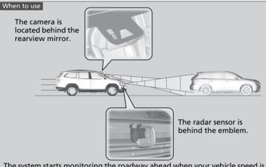
The system starts monitoring the roadway ahead when your vehicle speed is about 3 mph (5 km/h) or above and will search for a vehicle in front of you.
