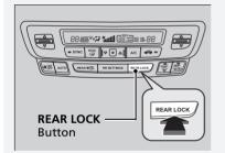
Press the **REAR LOCK** button to turn the rear lock mode on and off.
