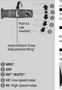
The windshield wipers and washers can be used when the power mode is in ON.
