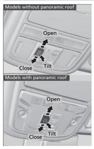
Automatic operationTo open: Pull the switch back firmly.To close: Push the switch forward firmly.
