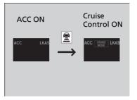
Press and hold the  $\boxed{\blacksquare}$  (interval) button for one second. **Cruise Mode Selected** appears on the driver information interface for two seconds, and then the mode switches to Cruise.
