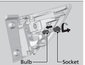
**3.** Turn the socket counter-clockwise and remove it. Remove the old bulb.
