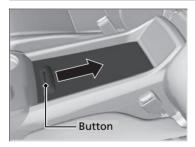
To open the console compartment, press the button to unlock the lid, and then slide it rearward.
