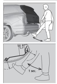
Use a forward and back kicking motion for about 1 second under the center of the rear bumper to open or close the power tailgate while carrying the keyless remote.
