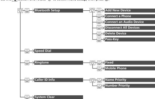
Press the 📞 button and rotate 😙 to select Phone Setup, then press 🕹.
