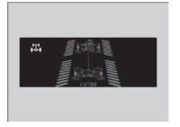
The indicators on the display show the amount of torque being transferred to the right front, left front, right rear, and left rear wheels.
