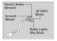
The trailer hitch harness is used to install the controller for the electric trailer brakes. Insert the trailer brake fuse into the engine compartment sub fuse box. Engine Compartment Fuse Box Type B
