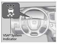
When VSA<sup>®</sup> activates, you may notice that the engine does not respond to the accelerator. You may also notice some noise from the hydraulic brake system. You will also see the indicator blink.
