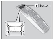
Park your vehicle in a safe place with the power mode in ON, then apply the brakes and press the  $\boxed{P}$  button to put the transmission in Park.
