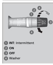
The rear wiper and washer can be used when the power mode is in ON.
