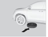
**9.** Place the compact spare tire (wheel side up) under the vehicle body, near the tire that needs to be replaced.
