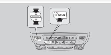
You can set the temperature synchronously for the driver side, front passenger side and rear seats in synchronization mode.
