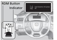
Press the RDM button to turn the system on and off.
