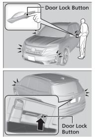
Press the door lock button on a front door or the tailgate.
