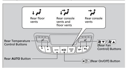
Use the system when the engine is running and the climate control system is operating.
