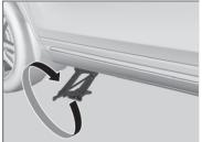
**1.** Place the jack under the jacking point closest to the tire to be changed.
