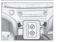
The seat heaters or ventilators can be used when the power mode is in ON. The seat heaters: Use them to warm up the seat.
