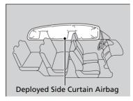
The side curtain airbag is designed to deploy in a rollover or a moderate-to-severe side impact. Safe Driving
