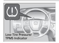
Monitors the tire pressure while you are driving. If your vehicle's tire pressure becomes significantly low, the Low Tire Pressure/TPMS indicator comes on and a message appears on the driver information interface.
