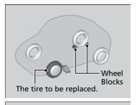
**8.** Place a wheel block or rock in front and rear of the wheel diagonal to the flat tire.
