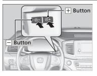
When the power mode is in ON, you can use the + or button to adjust instrument panel brightness. Brighten: Press the + button. Dim: Press the button.
