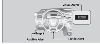
You can change the distance (**Long/Normal/Short**) between vehicles at which the system's earliest collision alert will come on through the driver information interface or the audio/information screen setting options.
