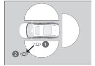
When you walk away from the vehicle with all doors and tailgate closed while carrying the keyless remote, the doors will automatically lock.
