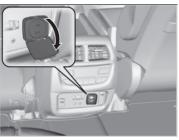
Open the cover to use it. Plug in the appliance slightly, turn it 90° clockwise, then push it all the way.
