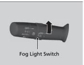
When the parking lights or the headlights are on, turn the fog light switch on to use the fog lights.
