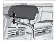
A passenger sitting in the second and third row center seating position should adjust the height of their head restraint to an appropriate position before the vehicle begins moving. **To raise the head restraint:** Pull it upward.
