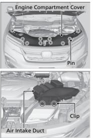
**1.** Pull up on the engine compartment cover, remove it from the pins.
