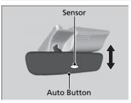
When you are driving after dark, the automatic dimming rearview mirror and power door mirror reduce the glare from headlights behind you. Press the AUTO button to turn this function on and off. When activated, the AUTO indicator comes on.
