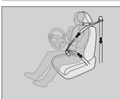
The front seats are equipped with automatic seat belt tensioners to enhance safety.
