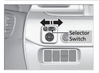
If activated, either side door mirror automatically tilts downward when you put the transmission into  $[\mathbf{R}]$ ; this improves closein visibility on the selected side of the vehicle when backing up. The mirror automatically returns to its original position when you take the transmission out of  $[\mathbf{R}]$ .
