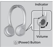
To turn on the switch: Press the (b) (power) button at the right earpiece. The indicator comes on.
