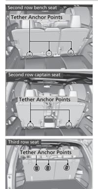
A tether anchor point is provided behind each second and third row seating position. If you have a child seat that comes with a tether but can be installed with a seat belt, the tether may be used for additional security.
