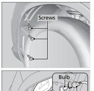
**1.** Remove the screws, pull the inner fender back.
