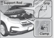
**4.** Remove the support rod from the clamp using the grip. Mount the support rod in the hood.
