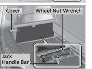
**2.** Pull and remove the cover. Take the wheel nut wrench and jack-handle bar out of the rear side compartment.
