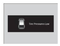
**Tire Pressures Low** is displayed when a tire has significantly low pressure. The specific tire is displayed on the screen.
