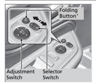
You can adjust the door mirrors when the power mode is in ON.
