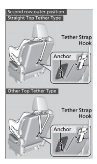
**2.** Put the head restraint to its upper-most position, then route the tether strap outside/through the head restraint legs. Make sure the strap is not twisted.
