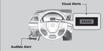
You can change the distance (**Long/Normal/Short**) between vehicles at which the system's earliest collision alert will come on through the driver information interface\* or audio/information screen\* setting options.
