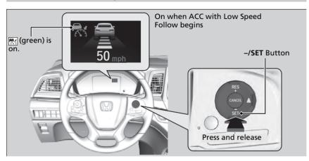
When driving at about 25 mph (40 km/h) or above: Take your foot off the pedal and press down the –/SET button when you reach the desired speed. The moment you release the button, the set speed is fixed, and ACC with Low Speed Follow begins.
