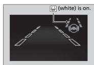
When the LKAS is suspended, the lane lines on the driver information interface change to contour lines, and the beeper sounds (if activated).
