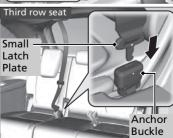
**2.** Line up the triangle marks on the small latch plate and anchor buckle.
