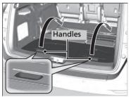
**1.** Grab the handle from outside. Pull up the folded seat, begin to pivot it forward, then allow it to drop into position.
