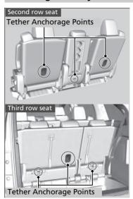
A tether anchorage point is provided behind each second and third row seating position. If you have a child seat that comes with a tether but can be installed with a seat belt, the tether may be used for additional security.
