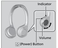
To turn on the switch: Press the (b) (power) button at the right earpiece. The indicator comes on.
