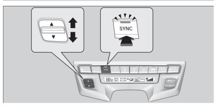
You can set the temperature synchronously for the front compartment and the rear passenger compartment in synchronization mode.
