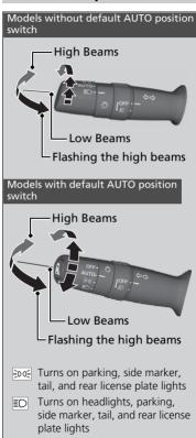
Rotating the light switch turns the lights on and off, regardless of the power mode setting.
