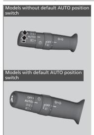
Automatic lighting control can be used when the power mode is in ON.
