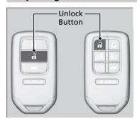
**To open:** Press the unlock button, and then within 10 seconds, press it again and hold it. If the windows stop midway, repeat the procedure.
