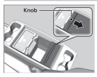
To open the console compartment, press the knob to unlock the lid, and then slide it rearward.
