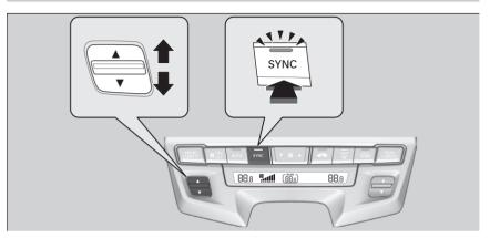
You can set the temperature synchronously for the driver's side, the passenger's side and the rear passenger compartment in synchronization mode.
