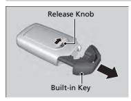
The built-in key can be used to lock/unlock the doors and tailgate when the keyless remote battery becomes weak and the power door lock/unlock operation is disabled.
