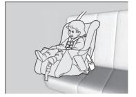
■ Forward-facing child seat placement We strongly recommend placing a forward-facing child seat in a rear seating position.
