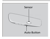
When you are driving after dark, the automatic dimming rearview mirror and power door mirrors\* reduces the glare from headlights behind you. Press the auto button to turn this function on and off. When activated, the auto indicator comes on.
