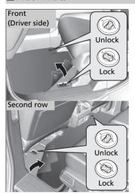
The front and second row floor mats hook over floor anchors, which keep them from sliding forward. To remove a mat for cleaning, turn the anchor knobs to the unlock position. When reinstalling the mat after cleaning, turn the knobs to the lock position.
