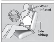
When the sensors detect a moderate-tosevere side impact, the control unit signals the side airbag on the impact side to immediately inflate
