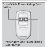
Press the power sliding door button for more than one second to operate.
