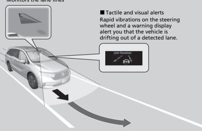
When you operate the turn signals to change lanes, the system is suspended, and resumes after the signals are off.
