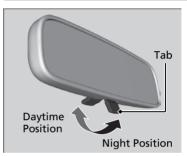
Flip the tab to switch the position. The night position will help to reduce the glare from headlights behind you when driving after dark.
