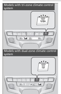
Press the rear defogger and heated door mirror\* button to defog the rear window and mirrors\* when the power mode is in ON.
