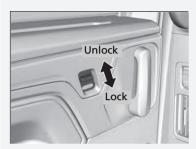
To open the door from the inside when the childproof door lock is on, put the lock tab in the unlock position, lower the rear window, put your hand out of the window, and pull the outside door handle
