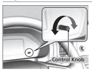
When the power mode is in ON, you can use the brightness control knob to adjust instrument panel brightness.
