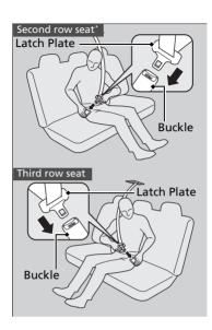
**3.** Insert the latch plate into the buckle. Properly fasten the seat belt the same way you fasten the lap/shoulder seat belt.
