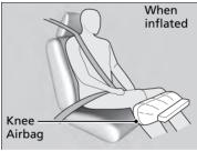
The driver's and front passenger's knee airbag deploy at the same time as the driver's and front passenger's airbag respectively.
