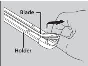
**4.** Pull the wiper blade in the opposite direction to slide it out of the holder.
