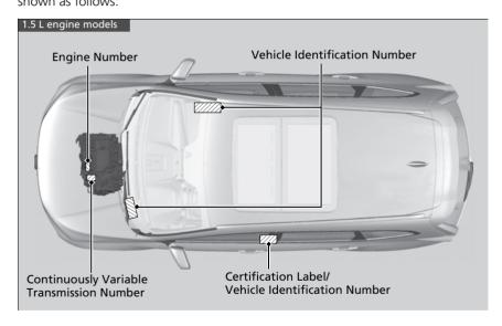
■ Vehicle Identification Number (VIN), Engine Number, and Transmission Number
