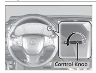
With the parking lights are turned on and the ignition switch is in ON [II]\*1, you can use the brightness control knob to adjust instrument panel brightness.
