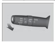
Disable or re-enable the system when the vehicle is parked and the power mode is in ON and the light switch is in the **AUTO** position. **Disabling the system:** Pull the light switch lever towards you and hold it for at least 40 seconds.
