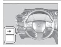
Press the heated windshield button to deice the windshield when the power mode is in ON.
