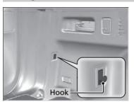
The cargo hooks on the driver's side of the cargo area can be used to hang a light items.
