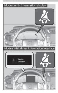
The seat belt system includes an indicator on the instrument panel to remind the driver or a front passenger or both to fasten their seat belts.
