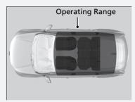
You can start the engine when the smart entry remote is inside the vehicle.
