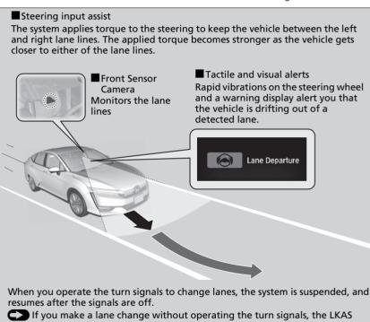
alerts activate, and torque is applied to the steering.
