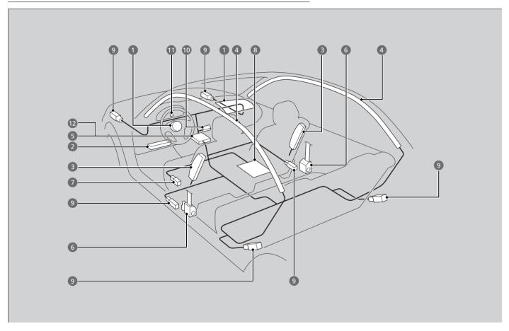
The front, driver's knee, front side, and side curtain airbags are deployed according to the direction and severity of impact. Both side curtain airbags are deployed in a rollover. The airbag system includes:
