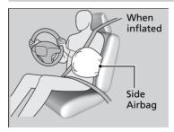
When the sensors detect a moderate-tosevere side impact, the control unit signals the side airbag on the impact side to immediately inflate.
