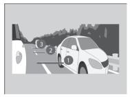
Three lines that appear on the screen can give an idea of how far the vehicles or objects on the screen are from your vehicle, respectively. If an object is near line 1 (in red), it indicates that it is close to your vehicle whereas an object near line 3 farther away.
