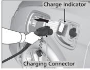
**6.** To connect the cable to the vehicle, push the cable's charging connector until it clicks to the charge lid.
