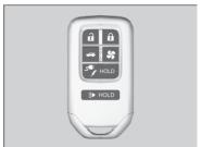
Use the keys to turn on and off the power system, and to lock and unlock the doors and to open the trunk. You can also use the remote transmitter to lock and unlock the doors and trunk, and open the charge lid.
