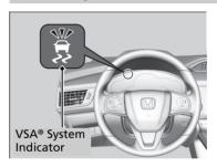
When VSA® activates, you may notice that the engine and motor do not respond to the accelerator. You may also notice some noise from the hydraulic system. You will also see the indicator blink.
