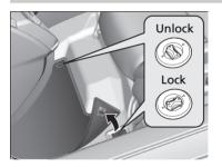
The front and rear floor mats hook over floor anchors, which keep them from sliding forward. To remove a mat for cleaning, turn the anchor knobs to the unlock position. When reinstalling the mat after cleaning, turn the knobs to the lock position.
