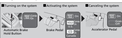
Fasten your seat belt properly, then start the power system. Press the automatic brake hold button.
