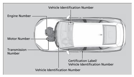
Vehicle Identification Number (VIN), Engine Number, Motor Number, and Transmission Number
