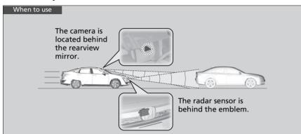
The system starts monitoring the roadway ahead when your vehicle speed is about 3 mph (5 km/h) and there is a vehicle in front of you.
