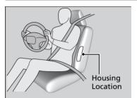
The side airbags are housed in the outside edge of the driver's and passenger's seat-backs.
