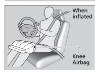
When the driver's front airbag inflates, the driver's knee airbag also inflates.
