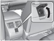
Accessory power socket (back of the console compartment)
