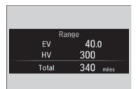
Shows the estimated distance you can travel on the remaining power and fuel. This estimate is based on the fuel economy and energy consumption of your previous trips and the remaining high voltage battery charge level.
