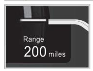
Shows the estimated distance you can travel on the remaining power and fuel. This estimate is based on the fuel economy and energy consumption of your previous trips and the remaining high voltage battery charge level.
