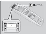
The gear position changes to  $\boxed{\textbf{P}}$  when you press the  $\boxed{\textbf{P}}$  button while the vehicle is parked with the power mode in ON. The indicators on the sides of the  $\boxed{\textbf{P}}$  button come on.
