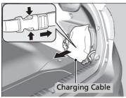
**1.** Remove the charging cable by releasing the belt.
