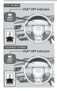
This button is on the driver side control panel. To partially disable VSA® functionality/ features, press and hold it until you hear a beep.
