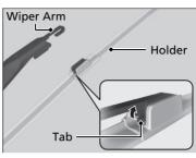
**4.** Press and hold the tab, then slide the holder off the wiper arm.
