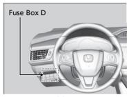
Replacement of fuses in the driver's side outer panel should be done by an authorized Honda Clarity Plug-In Hybrid dealer.
