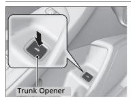
Press and hold the trunk opener on the driver's door to unlock and open the trunk. When You Cannot Open the Trunk P. 699
