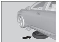
**6.** Place the compact spare tire (wheel side up) under the vehicle body, near the tire that needs to be replaced.
