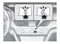
The rear defogger and heated door mirrors automatically switch off after 10-30 minutes depending on the outside temperature. However, if the outside temperature is 32°F (0°C) or below, it does not automatically switch off.
