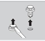
Insert the clip with the pin raised, and push until it is flat.
