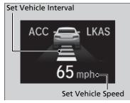
When ACC starts operating, the vehicle icon, interval bars and set speed appear on the driver information interface.
