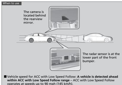
No vehicle is detected within ACC with Low Speed Follow range – ACC with Low Speed Follow operates at the speed of 25 mph (40 km/h) or above. ■ Gear position for ACC with Low Speed Follow: In D or S\*.
