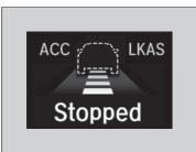
Your vehicle also stops, automatically. The **Stopped** message appears on the driver information interface. When the vehicle ahead of you starts again, the vehicle icon on the driver information interface blinks. If you press the **RES/+** or **SET/** – button, or depress the accelerator pedal, ACC with Low Speed Follow operates again
