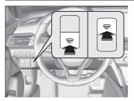
Press the heated windshield button to deice the windshield when the power mode is in ON. Rear Defogger/Heated Door Mirror \* Button
