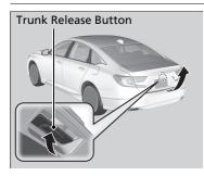
Push up the release button on the trunk lid after all the doors are unlocked.
