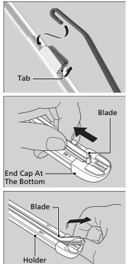
4. Press and hold the tab, then slide the holder off the wiper arm.
