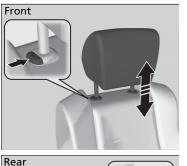
**To raise the head restraint:** Pull it upward. **To lower the head restraint:** Push it down while pressing the release button.
