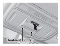
When the parking lights are on, push the ambient light switch to turn the ambient lights on.
