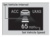
When ACC with Low Speed Follow starts operating, the vehicle icon, interval bars and set speed appear on the driver information interface.
