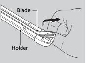
6. Pull the wiper blade in the opposite direction to slide it out of its holder.
