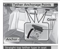
Tether Strap Hook Anchor Other top tether type in seat position with adjustable headrest
