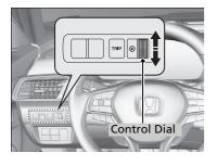
When the power mode is in ON, you can use the brightness control dial to adjust instrument panel brightness. **Brighten:** Turn the dial up. **Dim:** Turn the dial down.
