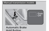
While the system is on, press the automatic brake hold button again.
