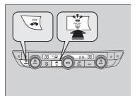
Pressing the mean button turns the air conditioning system on and automatically switches the system to fresh air mode.
