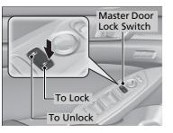
Press the master door lock switch in (as shown) to lock or unlock all the doors, fuel fill door.
