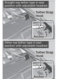
**4.** Open the tether anchor cover behind the head restraint.
