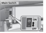
The trunk main switch disables the trunk release button on the remote transmitter and the trunk release button on the trunk lid and trunk opener on the driver's door to protect luggage in the trunk.
