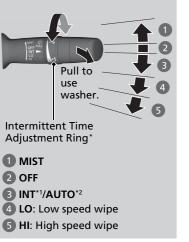
The windshield wipers and washers can be used when the power mode is in ON.
