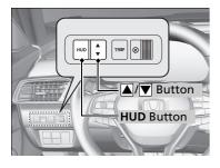
When the head-up display is on, press and hold the **HUD** button until its brightness level indicator on the driver information interface. **Brighten:** Press the button. **Dim:** Press the button.
