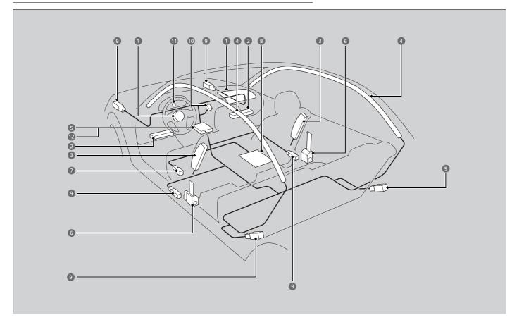
The front, front knee, front side, and side curtain airbags are deployed according to the direction and severity of impact. Both side curtain airbags are deployed in a rollover. The airbag system includes:
