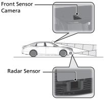
The radar sensor is at the lower part of the front bumper.
