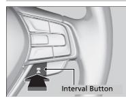
Press the (interval) button to change the ACC following interval. Each time you press the button, the following interval (the interval behind a vehicle detected ahead of you) setting cycles through extra long, long, middle, and short following intervals.
