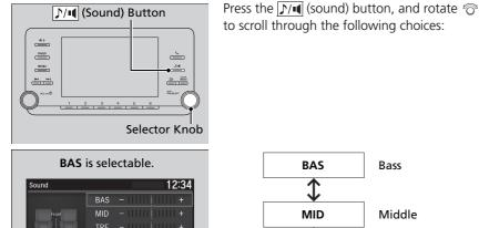
BAS Bass 1 MID Middle 1 TRE Treble 1 FAD Fader 1 BAL Balance 1 Speed-sensitive SVC Volume Compensation
