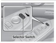
If activated, passenger's side door mirror automatically tilts downward when you put the transmission into  $[\mathbf{R}]$ ; this improves closein visibility on the passenger's side of the vehicle when backing up. The mirror automatically returns to its original position when you take the transmission out of  $[\mathbf{R}]$ .
