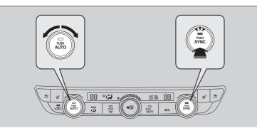
You can set the temperature synchronously for the driver side and the passenger side in synchronization mode.
