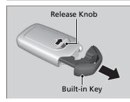
The built-in key can be used to lock/unlock the doors or open the trunk when the remote battery becomes weak and the power door lock/unlock operation is disabled.
