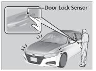
When you carry the remote, you can lock/ unlock the doors, fuel fill door, and open the trunk.
