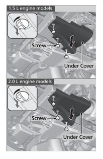
**5.** Remove the slotted head screws by turning 90° counterclockwise on the undercarriage and remove the under cover.
