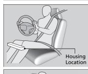
The driver's knee airbag is housed under the steering column.
