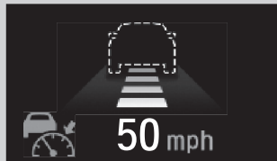
A vehicle icon with dotted-line contour appears on the driver information interface
