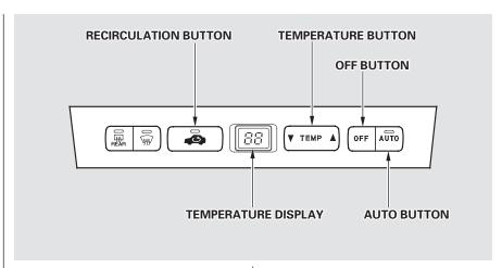
not regulate the interior temperature. When the temperature is set between the lower and upper limits, the system regulates the interior temperature to the set value.
