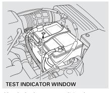
Check the battery condition by looking at the test indicator window on the battery.
