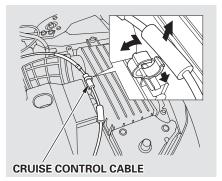
5. Before removing the reserve tank, remove the cruise control cable from its clip, then remove the ground cable from the clip on the reserve tank. To remove the cruise control cable, pivot the upper part of the clip and push down the lower part slightly.
