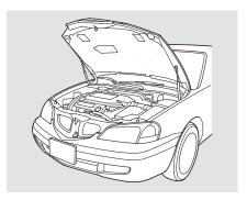
3. Lift the hood up most of the way. The hydraulic supports will lift it up the rest of the way and hold it up.
