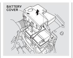
To remove the battery cover, pull up on the right side of the cover to remove it from the bolt, then pull the cover out.
