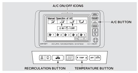
When you turn the A/C off, the system cannot regulate the inside temperature if you set it below the outside temperature. With the A/C off, use the temperature buttons to adjust the temperature of the air flow to a comfortable setting.
