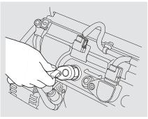
7. Torque the spark plug. (If you do not have a torque wrench, tighten the spark plug two-thirds of a turn after it contacts the cylinder head.) Tightening torque:
