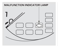
This indicator comes on when you turn the ignition switch ON (II) and goes off after the engine starts. If it comes on at any other time, it indicates one of the engine's emissions control systems may have a problem. Even though you may feel no difference in your car's performance, it can reduce your fuel economy and cause your car to put out excessive emissions. Continued operation may cause serious damage.
