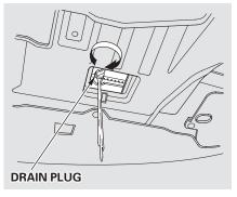
3. Loosen the drain plug on the bottom of the radiator. The coolant will drain through the splash guard. Drain the coolant into an appropriate container.
