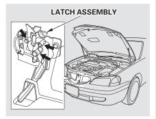
Clean the hood latch assembly with a mild cleaner, then lubricate it with a multipurpose grease. Lubricate all the moving parts (as shown), including the pivot. Follow the time and distance recommendations in the Maintenance Schedule. If you are not sure how to clean and grease the latch, contact your Acura dealer.
