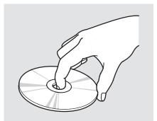
Handle a CD by its edges; never touch either surface. Do not place stabilizer rings or labels on the CD. These and contamination from fingerprints, liquids, and felt-tip pens can cause the CD to not play properly, or possibly jam in the drive.
