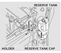
6. Remove the reserve tank from its holder by pulling it straight up. Drain the coolant into an appropriate container, then put the tank back in its holder.
