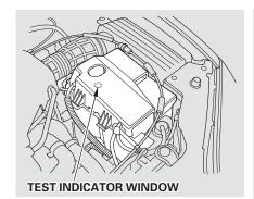
Check the condition of your car's battery monthly. You should check the color of the test indicator window, and for corrosion on the terminals.
