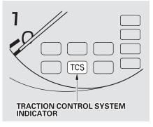
Driving with TCS requires no special skills or technique. The TCS does not control your car's whole braking system and cannot prevent skidding if you enter a corner too fast. It is still your responsibility to drive at reasonable speeds and to leave a sufficient margin of safety.
