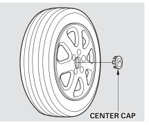
16.Remove the center cap before storing the flat tire in the trunk well.
