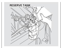
16.If necessary, fill the reserve tank to the MAX mark. Install the reserve tank cap.
