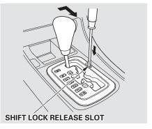
6. Remove the screwdriver from the Shift Lock Release slot, then reinstall the cover. Make sure the notch on the cover is on the right side. Depress the brake pedal and restart the engine.
