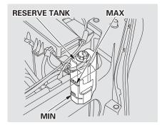
Look at the coolant level in the radiator reserve tank. Make sure it is between the MAX and MIN lines. If it is below the MIN line, see **Adding Engine Coolant** on page 223 for information on adding the proper coolant.
