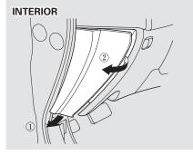
The interior fuse boxes are located on each side of the dashboard. To open an interior fuse box, open the car door. Pull the bottom of the cover open, then take it out of its side hinges by pulling it toward you.
