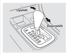
Even with the Sequential SportShift Mode selected, the transmission will automatically upshift and downshift between first and second gear.
