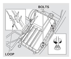
On Type-S Loosen the two bolts with a Phillips-head screwdriver. Remove the air cleaner housing cover by lifting and pivoting it out of the loops.
