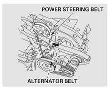
Check the condition of the two drive belts (power steering belt and alternator belt). Examine the edges of each belt for cracks or fraying.
