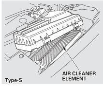
6. On Premium model Reinstall the air cleaner housing cover, tighten the four bolts.
