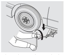
14.Lower the car to the ground and remove the jack.
