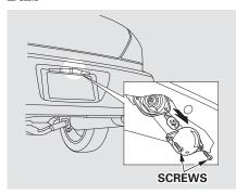
1. Use a small Phillips-head screwdriver to remove the two screws. Remove the lens from the license plate assembly.
