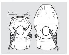
Your car has a Supplemental Restraint System (SRS) with front airbags to help protect the heads and chests of the driver and a front seat passenger during a moderate to severe frontal collision.
