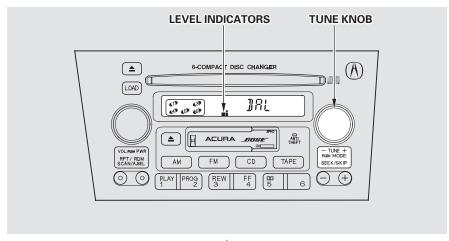
Select BAL or FAD by pressing the TUNE knob. Adjust the Balance or Fader to your liking by turning the TUNE knob. The level indicators on the display show you the range.
