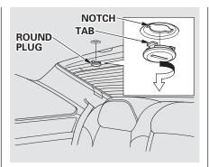
4. To remove the round plug in the center of the headliner, turn the plug by using a screwdriver or coin and pry it off. Make sure to align the tabs on the round plug to the notches on the ceilling as shown in the illustration.
