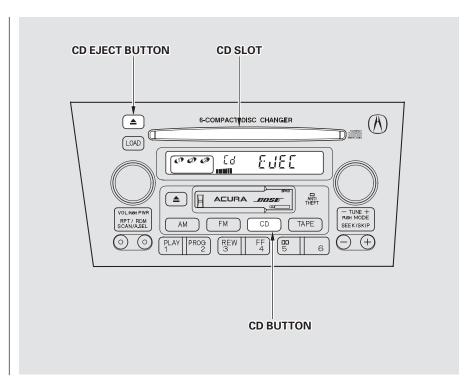
If you press the Eject button while listening to the radio or tape, or with the audio system turned off, the disc that was last selected is ejected. After that disc is ejected, pressing the Eject button again will eject the next disc in the numerical order. By doing this six times, you can remove all the CDs from the changer.
