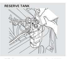
10. Fill the reserve tank to the MAX mark. Install the reserve tank cap.
