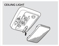
The courtesy lights in the doors and roof come apart the same way. They do not use the same type of bulb.
