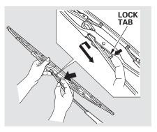
3. Disconnect the blade assembly from the wiper arm by pushing in the lock tab. Hold it in while you push the blade assembly toward the base of the arm.
