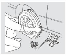
11. Remove the wheel nuts and flat tire. Temporarily place the flat tire on the ground with the outside surface of the wheel facing up. You could scratch the wheel if you put it face down.
