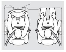
Your car also has side airbags to help protect the upper torso of the driver or a front seat passenger during a moderate to severe side impact.
