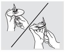
A new CD may be rough on the inner and outer edges. The small plastic pieces causing this roughness can flake off and fall on the recording surface of the disc, causing skipping or other problems. Remove these pieces by rubbing the inner and outer edges with the side of a pencil or pen.
