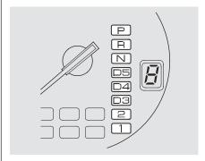
This indicator in the tachometer shows which position the shift lever is in. The illuminated number next to the "D<sub>5</sub>" indicator shows you the gear you have selected in the Sequential SportShift mode.
