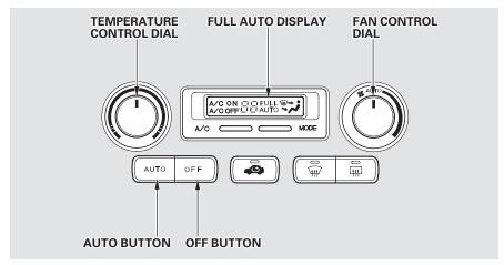
When the temperature is set between the lower and upper limits, the system regulates the interior temperature to the set value. Pressing the OFF button shuts the climate control system completely off. Keep the system completely off only for short periods. To keep stale air and mustiness from collecting, you should have the fan running at all times.
