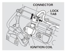
3. Disconnect the wire connector from the ignition coil by pushing on the lock tab and pulling on the connector. Pull on the plastic connector, not the wires.
