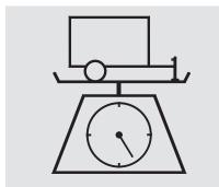
• Total Trailer Weight: The total weight of the trailer and everything loaded in it must not exceed 1,000 lbs (450 kg). Towing a load that is too heavy can seriously affect your car's handling and performance. It can also damage the engine and drivetrain.
