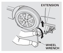
10.Use the extension and wheel wrench as shown to raise the vehicle until the flat tire is off the ground.
