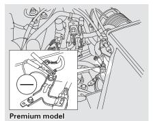
5. Connect the second jumper cable to the negative (—) terminal on the booster battery. Connect the other end to the grounding strap as shown. Do not connect this jumper cable to any other part of the engine.
