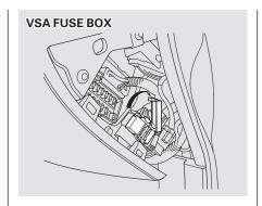
On Type-S The VSA fuse box is located under the interior fuse box on the passenger's side of the dashboard. To open it, push the tab and pull up the left side of the cover as shown.
