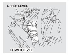
Always use Honda Power Steering Fluid. If it is not available, you may use another power steering fluid as an emergency replacement. However, continued use can cause increased wear and poor steering in cold weather. Have the power steering system flushed and refilled with Honda PSF as soon as possible.
