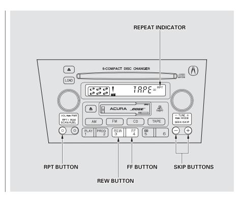
REPEAT — The Repeat function continuously replays the current song or passage. Press the RPT button to activate it; you will see RPT displayed as a reminder. When the system reaches the end of the song or passage currently playing, it will automatically go into rewind. When it senses the beginning of the same song or passage, the system returns to PLAY mode. It will continue to repeat this same program until you deactivate REPEAT by pressing the button again.
