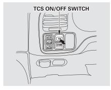
This switch is under the side vent. It lets you turn the Traction Control System on and off. You cannot turn off the TCS while the TCS indicator light is flashing.
