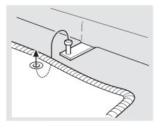
The genuine Acura driver's floor mat that came with your car was designed to be hooked over the floor mat anchor. This keeps the floor mat from sliding forward and possibly interfering with the pedals.
