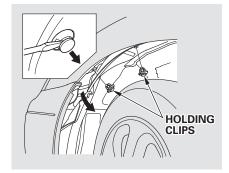
1. If you are changing the bulb on the driver's side, start the engine, turn the steering wheel all the way to the right, and turn off the engine. If you are changing the bulb on the passenger's side, turn the steering wheel to the left.
