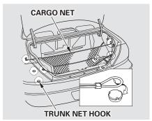
The cargo net can be used to help hold down items stored in the trunk. To use the cargo net, hook it to the buttons on the floor and sides of the trunk. You can use the cargo net in several configurations by hooking it to different buttons.
