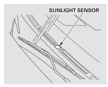
The climate control system has two sensors. A sunlight sensor is located in the top of the dashboard and a temperature sensor is next to the steering column. Do not cover the sensors or spill any liquid on them.
