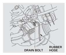
4. Install a rubber hose on the drain bolt at the rear of the engine cylinder block. Loosen the drain bolt.
