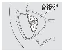
Two controls for the audio system are mounted in the steering wheel hub. These let you control basic functions without removing your hand from the wheel
