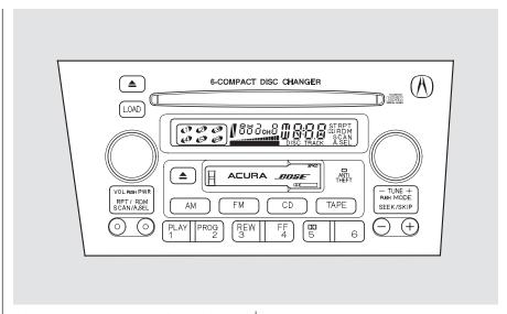
The anti-theft feature will disable the system if it is disconnected from the car's battery. To get the system working again, you must enter a code number (see page 149).
