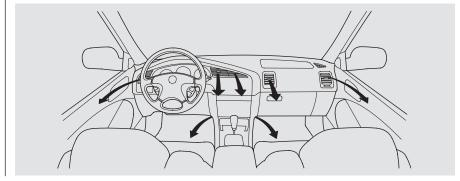
The the button directs the main air flow to the windshield for faster defrosting. It also overrides any MODE selection you may have made.
