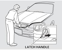
2. Standing in front of the car, reach in between the hood and the front. bumper with your finger. The hood latch handle is under the "A" logo. Slide the latch handle to the right.
