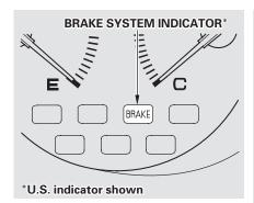
The Brake System Indicator normally comes on when you turn the ignition switch ON (II). It is a reminder to check the parking brake. It comes on and stays lit if you do not fully release the parking brake.
