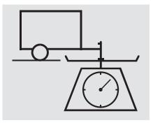
• Tongue Load: The weight that the tongue of a fully-loaded trailer puts on the hitch should be approximately 10 percent of the trailer weight. Too little tongue load can make the trailer unstable and cause it to sway. Too much tongue load reduces front-tire traction and steering control.
