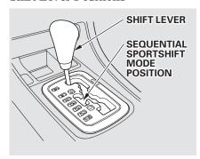
The shift lever has nine positions. It must be in Park or Neutral to start the engine. When you are stopped in D5, D4, D3, 2, 1, N, R, or the Sequential SportShift mode, press firmly on the brake pedal and keep your foot off the accelerator pedal.
