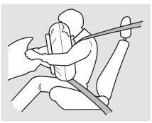
If you ever have a moderate to severe frontal collision, the sensors will detect the vehicle's rapid deceleration. If the rate of deceleration is high enough, the control unit will instantly inflate the front airbags.
