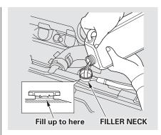
9. Start the engine and let it run for about 30 seconds. Then turn off the engine. Pour coolant into the radiator up to the base of the filler neck.
