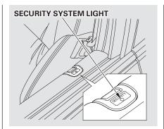
Once the security system is set, opening either door (without using the key or the remote transmitter), or the hood, will cause it to alarm. It also alarms if the radio is removed from the dashboard or the wiring is cut.
