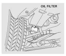
3. Remove the oil filter and let the remaining oil drain. A special wrench (available from your Acura dealer) is required to remove the filter.
