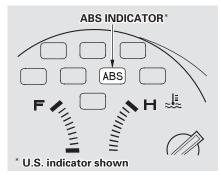
The ABS is self-checking. If anything goes wrong, the ABS indicator on the instrument panel comes on (see page 56). This means the anti-lock function of the braking system has shut down. The brakes still work like a conventional system without anti-lock, providing normal stopping ability. You should have the dealer inspect your car as soon as possible.
