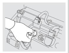
6. Put the new spark plug into the socket; then screw it into the hole. Screw it in by hand so you do not crossthread it.
