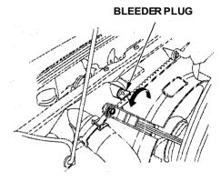
5. Loosen the bleeder plug on top of the radiator.
