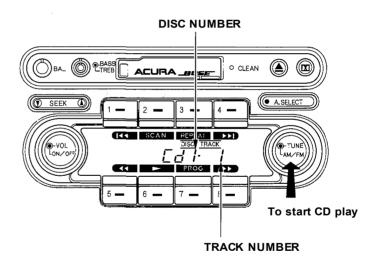
When that disc ends, the next disc in the magazine is loaded and played. When disc 6 has completed, the system will return to disc 1. To select another disc, press PROG. The next CD in the changer is loaded and starts to play from the first track. The new CD and track numbers are displayed.
