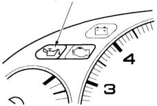
This indicator should light when the ignition switch is ON (II), and go out after the engine starts. It should never come on when the engine is running. If it starts flashing, it indicates that the oil pressure dropped very low for a moment, then recovered. If the indicator stavs on with the engine running, it shows that the engine has lost oil pressure and serious engine damage is possible. In either case, you should take immediate action.
