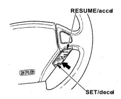
Press and release the SET/decel button on the steering wheel. The CRUISE CONTROL light on the instrument panel comes on to show the system is now activated.
