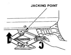
8. Locate the jacking point nearest the tire you need to change. It is pointed to by an arrow molded into the underside of the body. Place the jack under the jacking point. Turn the end bracket clockwise until the top of the jack contacts the jacking point. Make sure the jacking point tab is resting in the jack notch.
