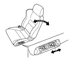
Adjust the seat-back angle by pushing the rear switch in the direction you want to move.
