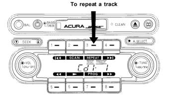
To search for a particular program on a disc, press SCAN. The system will skip forward to the next track and begin to play it. If you do not touch any of the controls, the system skips to the beginning of the next track after ten seconds and begins to play that. When the system gets to a track you want to hear all the way through, press SCAN again. You can only scan tracks on the disc currently being played.
