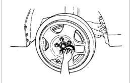
12. Put on the folding spare tire with the air valve toward the bottom. Put the wheel nuts back on fingertight, then tighten them in a crisscross pattern with the wheel wrench until the wheel is firmly against the hub. Do not try to tighten them fully. Inflate the folding spare tire only when it is on the car. Inflating it while it is lying on the ground may trap stones or other foreign matter between the tire and the wheel rim.
