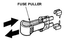
4. Check the smaller fuses by pulling out the fuse with the fuse puller provided in the interior fuse box.
