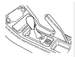
The manual transmission is synchronized in all forward gears for smooth operation. It has a lockout so you cannot shift directly from Fifth to Reverse instead of sixth (see page 150). When shifting up or down, make sure you push the clutch pedal down all the way, shift to the next gear, and let the pedal up gradually. When you are not shifting, do not rest your foot on the clutch pedal. This can cause your clutch to wear out faster.
