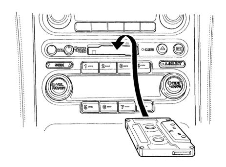
Dolby B noise reduction turns on when you insert a cassette. If the tape was not recorded with Dolby B noise reduction, turn it off by pressing the DD button.
