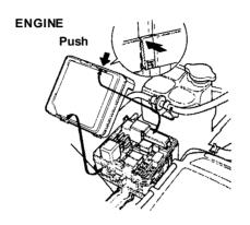
The engine compartment fuse box is located next to the air cleaner housing. To open, push the tab as shown.
