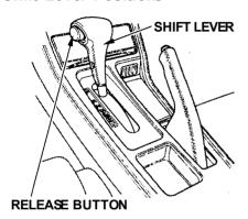
The console shift lever has seven positions. It must be in Park or Neutral to start the engine.
