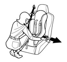
With the child seat in position, route the belt through the child seat according to the seat maker's instructions, then insert the latch plate into the buckle.
