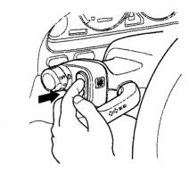
The rear window defogger will clear fog, frost, and thin ice from the window. Push the defogger button to turn it on and off. The light on the front of the pod lights to show the defogger is on. If you do not turn it off, the defogger will shut itself off after about 25 minutes. It also shuts off when you turn off the ignition. You have to turn it on again when you restart the car.
