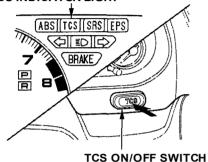
This switch is on the dashboard behind the right control pod. It lets you turn the Traction Control System on and off. You cannot turn off the TCS while the TCS indicator light is flashing.
