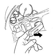
To change between low beams and high beams, pull the turn signal lever as far as it will move towards you, then let go. The blue high beam indicator will light (see page 52).
