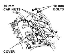
Replace the spark plugs one side at a time. Make sure the front cylinder ignition coils and the back side of the cover are marked "FR" and the rear cylinder ignition coils and the back side of the cover are marked "RR". To replace them:
