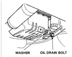
2. Remove the engine oil fill cap. Remove the oil drain bolt from the bottom of the engine. Drain the oil into an appropriate container.
