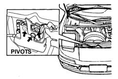
Clean the hood latch assembly with a mild cleaner, then lubricate it with a multipurpose grease. Lubricate all the moving parts, including the pivot. Follow the time and distance recommendations in the Maintenance Schedule. If you are not sure how to clean and grease the latch, contact your Acura dealer.
