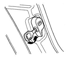
To prevent anyone from getting to the roof panel and the engine when you park the car with the roof removed, lock the rear window release lever with the master key.
