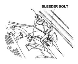
11. Loosen the bleeder bolt near the expansion tank.
