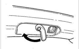
Secure the roof by turning each release lever until the lock tab clicks forward. Pull on the levers to make sure they are locked. If the release levers are locked correctly, the roof unlatched indicator will not light when you turn the ignition ON (II). 10.Close the roof cover and snap the hook onto the window frame. Close the rear window.
