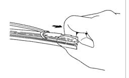
3. Remove the blade from its holder by grasping the tabbed end of the blade. Pull firmly until the tabs come out of the holder.
