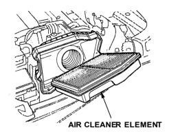
4. Remove the old air cleaner element. Carefully clean the inside of the air cleaner housing with a damp
