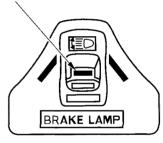
This indicator lights when the roof is installed if either release lever is not fully locked. Check both release levers to make sure they are locked. This indicator also lights when the roof is removed but is not properly stored in the holder.
