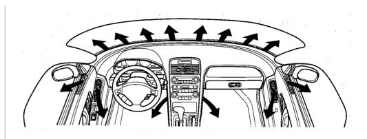
The the button directs the main air flow to the windshield for faster defrosting. It also overrides any MODE selection you may have made. To defrost more quickly, turn the temperature control to 82°F~86°F (28°C~30°C).
