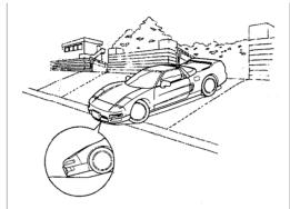
Curbs and steep inclines could damage the front and rear bumpers. Low curbs that do not affect the average car may be high enough to hit the bumper on your Acura. The front or rear bumper may scrape when trying to drive onto an incline, such as a steep driveway or trailer ramps.
