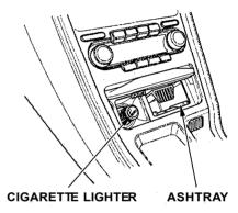
The ignition switch must be in ACCESSORY (I) or ON (II) for the cigarette lighter to work. To heat up the lighter, push it in. It will pop out when it is ready for use. Do not hold the lighter in while it is heating up, you could cause it to overheat.
