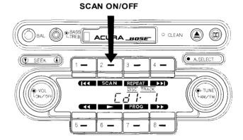
You can get the CD changer to randomly select tracks by pressing A. SELECT. The indicator in the button lights as a reminder. With this active, the system selects and plays tracks randomly rather than sequentially. Random selection only works on the disc currently playing, not across all six discs. Cancel random selection by pressing A. SELECT again. Random selection is also cancelled by selecting the SCAN function.
