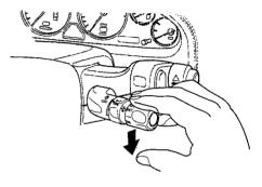
To operate the wipers in mist mode, push the control lever down. The wipers run at high speed until you release the lever. This gives you a quick way to clear the windshield.
