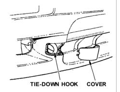
For very short distances such as freeing the car, you can use the tiedown hook on the lower right of the front bumper. Remove the cover to expose the hook. This hook is not for open-road towing (see Emergency Towing, page 269).
