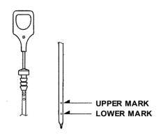
Remove the dipstick again and check the level. It should be between the upper and lower marks.
