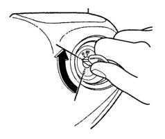
14.Reach into the car and turn the ignition switch to ACCESSORY (I). This will start the air pump to inflate the tire
