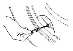
17. Screw the valve cap on the valve tightly with your hands.
