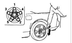
19. Tighten the wheel nuts securely in the same crisscross pattern. Have the wheel nut torque checked at the nearest automotive service facility.
