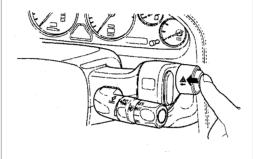
Push the large red button on the right pod to turn on the hazard warning lights (four-way flashers). This causes all four outside turn signals and both indicators in the instrument panel to flash. Use the hazard warning lights if you need to park in a dangerous area near heavy traffic, or if your car is disabled.
