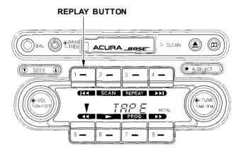
The SKIP function ▶▶I allows you to skip over a song or other passage. When you press this button, the system goes into fast forward until it senses a silent period on the tape. The light in the SKIP button flashes during fast forward. When the system finds a silent period, it goes back to PLAY.
