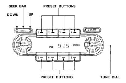
The A. SELECT function allows you to find stations easily when you are in an unfamiliar area. Press the A. SELECT button. The system automatically scans both the AM and FM bands, memorizes the eight strongest on each band, and stores them in the eight preset buttons. You can then use the buttons to tune to those stations. The light in the A. SELECT button stays on as a reminder.
