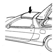
Set the roof in place on the car. Make sure all four corners are sitting flush with the car body.
