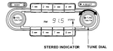
The easiest way to find your favorite stations is to set their frequencies into the eight preset buttons. To do this, tune to the desired station as described previously. Press one of the preset buttons (1 — 8) and hold it until you hear a beep. You can preset eight stations on each band.
