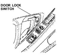
Each door has a door lock switch. Either switch locks and unlocks both doors. Push LOCK to lock both doors, and the top portion of the switch to unlock them.
