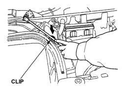
5. Snap the support rod back into its holding clip.
