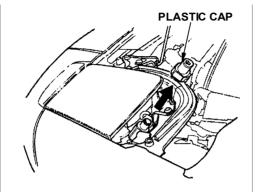
3. Remove the plastic cap on top of the headlight motor.
