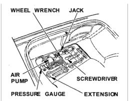
4. Open the trunk (see page 70). Lift the cover; remove the jack, wheel wrench, extension, air pump, pressure gauge, and screwdriver from the trunk. The tools may become very hot while the car is being driven. Wear gloves or use a protective cloth when handling the tools.
