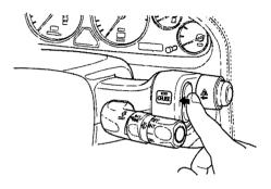
The cruise control master switch is on the right pod. For information on using the cruise control, see page 62
