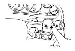
(40 km/h), then press the RESUME/accel button. The CRUISE CONTROL light comes on, and the car will accelerate to the same cruising speed as before.
