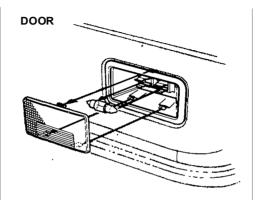
1. Remove the lens by carefully prying on the edge with your fingernail or a small flat-tip screwdriver. The two lenses on the roof-mounted interior light come out as a unit.
