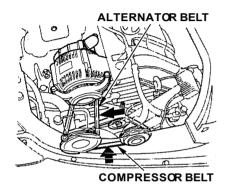
You should check the condition of the two engine belts every 2 years. Examine the edges of each belt for cracks or fraying. Check the tension of each belt by pushing on it at the point shown in the diagram. The belts should have the following "play" or deflection.
