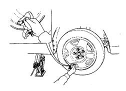
15. After about five minutes, unscrew the air pump hose and check the pressure with the supplied pressure gauge. Inflate to:
