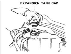
13. Fill the expansion tank to about 1 in. (2.5 cm) above the MAX line. Put the cap back on the tank, only tighten it to the first stop. Start the engine and let it run until it warms up (the radiator cooling fan comes on at least twice).
