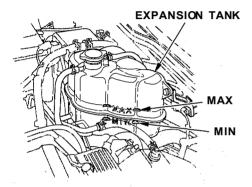
Look at the coolant level in the expansion tank. Make sure it is between the MAX and MIN lines. If it is below the MIN line, see Adding Engine Coolant on page 185 for information on adding the proper coolant.
