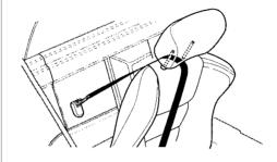
Pass the strap between the top of the seat and the bottom of the head restraint.
