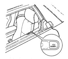
The security system helps to protect your car and valuables from theft. The horn sounds, the headlights pop up, and all the exterior lights flash if someone attempts to break into your car or remove the radio. The system alarms continue for two minutes unless you turn it off manually. To turn the system off, unlock either door with the key.
