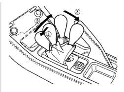
1. With the clutch pedal depressed, move the shift lever to the First/ Second gear side of the Neutral gate, then shift to Reverse.
