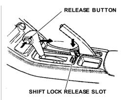
6. Remove the key from the Shift Lock Release slot. Depress the brake pedal and restart the engine.
