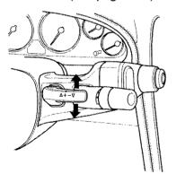
If you move the console shift lever from "D" to "3/M" while the car is moving, the transmission remains in the gear it was in. If you do this while stopped, the transmission selects first gear.
