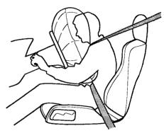
If you ever have a moderate to severe frontal collision, the sensors will detect rapid deceleration and signal the control unit to instantly inflate the airbags and activate the automatic seat belt tensioners.
