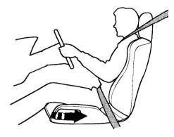
Any driver who sits too close to the steering wheel is at risk of being seriously injured or killed by striking the steering wheel, or from being struck by an inflating airbag during a crash.
