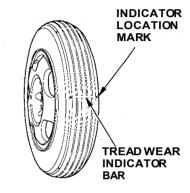
The folding spare tire has a shorter tread life than a regular tire. Replace it when you can see the tread wear indicator bars. The spare tire is not designed to be mounted on a regular wheel, and the compact wheel is not designed for mounting a regular tire.
