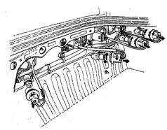
The bulbs for the taillights, tail/stoplights, rear turn signals, and back-up lights are behind the trunk liner.
