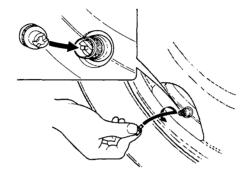
3. Remove the rubber cover on top of the valve cap. Use the notch on the valve cap to unscrew the spare tire valve core until the air starts coming out. Use your hand to shield your eyes. The valve core can fly out under pressure.
