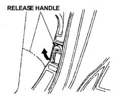
1. Shift to Park or Neutral and set the parking brake. Locate the release handle on the rear of the driver's door opening, next to the seat. Pivot this handle towards the driver's seat. The rear window will pop up slightly.
