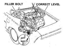
Check the fluid level with the transmission at normal operating temperature and the car sitting on level ground. Remove the transmission filler bolt and carefully feel inside the bolt hole with your finger. The fluid level should be up to the edge of the bolt hole. If it is not, add Honda Manual Transmission Fluid (MTF) until it starts to run out of the hole. Reinstall the filler bolt and tighten it securely.
