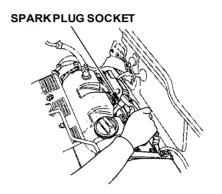
4. Remove the spark plug with a five-eighths inch (16 mm) spark plug socket.
