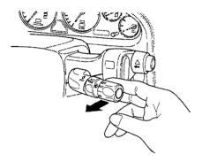
To clean the windshield, pull back on the wiper control lever. The washers spray until you release the lever. The wipers run at low speed while you're pulling the lever, then complete one more sweep of the windshield after you release it.
