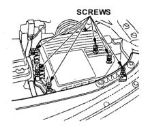
Loosen the six Phillips-head screws around the edge of the air cleaner housing cover. Remove the air cleaner housing cover and set it aside.
