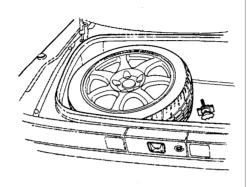
21. Temporarily keep the wing bolt in the trunk as well. See Replacing Tires and Wheels on page 213 for tire replacement.
