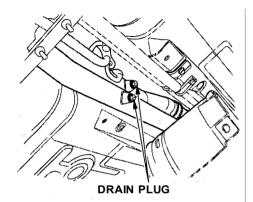
6. Remove the drain plugs from the coolant pipes under the car.
