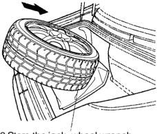
20. Store the jack, wheel wrench, extension, air pump, pressure gauge, screwdriver, and flat tire in the trunk.
