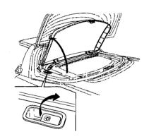
6. Pull up the roof cover release lever and raise the roof cover.
