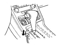
16. When finished, reach in and turn the ignition switch to LOCK (0). Unplug the air pump power cord.
