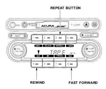
similar to REPEAT. When you press this button, the system immediately goes into rewind. The light in the REPLAY button flashes during rewind When it senses a silent period on the tape, the system stops rewinding and goes back to PLAY. Unlike REPEAT, this function replays a selection only once. If you will play straight through.
