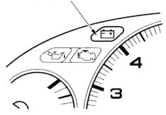
This indicator should come on when the ignition switch is ON (II), and go out after the engine starts. If it comes on brightly when the engine is running, it indicates that the charging system has stopped charging the battery.
