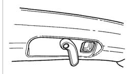
Make sure the roof panel release levers are in the unlocked (down) position.
