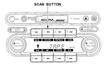
The REPLAY, SKIP and SCAN functions use silent periods on the tape to find the end of a selection. These features may not work satisfactorily on tapes that have almost no gap between songs, a high noise level between songs, or silent periods in the middle of songs.
