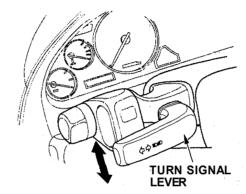
Signal a turn or lane change with this lever. Push down on the lever to signal a left turn, and up to signal a right turn. If you push it up or down all the way, the turn signal continues to blink even when you release the lever. It shuts off automatically as you complete the turn.
