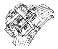
Check the battery condition by looking at the test indicator window oil the battery.
