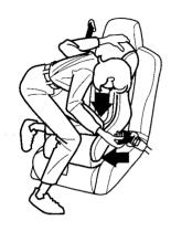
5. After confirming that the belt is locked, grab the shoulder part of the belt near the buckle and pull up to remove any slack from the lap part of the belt. Remember, if the lap part of the belt is not tight, the child seat will not be secure. It may help to put weight on the child seat, or push on the back of the seat, while pulling up on the belt.
