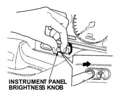
The knob on the dashboard behind the left pod controls the brightness of the instrument panel lights. Push the knob to get it to pop out. Turn the knob to adjust the brightness, then push it back in so you cannot accidentally bump it.
