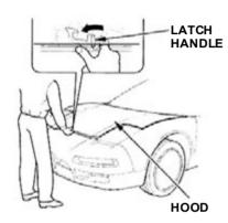
2. Standing in front of the car, put your fingers under the front edge of the hood to the right of center. Slide your hand to the left until you feel the hood latch handle. Push this handle to the left until it releases the hood. Lift the hood.
