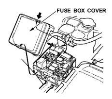
3. Open the rear window and engine cover. Locate the engine compartment fuse box on the driver's side of the compartment. Remove the fuse box cover.
