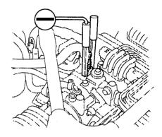
5. Connect the second jumper cable to the negative ( — ) terminal on the booster battery. Connect the other end to the boss on the intake manifold as shown. Do not connect this jumper cable to any other part of the engine.
