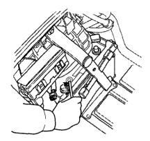
If the terminals are severely corroded, clean them with baking soda and water. Then use a wrench to loosen and remove the cables from the terminals. Always disconnect the negative ( — ) cable first and reconnect it last. Clean the battery terminals with a terminal cleaning tool or wire brush. Reconnect and tighten the cables, then coat the terminals with grease.
