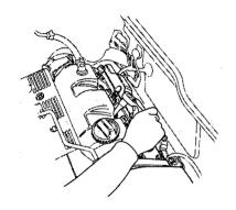
Torque the spark plug. (If you do not have a torque wrench, tighten the spark plug two-thirds of a turn after it contacts the cylinder head.) Tightening torque: 13 lbf.ft (18 N.m,1.8 kgf.m)
