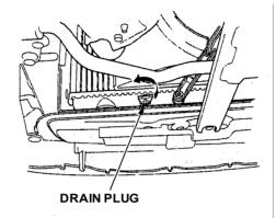
4. Remove the drain plug from the bottom of the radiator.
