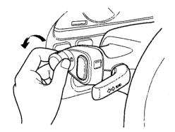
The rotating switch on the left pod controls the lights. Turning this switch to "•" turns on the parking lights, taillights, instrument panel lights, side-marker lights, and rear license plate lights. Turning the switch to "•" raises the headlights and turns them on.
