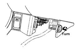
The interior fuse box is underneath the dashboard on the driver's side. To open it, turn the knob as shown.
