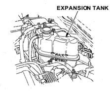
If the expansion tank is completely empty, add coolant to bring it up to the MAX line. Inspect the cooling system for leaks. This coolant should always be a mixture of 50 percent antifreeze and 50 percent water. Never add straight antifreeze or plain water.
