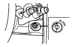
The ignition switch is on the right side of the steering column. It has four positions:
