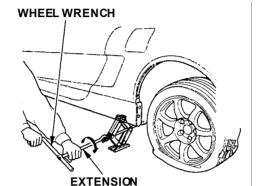
9. Use the extension and wheel wrench as shown to raise the car until the flat tire is off the ground.
