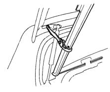
8. Put the hook around the edge of the roof cover to hold it up.
