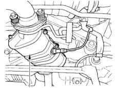
THREE WAY CATALYTIC CONVERTER
