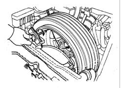
7. Store the folding spare tire in the front compartment with the outside surface of the wheel contacting the bracket of the spare tire well. Securely tighten the wing bolt.
