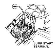
4. Connect one jumper cable to the JUMP START terminal in the fuse box. Connect the other end to the positive (+) terminal on the booster battery.
