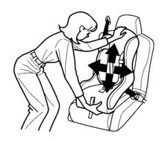
Push and pull the child seat forward and from side to side to verify that it is secure enough to stay upright during normal driving maneuvers. If the child seat is not secure, unlatch the belt, allow it to retract fully, then repeat these steps.
