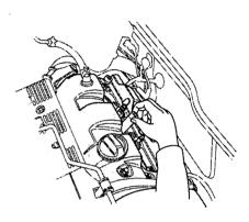
5. Put the new spark plug into the socket; then screw it into the hole. Screw it in by hand so you do not crossthread it.
