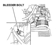
10.Loosen the bleeder bolt on top of the engine.
