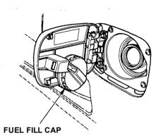
3. Remove the fuel fill cap slowly. You may hear a hissing sound as pressure inside the tank escapes. Place the cap in the holder on the fuel fill door.
