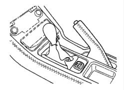
To apply the parking brake, pull the lever up fully. To release it, pull up slightly, push the button, and lower the lever. The parking brake light on the instrument panel should go out when the parking brake is fully released (see page 49). If you try to drive the vehicle without releasing the parking brake, the ABS indicator may come on, and the ABS may not work properly.
