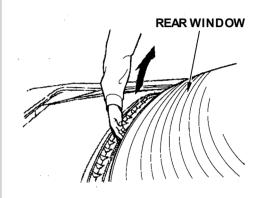
2. Stand just behind the driver's door. Reach under the rear edge of the rear window at its center and raise it. It will stay up by itself.
