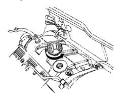
To add oil, unscrew and remove the engine oil fill cap on top of the left valve cover. Pour in the oil, and replace the engine oil fill cap. Tighten it securely. Wait a few minutes and recheck the oil level. Do not fill above the upper mark; you could damage the engine.
