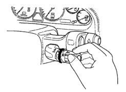
The lever on the right pod controls the windshield wipers and washers. The rotary switch at the end of the lever has three positions:
