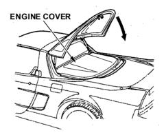
To Close the Rear Window: Snap the support rod back into the clip and lower the engine cover or roof holder. Pull the rear window down until it is resting on the body, then push on the center of the back edge until it latches. Make sure it is securely closed before driving away.
