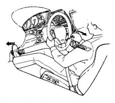
Park (P) — This position mechanically locks the transmission. Use Park whenever you are turning off or starting the engine. To shift out of Park, you must press on the brake pedal and have your foot off the accelerator pedal. Press the release button on the side of the shift lever to move it.
