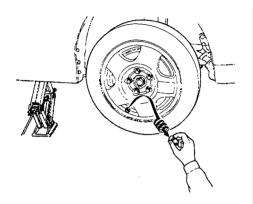
2. Unscrew and remove the folding spare tire valve cap.
