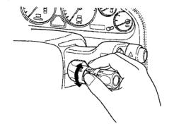
In intermittent, the wipers operate every few seconds. You can vary how often the wipers sweep the windshield by turning the INT TIME ring next to the rotary switch. In low speed and high speed, the wipers run continuously.
