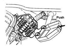
The under-hood fuse box is located in the front of the engine compartment on the passenger's side. To open it, push the tab as shown.
