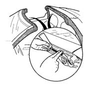
Dust is the main cause of creaks or other sounds coming from the roof. Regularly clean the roof panel and body seals with glass cleaner and a soft cloth.
