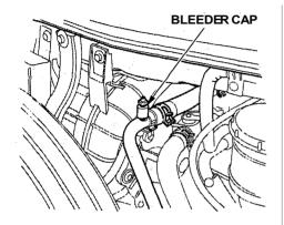
9. Remove the bleeder cap from the top of the heater inlet.
