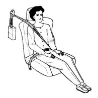
Your Acura has automatic seat belt tensioners for added protection during a moderate to severe frontal collision.
