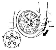
6. Remove the folding spare tire and install the original tire and wheel nuts. Lower the car and tighten the wheel nuts securely in a crisscross pattern. Tighten to: 80 lbf.ft (108N.m, 11 kgf.m)
