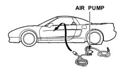
5. Place the air pump near the flat tire. Open the nearest window, and route the air pump's power cord through the open window.
