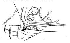
To raise and lower the headlight doors without turning on the headlights, push the dashboard button behind the left pod.
