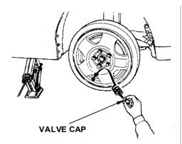
5. Put the rubber cap back on the valve cap. Screw the valve cap back on the folding spare tire valve.
