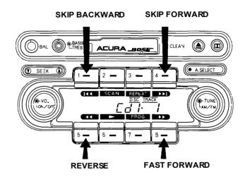
To replay the current track, press REPEAT. The indicator in the preset button will come on as a reminder. At the end of the track, the system skips back to its beginning. That track will repeat continuously until you cancel REPEAT by pressing the button again.
