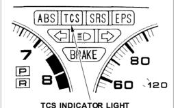
When driving on a loose or slippery road surface, you may notice that the engine does not respond to the accelerator in the same way it does at other times. This is a sign the TCS is activating. You will see the TCS indicator light flash.
