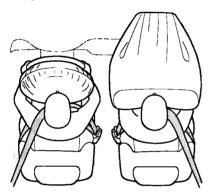
Your car has a Supplemental Restraint System (SRS) with frontal airbags to help protect the driver and a passenger.
