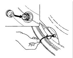
4. As the tire deflates, it will fold back to its original shape. When the air stops coming out of the tire, use the notch on the valve cap to tighten the valve core.
