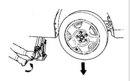
18.Lower the car to the ground and remove the jack.
