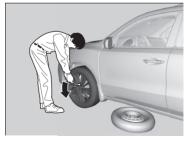
**10.** Loosen each wheel nut about one turn using the wheel nut wrench.
