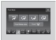
Select a desired vent mode icon, or **Front Mode Auto**: The system automatically selects
