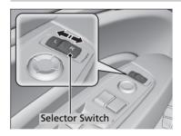
If activated, either side door mirror automatically tilts downward when you put the transmission into  $\boxed{\mathbf{R}}$ ; this improves close-in visibility on the selected side of the vehicle when backing up. The mirror automatically returns to its original position when you take the transmission out of  $\boxed{\mathbf{R}}$ .
