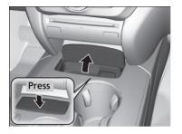
Press the raised detent to open the lid. To close the lid, push it down until it latches.
