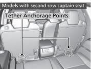
A tether anchorage point is provided behind each second and third row seating position. If you have a child seat that comes with a tether but can be installed with a seat belt, the tether may be used for additional security.
