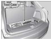
**3.** Take the jack, wheel nut wrench, and jack handle bar out of the tool case.
