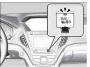
The rear defogger and heated door mirrors automatically switch off after 10-30 minutes depending on the outside temperature.
