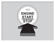
**3.** Press the **ENGINE START/STOP** button without depressing the accelerator pedal. The engine will crank until it starts.
