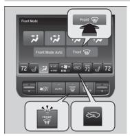
Pressing the button or selecting the **Front** con appearing after the vent mode icon is selected turns the air conditioning system on and automatically switches the system to fresh air mode.
