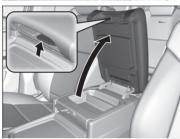
Pull the driver's side handle to open the utility tray in the console lid.
