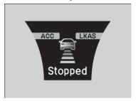
Your vehicle also stops, automatically. The **Stopped** message appears on the MID. When the vehicle ahead of you starts again, the vehicle icon on the MID blinks. If you press the **RES/+/SET/-** switch up or down, or depress the accelerator pedal, ACC with Low Speed Follow operates again within the prior set speed.
