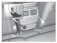
Open the outlet cover and insert the cable.
