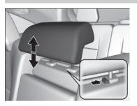
A passenger sitting in the second row center seating position should adjust the height of their head restraint to an appropriate position before the vehicle begins moving.
