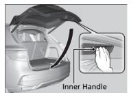
When all the doors are unlocked, the tailgate is unlocked.
