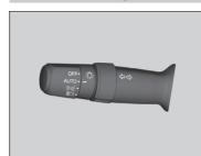
Automatic lighting control can be used when the power mode is in ON.
