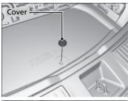
**4.** Remove the cover on the cargo area lining to access the shaft for the spare tire hoist.
