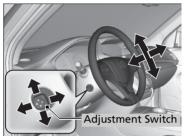
Push and hold the adjustment switch to move the steering wheel in, out, up or down.
