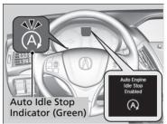
The engine then restarts once the vehicle is about to move again, or depending on environmental and vehicle conditions, and the indicator (green) goes off.
