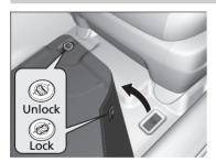
The front and second row passenger's floor mats hook over floor anchors, which keep them from sliding forward. To remove a mat for cleaning, turn the anchor knobs to the unlock position. When reinstalling the mat after cleaning, turn the knobs to the lock position.
