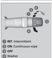
The rear wiper and washer can be used when the power mode is in ON.
