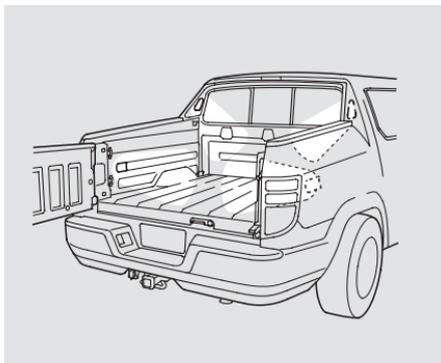
Your vehicle has bed lights in the pickup bed: a light on each front upper and rear bottom side. With the shift lever in the Park position, the bed lights come on when you push the bed light switch on the dashboard, swing open the tailgate, or open the In-Bed Trunk. The indicator on the instrument panel also comes on to remind you that the bed lights are on.
