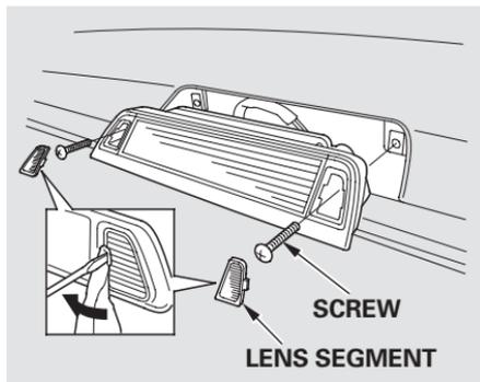
1. Place a cloth on the edge of the lens segment to prevent scratches. Remove each lens segment by carefully prying on its edge with a small flat-tip screwdriver.
