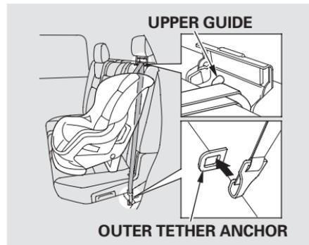
1. After properly securing the child seat (see page 46), lift the head restraint, then route the tether strap over the seat-back and through the head restraint legs.
