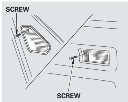
1. Remove the mounting screw from the bed light assembly.
