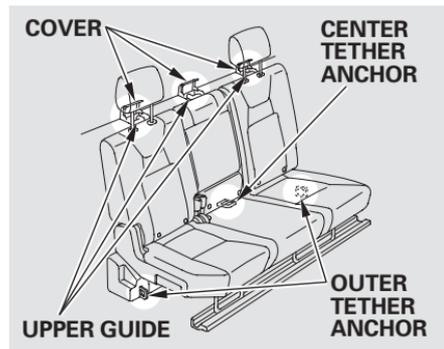
A child seat with a tether can be installed in any seating position in the back seat.
