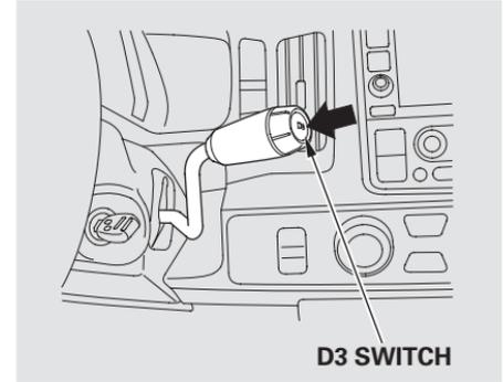
Press the D3 switch on the end of the shift lever to turn this mode on or off; the D3 indicator comes on whenever D3 is selected.
