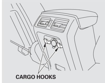
There are two cargo hooks for plastic grocery bags at the back of the center console. They are designed to hold light items. Heavy objects may damage the hooks.
