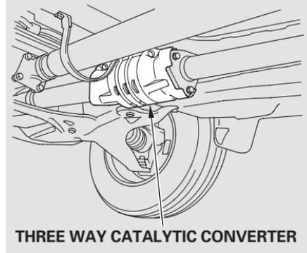
The defective three way catalytic converters contribute to air pollution, and can impair your engine's performance. Follow these guidelines to protect your vehicle's three way catalytic converters.
