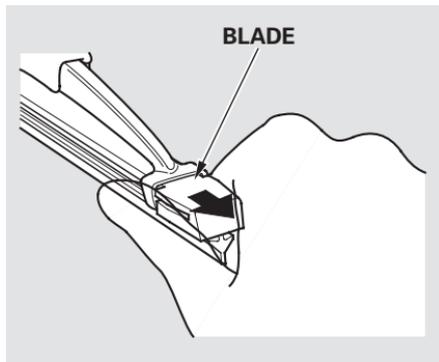
4. Remove the blade from its holder by grabbing the tabbed end of the blade. Pull up firmly until the tabs come out of the holder.
