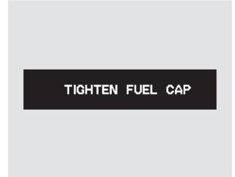
Your vehicle’s on board diagnostic system will detect a loose or missing fuel fill cap as an evaporative system leak. The first time a leak is detected a “TIGHTEN FUEL CAP” message appears on the multi-information display.
