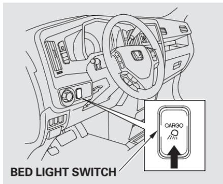
To turn off the lights, push the light switch again, or close the tailgate and the In-Bed Trunk.
