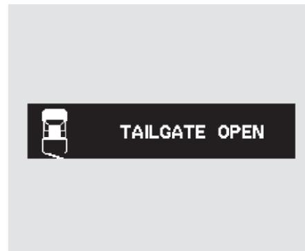
When the tailgate is not tightly closed, the “TAILGATE OPEN” message will come on.
