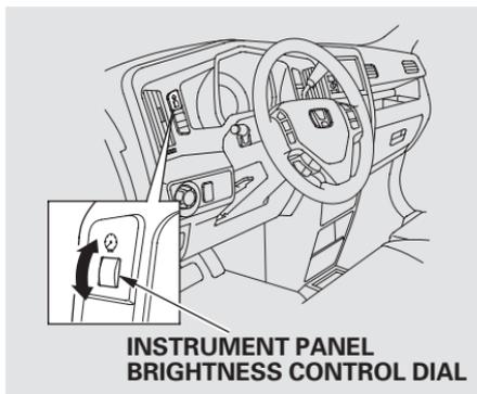
The dial on the instrument panel controls the brightness of the instrument panel lights and the console compartment light. Turn the dial to adjust the brightness.
