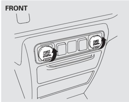
There are three accessory power sockets in your vehicle. Two accessory power sockets are above the center pocket on the dashboard, and another is on the back of the center console.
