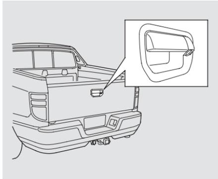
For the best picture, always keep the rearview camera clean, and do not cover the camera lens. To avoid scratching the lens when you clean it, use a moist, soft cloth.
