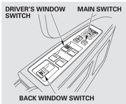
Turn the ignition switch to the ON (II) position to raise or lower any side window, or open and close the back window. To open the window, push the switch down and hold it. Release the switch when you want the window to stop. Pull back on the switch and hold it to close the window.
