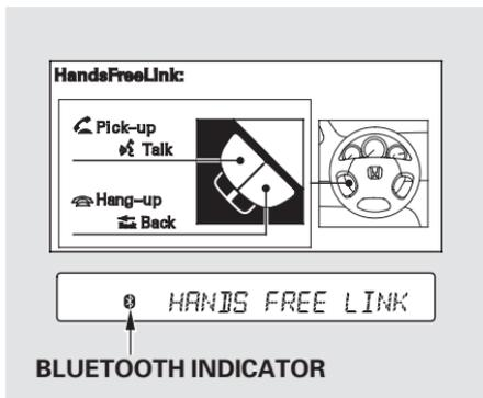
A notification that there is an incoming call, or HFL is in use, will appear on the navigation screen when the audio system is on.
