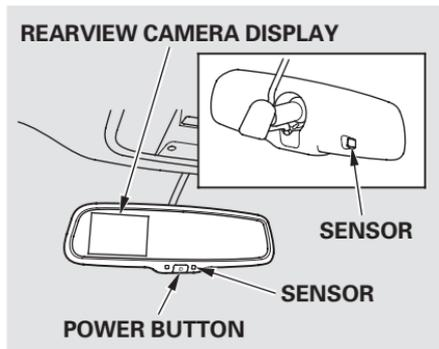
Whenever you shift to reverse (R) with the ignition switch in the ON (II) position, the rear view appears on a display in the rearview mirror.
