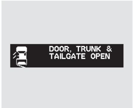
When the In-Bed Trunk, tailgate, and one or more doors are not tightly closed, the “DOOR, TRUNK & TAILGATE OPEN” message will come on.
