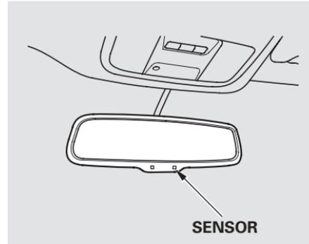
When driving after dark, the automatic dimming rearview mirror always reduces the glare from headlights behind you, based in inputs from the mirror sensor. This feature is always active.
