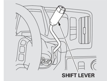
To shift from Park to any position, press firmly on the brake pedal, and pull the shift lever toward you. You cannot shift out of Park when the ignition switch is in the LOCK (0) or ACCESSORY (I) position.
