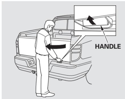
To swing open the tailgate, first make sure it is fully closed, then pull up the right lower handle, and swing the tailgate to the left.
