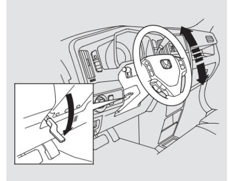
3. Push the lever up to lock the steering wheel in position.
