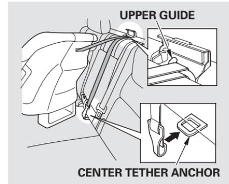
3. Route the tether strap over the seat-back, lift the cover, then hook the tether strap through the upper guide as shown.
