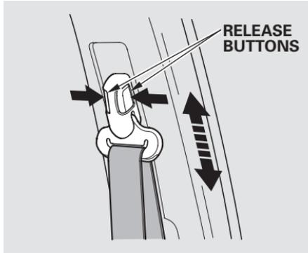
The front seats have adjustable seat belt anchors. To adjust the height of an anchor, squeeze the two release buttons, and slide the anchor up or down as needed (it has four positions).
