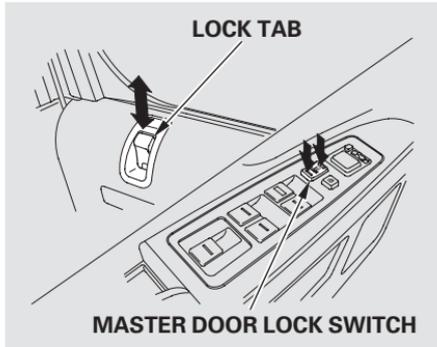
To lock all doors and the In-Bed Trunk, push the front of the master door lock switch on either front door, press the lock tab down on the driver's door, or use the key on the outside lock on the driver's door.
