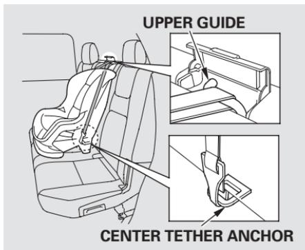
5. Attach the tether strap hook to the center tether anchor between the lower anchors for the LATCH-compatible child seat.
