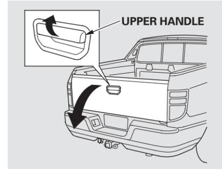
To drop open the tailgate, pull up the upper handle, then pull down the tailgate. To close the tailgate, push firmly up until it latches.
