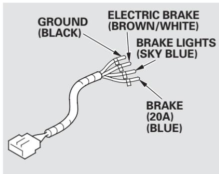
The trailer jumper harness is used to install the controller for the electric trailer brakes. For more information, see **Trailer Brakes** on page 296 .
