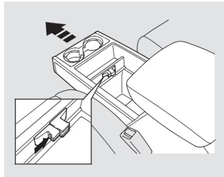
To open the front of the compartment, squeeze the knob, and push it forward while sliding the beverage holder. To close, squeeze the knob and pull the compartment backward until the beverage holder latches.
