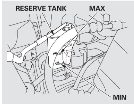
Look at the coolant level in the radiator reserve tank. Make sure it is between the MAX and MIN lines. If it is below the MIN line, see **Adding Engine Coolant** on page 327 for information on adding the proper coolant.
