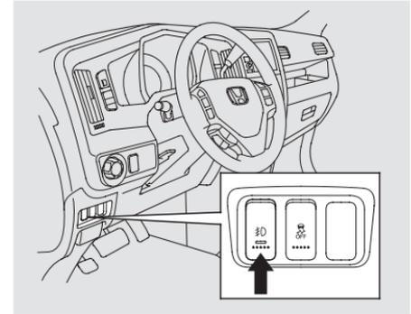
Turn the fog lights on and off by pressing the button. The indicator in the button lights to show the fog lights are on.
