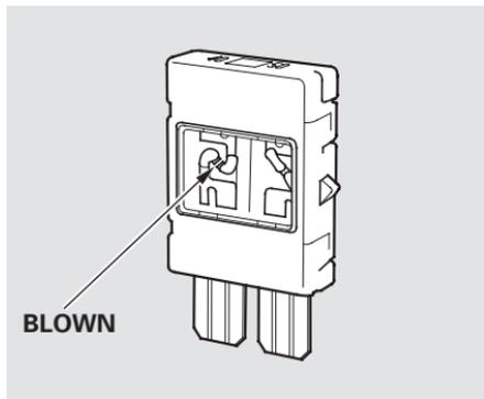
3. Check each of the large fuses in the primary under-hood fuse box by looking through the side window at the wire inside. Removing these fuses requires a Phillips-head screwdriver.
