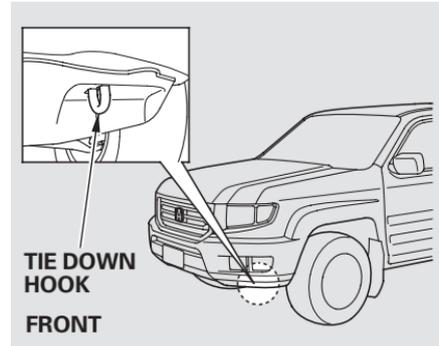
For very short distances, such as freeing the vehicle, you can use the tie down hooks on the lower of the front and rear bumpers.
