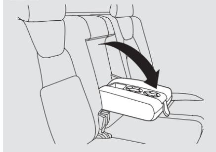
The rear seat armrest is in the center of the rear seats. Pivot it down to use it.
