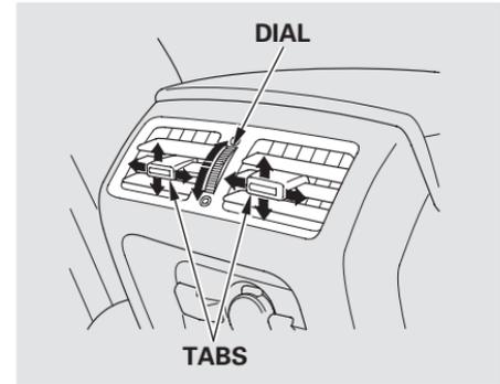
You can adjust the direction of the air coming from the rear vents in the back of the center console by moving the tab in the center of each vent up-and-down and side-to-side.
