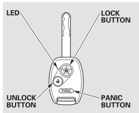
**LOCK** – Press this button once to lock all doors and the In-Bed Trunk. Some exterior and interior lights will flash once.
