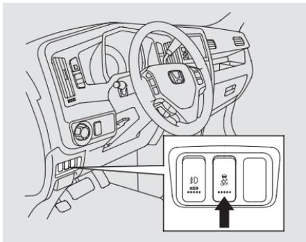
This switch is above the parking brake release handle. To turn the VSA system on and off, press and hold it until you hear a beep.
