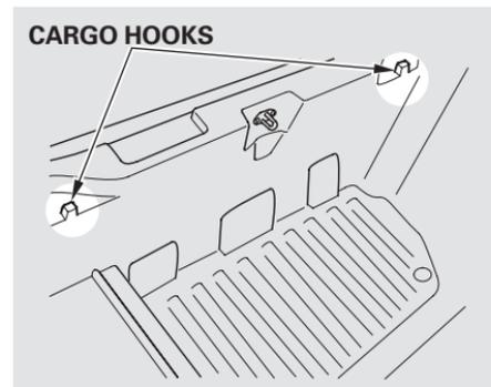
There are two cargo hooks for plastic grocery bags at the back of the In-Bed Trunk. They are designed to hold light items. Heavy objects may damage the hooks.
