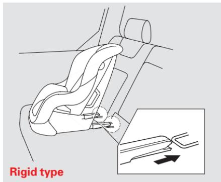
4. Place the child seat on the vehicle seat, then attach the seat to the lower anchors according to the child seat maker's instructions.
