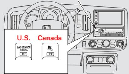
This indicator alerts you that the passenger’s front airbag has been shut off because weight sensors detect about 65 lbs (29 kg) or less (the weight of an infant or small child) on the front passenger’s seat. It does **not mean** there is a problem with the airbag.
