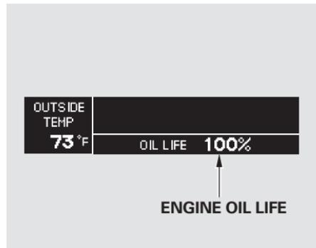
This shows the remaining life of the engine oil. It shows 100% after the engine oil is replaced and the display is reset. The engine oil life is calculated based on engine operating conditions and accumulated engine revolutions. For more information, see page [311](#).
