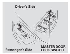
Each front door has a master door lock switch. Either switch locks and unlocks all doors and the tailgate. Push the top of the switch to lock all doors and the tailgate; push the bottom to unlock them.
