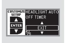
To exit HEADLIGHT AUTO OFF TIMER without changing the current setting, select EXIT by pressing the INFO (▲/▼) button, then press the SEL/RESET button. The screen goes back to CUSTOMIZE MENU.
