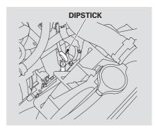
2. Remove the dipstick (yellow loop) from the transmission, and wipe it with a clean cloth.
