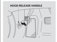
1. Park the vehicle, and set the parking brake. Pull the hood release handle located under the lower left corner of the dashboard. The hood will pop up slightly.
