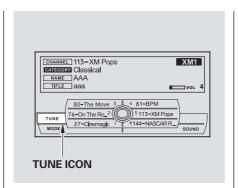
You can also change channel selections on the audio control display. Press the AUDIO button to view the display, then push down the selector on the interface dial. Rotate the interface dial to select the tune. Press ENTER on the selector to enter your selection. Rotate the interface knob to the desired channel. In the category mode, you can only select channels within that category.
