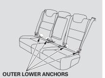
To install a LATCH-compatible child seat in either of the rear outer seats:
