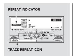
REPEAT — This feature, when activated, continuously replays the current track (file in MP3/WMA mode). To activate it, press the AUDIO button to view the display, then push down the selector on the interface dial. Rotate the interface dial to select track repeat. Press ENTER on the selector to enter your selection.
