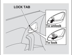
Each door has a lock tab next to the inside door handle. When you pull backward on the lock tab on the driver's door, all the doors and the tailgate lock. Pushing forward on the lock tab on the driver's door unlocks only that door. The lock tab on the each passenger's door locks and unlocks only that door.
