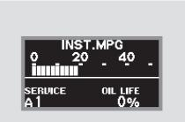
Press the SEL/RESET button on the steering wheel repeatedly to select the engine oil life. The message "SERVICE", along with "0 %", and the maintenance item code are displayed on the lower part of the multi-information display when the calculated engine oil life is 0-1 %.
