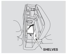
The console compartment has two shelves to divide it into two levels. To store small items, you can use the upper half of the space by putting the shelves down until they latch. The front and rear shelves can be used separately.
