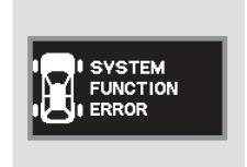
If there is a problem with the TPMS, the tire pressure monitor shows a "SYSTEM FUNCTION ERROR" message and the tire pressure readings are not displayed. If this happens, you will first see a system warning message "CHECK TPMS SYSTEM" on the multi-information display.
