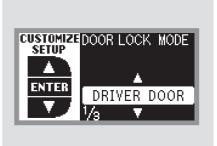
Press the SEL/RESET button. The screen changes as shown above. Select DRIVER DOOR or ALL DOORS by pressing the INFO (▲/▼) button, then press the SEL/RESET button to enter your selection.
