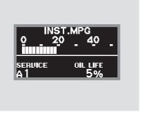
Press the SEL/RESET button on the steering wheel repeatedly to select the engine oil life. The message "SERVICE", along with "5%", and the maintenance item code are displayed on the lower part of the multi-information display when the calculated engine oil life is 1-5 percent (see page 327).
