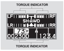
The SH-AWD torque distribution monitor on the multi-information display shows you the amount of torque being sent to the wheels. Each wheel: right front (RF), left front (LF), right rear (RR), and left rear (LR), has its own torque indicator.
