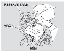
If the coolant level in the reserve tank is at or below the MIN line, add coolant to bring it up to the MAX line. Inspect the cooling system for leaks. Always use Honda Long-life Antifreeze/Coolant Type 2. This coolant is pre-mixed with 50 percent antifreeze and 50 percent water. Never add straight antifreeze or plain water.
