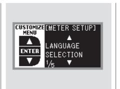
While METER SETUP is shown in the CUSTOMIZE GROUP of the multi-information display, press the SEL/RESET button. You will see the above display.
