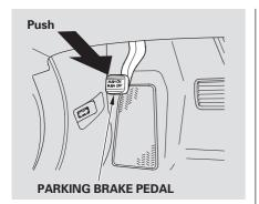
To apply the parking brake, push the pedal down with your foot. To release it, push on the pedal again. The parking brake indicator on the instrument panel should go out when the parking brake is fully released (see page 65).
