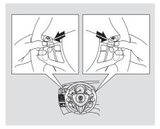
To shift up or down, use the + (right) or — (left) paddle shifter on each side of the steering wheel.
