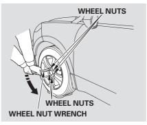
6. Loosen the five wheel nuts 1/2 turn with the wheel nut wrench.
