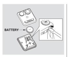
3. Place a cloth on the edge of the keypad, and remove the upper half by carefully prying on the edge with a small flat-tip screwdriver.
