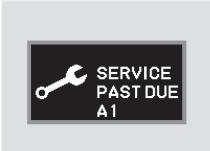
If the indicated maintenance service is not done and the remaining engine oil life reaches 0%, the multi-information display will show the message "SERVICE PAST DUE" and the maintenance item code(s). This message is displayed when the total mileage is less than 10 miles (for U.S. models) or 10 km (for Canadian models) after the engine oil life became 0%.
