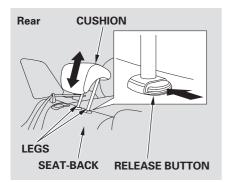
Removing the Head Restraint
