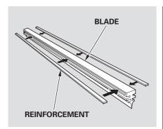
3. Examine the new wiper blades. If they have no plastic or metal reinforcement along the back edge, remove the metal reinforcement strips from the old wiper blade, and install them in the slots along the edge of the new blade.
