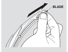
2. Slide the blade out of the wiper arm.
