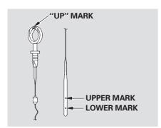
Make sure the "UP" mark on the loop is facing up when you insert the dipstick.
