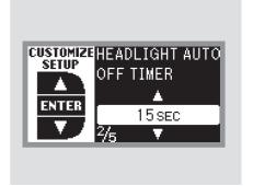
Press the SEL/RESET button. The screen changes as shown above. Select how long you want the lights to stay on before they go off (0, 15, 30, or 60 seconds) by pressing the INFO (▲/▼) button, then press the SEL/RESET button to enter your selection.
