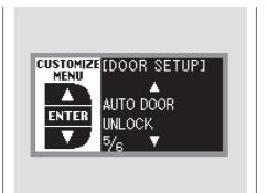
While DOOR SETUP is shown in the CUSTOMIZE GROUP of the multi-information display, press the SEL/RESET button. The screen changes to CUSTOMIZE MENU. Press the INFO (▲/▼) button until you see the above display.
