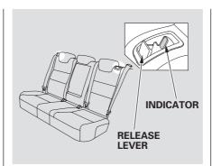
After returning the seat-back to the upright position, tug on the seat-back to make sure it is latched. If the seat-back is not latched fully, the seat belt will not work properly and you will see the red indicator behind the release lever as shown.
