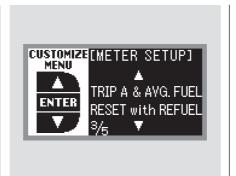
While METER SETUP is shown in the CUSTOMIZE GROUP of the multi-information display, press the SEL/RESET button. The screen changes to CUSTOMIZE MENU. Press the INFO (▲/▼) button until you see the above display.
