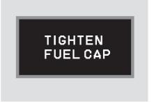
If your fuel fill cap is loose or missing, a "TIGHTEN FUEL CAP" message appears on the multiinformation display after you start the engine. Turn the engine off, and confirm the fuel fill cap is installed. If it is, loosen it, then retighten it until it clicks at least once. When you can restart the engine, the message appears again. The message goes off after several days of normal driving once you tighten or replace the fuel fill cap. To scroll to another message, press the INFO (▲/▼) button.
