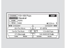
MODE — To switch between the category mode and channel mode, press and hold the DISP/MODE button until the mode changes. A "CH" (channel) or "CAT" (category) mode indicator appears on the upper display.
