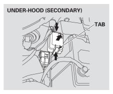
The secondary under-hood fuse box is next to the battery. To open it, push the tabs as shown.
