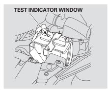
Check the condition of the battery monthly by looking at the test indicator window. The label on the battery explains the test indicator's colors. Check the terminals for corrosion (a white or yellowish powder). To remove it, cover the terminals with a solution of baking soda and water. It will bubble up and turn brown. When this stops, wash it off with plain water. Dry off the battery with a cloth or paper towel. Coat the terminals with grease to help prevent future corrosion.
