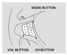
The VOL button adjusts the volume up  $(\blacktriangle)$  or down  $(\blacktriangledown)$ . Press the top or bottom of the button, hold it until the desired volume is reached, then release it.
