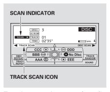
To activate scan feature on the audio control display, press the AUDIO button to view the display. Push down the selector on the interface dial, then push the selector to the left. You will see "SCAN" next to the TRACK icon on the audio control display. To turn off this feature, push the selector to the left again within 10 seconds.
