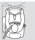
If you ever have a moderate to severe side impact, sensors will detect rapid acceleration and signal the control unit to instantly inflate either the driver's or the passenger's side airbag. Only one airbag will deploy during a side impact. If the impact is on the passenger's side, the passenger's side airbag will deploy even if there is no passenger.
