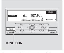
To tune with the interface dial, press the AUDIO button to view the audio control display, then push the selector down, and turn the knob to TUNE. Then press ENTER on the selector, and turn the knob to the desired frequency. To exit the TUNE mode, press ENTER again.
