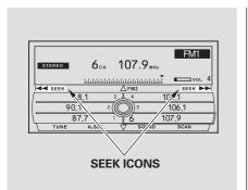
SEEK — The SEEK function searches up and down from the current frequency to find a station with a strong signal. To activate it, press the ◄ or ► side of the SEEK/SKIP bar, then release it.
