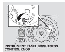
The knob on the instrument panel controls the brightness of the instrument panel lights. Turn the knob to adjust the brightness.
