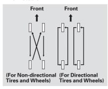
To help increase tire life and distribute wear more evenly, rotate the tires according to the maintenance messages displayed on the multi-information display. Move the tires to the positions shown in the illustration each time they are rotated. If you purchase directional tires, rotate only front-to-back.
