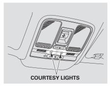
The courtesy lights in the ceiling console come on when the light switch is in the 30% or the
