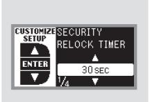
Press the SEL/RESET button. The screen changes as shown above. Select the relock time you want (30, 60, or 90 seconds) by pressing the INFO (▲/▼) button, then press the SEL/RESET button to enter your selection.
