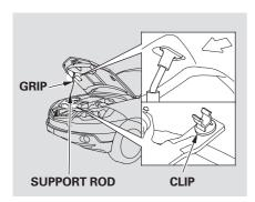
3. Holding the grip, pull the support rod out of its clip. Insert the end into the designated hole in the hood.
