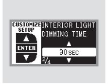
Press the SEL/RESET button. The screen changes as shown above. Select how long you want the lights to stay on before they fade out (15, 30, or 60 seconds) by pressing the INFO (▲/▼) button, then press the SEL/RESET button to enter your selection.
