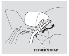
6. Lift the head restraint (see page 132), then route the tether strap through the legs of the head restraint and over the seat-back, making sure the strap is not twisted.
