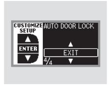
To exit AUTO DOOR LOCK without changing the current setting, select EXIT by pressing the INFO (▲/▼) button, then press the SEL/RESET button. The screen goes back to CUSTOMIZE MENU.
