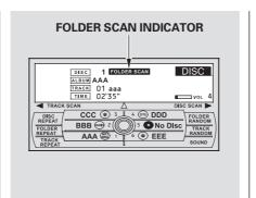
If you don't, the system advances to the next folder, plays about 10 seconds of it, and continues through the rest of the folders the same way. When the system finishes scanning all the folders on the current disc, the system returns to the folder it started scanning with, folder scan is canceled, and the system begins to play that folder normally.
