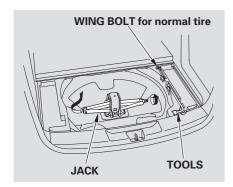
5. Remove the tools, wing bolt and the jack. To remove the jack, turn the jack's end bracket counterclockwise to loosen it.
