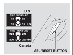
To see the inflation pressures of all four tires, press the SEL/RESET button. The display changes as shown above.
