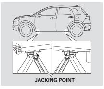
7. Place the jack under the jacking point nearest the tire you need to change. Turn the end bracket clockwise until the top of the jack contacts the jacking point. Make sure the jacking point tab is resting in the jack notch.
