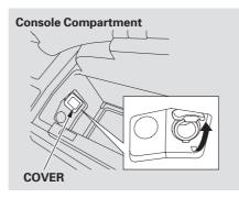
None of the sockets will power an automotive type cigarette lighter element. When both sockets are being used, the combined power rating of the accessories should be 120 watts or less (10 amps).
