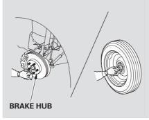
10.Before mounting the spare tire, wipe any dirt off the mounting surface of the wheel and hub with a clean cloth. Wipe the hub carefully; it may be hot from driving.
