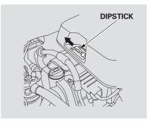
Park the vehicle on a level surface. Wait a few minutes after turning the engine off before you check the oil.
