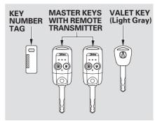
The master key fits all the locks on your vehicle. The valet key works only in the ignition and the door locks. You can keep the glove box and console compartment locked when you leave your vehicle and the valet key at a parking facility.
