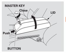
To open the console compartment, push the button and lift the lid. To close, lower the lid, and push it down until it latches.
