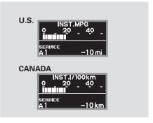
When you press the SEL/RESET button to select the engine oil life, the message "SERVICE", along with the maintenance item code and the total negative mileage after the oil life became 0 %, will be displayed on the lower part of the multi-information display.
