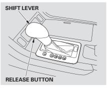
To shift from Park to any position, press firmly on the brake pedal and press the release button on the front of the shift lever, then pull the lever. You cannot shift out of Park when the ignition switch is in the LOCK (0) or the ACCESSORY (I) position.
