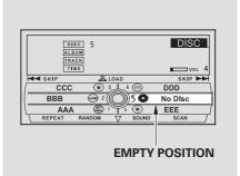
To select a disc, press an appropriate preset button (1-6), or select an appropriate preset icon by rotating the interface dial, then press ENTER on the interface selector. If you select an empty position ("No Disc" is shown) in the CD changer, the system will load a CD into the empty slot (see page 200).
