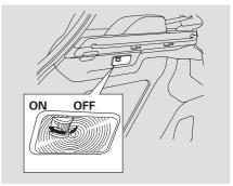
The cargo area light has a two position switch. In the OFF (right) position, the light does not come on. In the ON (left) position, the light comes on when you open the tailgate.
