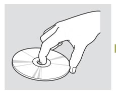
Handle a CD by its edges; never touch either surface. Do not place stabilizer rings or labels on the CD. These, along with contamination from fingerprints, liquids, and felt-tip pens, can cause the CD to not play properly or possibly jam in the drive.
