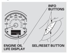
To see the current engine oil life, turn the ignition switch to the ON (II) position, and push and release the INFO ( $\triangle/\nabla$ ) button on the steering wheel repeatedly, until the engine oil life is displayed (see page 73).
