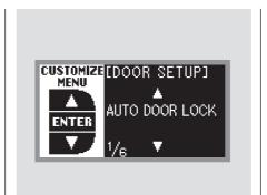
While DOOR SETUP is shown in the CUSTOMIZE GROUP of the multi-information display, press the SEL/RESET button. You will see the above display.
