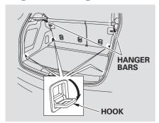
To secure the cargo, you can use the four cargo hooks in the cargo area. The illustration shows the location of each cargo hook.
