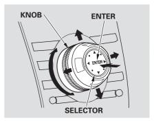
The knob turns left and right. Use it to make selections or adjustments to a list or menu on the screen.
