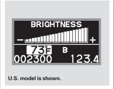
To reduce glare at night, the instrument panel illumination dims when you turn the light switch to the ₹00€ or ≣○ position.
