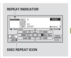
DISC REPEAT — This feature, when activated, continuously replays the current CD. Press the AUDIO button to view the audio control display, then push down the selector on the interface dial. Rotate the interface dial to select the disc repeat. Press ENTER on the selector to enter your selection. You will see "REPEAT" next to the DISC icon on the audio control display. To turn off this feature, select the disc repeat, then press ENTER again.
