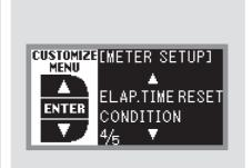
While METER SETUP is shown in the CUSTOMIZE GROUP of the multi-information display, press the SEL/RESET button. The screen changes to CUSTOMIZE MENU. Press the INFO (△/▼) button until you see the above display.
