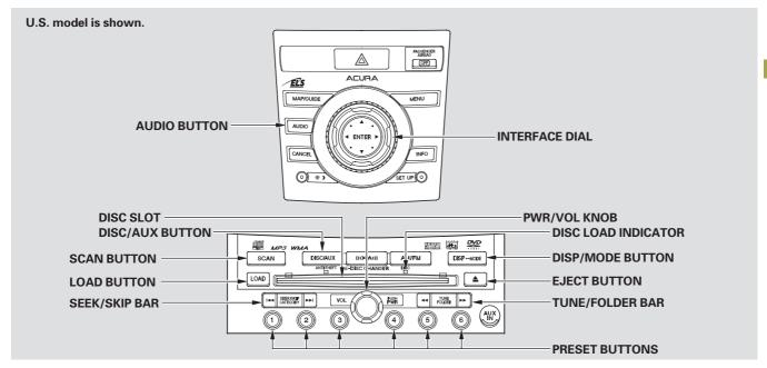
Your vehicle's audio system has an in-dash disc changer with the same controls used for the radio. To operate the disc changer, the ignition switch must be in the ACCESSORY (I) or the ON (II) position.
