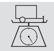
Total Trailer Weight: The maximum allowable weight of the trailer and everything in or on it must not exceed 1,500 lbs (680 kg). Towing a load that is too heavy can seriously affect your vehicle's handling and performance. It can also damage the engine and drivetrain.
