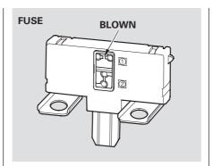
3. Check each of the large fuses in the under-hood fuse box by looking through the side window at the wire inside. Remove the screws with a Phillips-head screwdriver.
