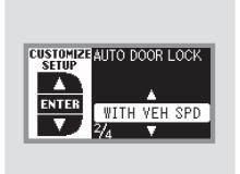
Press the SEL/RESET button. The screen changes as shown above. Select the desired setting by pressing the INFO (▲/▼) button, then press the SEL/RESET button to enter your selection.
