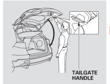
To close the tailgate, hold the tailgate handle, lower the tailgate, then press down on the back edge.
