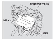
Look at the coolant level in the radiator reserve tank. Make sure it is between the MAX and MIN lines. If it is below the MIN line, see **Adding Engine Coolant** on page 340 for information on adding the proper coolant.
