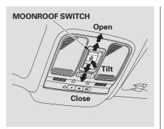
To open or close the moonroof partially, pull or push the moonroof switch lightly to the first detent and hold it. The moonroof will stop when you release the switch.
