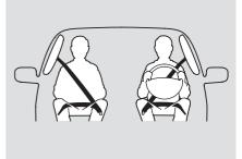
In addition, your vehicle has side curtain airbags to help protect the heads of the driver, front passenger, and passengers in the outer rear seating positions during a moderate to severe side impact or rollover (see page 30 for more information on how your side curtain airbags work).
