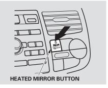
The outside mirrors are heated to remove fog and frost. With the ignition switch in the ON (II) position, turn on the heaters by pressing the button. The indicator in the button comes on as a reminder. Press the button again to turn the heaters off. Pressing this button also turns the rear window defogger on and off.
