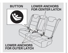
The location of each lower anchor is indicated by a small button above the anchor point.
