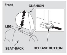
Adjusting the Head Restraint
