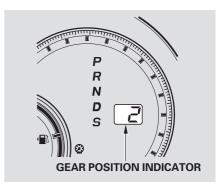
Each time you pull + (right), the transmission shifts to a higher gear. Pull - (left) to downshift. You will see the selected gear number on the instrument panel.
