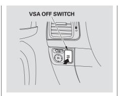
This switch is under the driver's side vent. To turn the VSA system on and off, press and hold it until you hear a beep.
