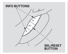
To change the display, press the SEL/RESET button or INFO (▲/▼) button on the steering wheel repeatedly until the desired information appears (see page 73).
