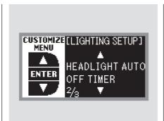
While LIGHTING SETUP is shown in the CUSTOMIZE GROUP of the multi-information display, press the SEL/RESET button. The screen changes to CUSTOMIZE MENU. Press the INFO (▲/▼) button until you see the above display.
