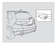
Whenever you shift to reverse (R) with the ignition switch in the ON (II) position, the rearview is shown on the navigation system screen.
