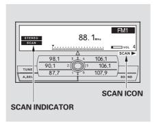
SCAN — The SCAN function samples all stations with strong signals on the selected band. To activate it, press the SCAN button, then release it. You will see "SCAN" on the upper display.
