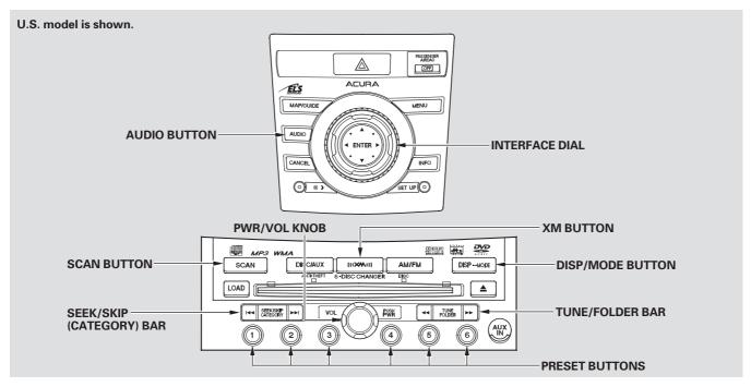
Your vehicle is capable of receiving XM® Satellite Radio anywhere in the United States, and Canada, except Hawaii and Alaska. XM® is a registered trademark of XM Satellite Radio, Inc.
