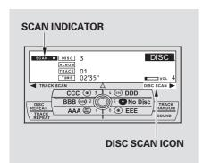
If you don't, the system advances to the next disc, plays about 10 seconds of it, and continues through the rest of the discs the same way. When the system finishes scanning all the discs, disc scan is canceled, and the system begins to play the first track/file of that disc normally.
