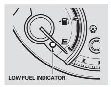
This indicator comes on as a reminder that you must refuel soon. When the indicator comes on, there is about 2.5 U.S. gal  $(9.5 \ \ell)$  of fuel remaining in the tank.
