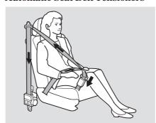
For added protection, the front seat belts are equipped with automatic seat belt tensioners. When activated, the tensioners immediately tighten the belts to help hold the driver and a front passenger in position. The tensioners are designed to activate in any collision severe enough to cause the front airbags to deploy, or if a sensor detects your vehicle is about to roll over (see page 30).
