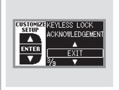
To exit KEYLESS LOCK ACKNOWLEDGEMENT without changing the current setting, select EXIT by pressing the INFO (△/▼) button, then press the SEL/RESET button. The screen goes back to CUSTOMIZE MENU.
