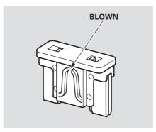
5. Look for a blown wire inside the fuse. If it is blown, replace it with one of the spare fuses of the same rating or lower. The spare fuses are provided on the back of the under-hood fuse cover.
