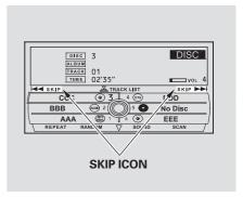
You can also change tracks/files on the audio control display. Press the AUDIO button to view the display, then push the selector on the interface dial to the right to skip forward to the beginning of the next track/file. Push the selector left to skip backward to the beginning of the current track/file. Press it again to skip to the beginning of the previous track/file.
