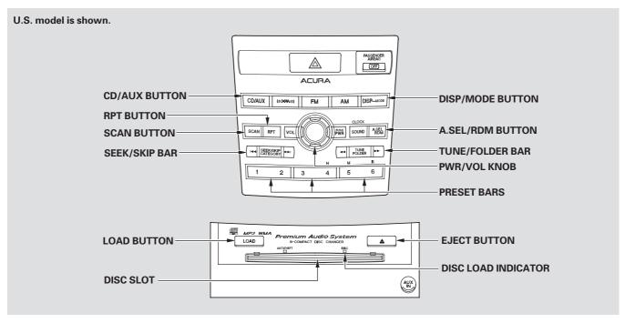
Your audio system has an in-dash CD changer that holds up to six CDs, providing several hours of continuous entertainment. You operate this CD changer with the same controls used for the radio.
