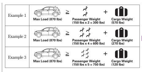
In addition, the total weight of the vehicle, all occupants, accessories, cargo, and trailer tongue load must not exceed the Gross Vehicle Weight Rating (GVWR) or the Gross Axle Weight Rating (GAWR). Both are on a label on the driver's doorjamb.
