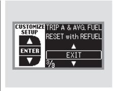
To exit TRIP A & AVG. FUEL RESET with REFUEL without changing the current setting, select EXIT by pressing the INFO (▲/▼) button, then press the SEL/RESET button. The screen goes back to CUSTOMIZE MENU.
