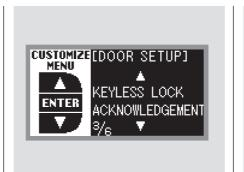
While DOOR SETUP is shown in the CUSTOMIZE GROUP of the multi-information display, press the SEL/RESET button. The screen changes to CUSTOMIZE MENU. Press the INFO (▲/▼) button until you see the above display.
