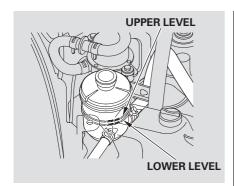
Check the level on the side of the reservoir when the engine is cold. The fluid should be between the UPPER LEVEL and LOWER LEVEL. If not, add power steering fluid to the UPPER LEVEL.
