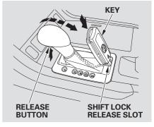
6. Remove the key from the shift lock release slot, then install the cover. Make sure the notch on the cover is on the rear.
