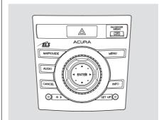
Most AcuraLink functions are controlled by the interface dial. The interface dial has two parts, a knob and a selector.
