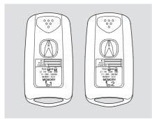
When you unlock the driver's door with your remote, each remote activates the keyless memory settings related to that remote. The driver's ID (MEMORY 1 or MEMORY 2) is shown on the back of each remote.
