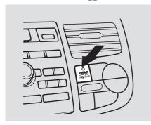
The rear window defogger clears fog, frost, and thin ice from the window. Push the defogger button to turn it on and off. Pushing this button also turns the mirror heaters on and off. The indicator in the button comes on to show the defogger is on.
