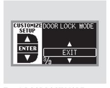
To exit DOOR LOCK MODE without changing the current setting, select EXIT by pressing the INFO (▲/▼) button, and then press the SEL/RESET button. The screen goes back to CUSTOMIZE MENU.
