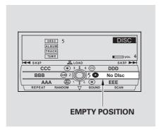
You can load a CD into an empty position while a CD is playing. Press the AUDIO button to view the audio control display. Select the empty position ("No Disc" is shown on the audio control display) by rotating the interface dial. Then press ENTER on the selector to enter your selection. The current CD stops playing and starts the loading sequence. The CD just loaded will play.
