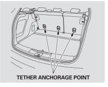
A child seat with a tether can be installed in any seating position in the back seat.
