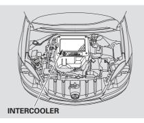
Your vehicle is equipped with a intercooler on the engine to cool the air flow from a turbo charger into the engine. The intercooler fins bend easily. Do not push them with your finger.
