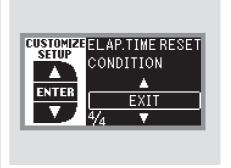
To exit ELAP. TIME RESET CONDITION without changing the current setting, select EXIT by pressing the INFO (▲/▼) button, then press the SEL/RESET button. The display goes back to CUSTOMIZE MENU.
