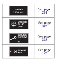
The system message(s) triggers the appropriate indicator(s) on the instrument panel, including the system message indicator, to come on. The system message indicator does not go off until the problem(s) is corrected.
