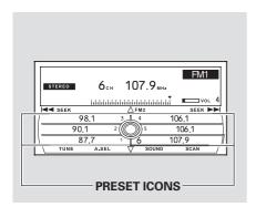
**Preset** — Each preset button/icon can store one frequency on AM and two frequencies on FM. To view the preset icons on the audio control display, push the AUDIO button.
