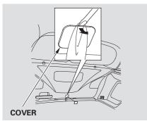
If the power door lock system cannot unlock the tailgate, unlock it manually.
