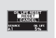
3. Press and hold the SEL/RESET button on the steering wheel for more than 10 seconds. The remaining engine oil life reset mode will be shown on the multi-information display.
