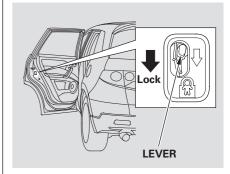
The childproof door locks are designed to prevent children seated in the rear from accidentally opening the rear doors. Each rear door has a lock lever near the edge. With the lever in the LOCK position (lever is down), the door cannot be opened from the inside regardless of the position of the lock tab. To open the door, push the lock tab forward and use the outside door handle.
