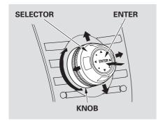
Most audio system functions can still be controlled by standard buttons, bars, and knob, but some functions can only be accessed using the interface dial. The interface dial has two parts, a knob and a selector. When you operate the audio system with the interface dial, press the AUDIO button on the control panel to display the audio control on the navigation display.
