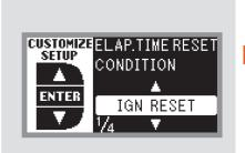
Press the SEL/RESET button. The screen changes as shown above. Select the desired setting by pressing the INFO (▲/▼) button, then press the SEL/RESET button to enter your selection.
