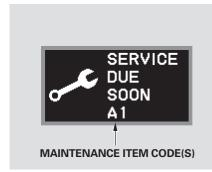
When the remaining engine oil life is 15 to 6 percent, the multi-information display shows a "SERVICE DUE SOON" message along with the maintenance schedule code indicating the main and sub items required at the time of the oil change. Refer to page 334 for a complete list of the maintenance main items and sub items.
