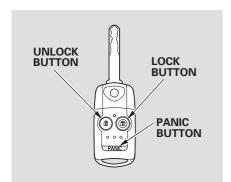
LOCK — Press this button once to lock all doors and the tailgate. Some exterior lights will flash. When you push LOCK twice within 5 seconds, you will hear a beep to verify that the doors and tailgate are locked and the security system has set. This button does not work if any door or tailgate is not fully closed.
