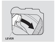
Push and hold the release lever to the right as shown, then push the tailgate to open it. If you need to unlock the tailgate manually, it means there is a problem with the tailgate. Have the vehicle checked by your dealer.
