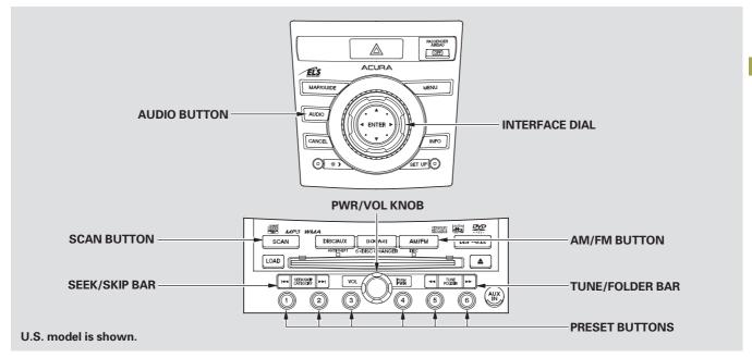
The ignition switch must be in the ACCESSORY (I) or the ON (II) position. Press the AUDIO button to view the audio control display. Turn the system on by pressing the PWR/VOL knob or the AM/FM button. Adjust the volume by turning the PWR/VOL knob.
