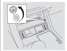
The auxiliary input jack is on the disc changer unit. The system will accept auxiliary input from standard audio accessories. When the audio system is on and you plug in a mini-jack cable between a compatible audio unit and the jack, you will see AUX in the display and the system automatically switches to AUX mode.
