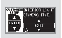
To exit INTERIOR LIGHT DIMMING TIME without changing the current setting, select EXIT by pressing the INFO (▲/▼) button, then press the SEL/RESET button. The screen goes back to CUSTOMIZE MENU.
