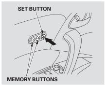
3. Press and release the SET button on the control panel. You will hear a beep. Immediately press and hold one of the memory buttons (1 or 2) until you hear two beeps. The indicator in the memory button will come on. The current positions of the driver's seat and outside mirrors are now stored.
