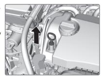
Remove the dipstick again and check the level. It should be between the upper and lower marks. Add oil if necessary.
