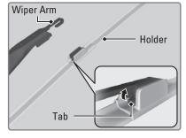
Pull the wiper blade (as shown) until it clears the end cap, then slide it out of the holder by pulling the blade up and out in the other direction.
