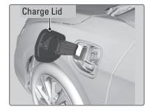
To connect the cable to the vehicle, push the cable's charge connector until it clicks to the charge lid. The charge indicator on the charge lid stays on.
