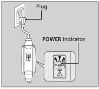
Remove the cover from the charge connector. Align and insert the charge connector into the vehicle's inlet until you hear a click. The charge indicator stops blinking, and stays on when charging starts.
