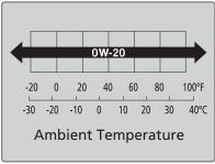
You may also use synthetic motor oil if it is labeled with the API Certification Seal and is of the specified viscosity grade.
