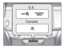
If the front passenger's seat is empty, the passenger's front airbag will not deploy and the indicator will come on.
