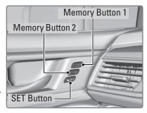
When you unlock and open the driver's door with a remote transmitter, the seat adjusts automatically to one of the two preset positions, depending on which keyless remote is present.
