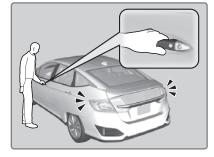
**To lock:** Press the door lock button on the front door handle when the vehicle is off. If the remote transmitter is inside the vehicle, the doors will not lock.
