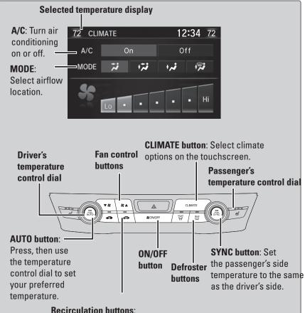
Recirculation mode (indicator on): Recirculates air from the vehicle's interior.
