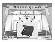
Straight top tether: Route the tether strap over the head restraint. Make sure the strap is not twisted.
