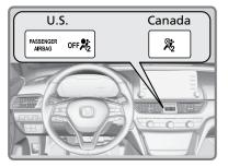
If the front passenger's seat is empty, the indicator will come on and, in the event of a crash, the front passenger's airbag will not deploy. If your vehicle is equipped with a front passenger's knee airbag, this airbag will not deploy either. To ensure the passenger is detected properly, confirm that:
