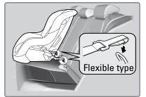
5. Tighten the tether strap according to the manufacturer's instructions.
