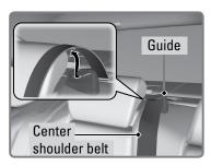
3. Push the seat-back up firmly until it locks into place to return it to its original position. Reposition the seat belts as necessary.
