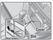
5. While pushing the key down, press the shift lever release button and place the shift lever into Neutral (N). The lock is now released. Have the shift lever checked by a dealer as soon as possible.
