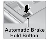
4. With the shift lever in Drive (D) or Neutral (N), press the brake pedal and come to a complete stop. The HOLD indicator appears, and brake hold is applied. Release the brake pedal.
