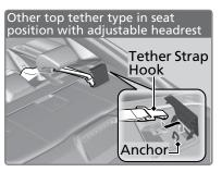
4. Tighten the tether strap according to the seat manufacturer's instructions.
