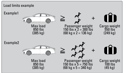
Overloading or improper loading can affect handling and stability and cause a crash in which you can be hurt or killed.
