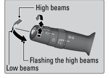
Headlights automatically\* come on after the wipers are engaged for a certain time. The headlights come on when you unlock a door in dark areas with the headlight switch in AUTO.
