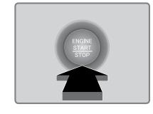
**Turning the vehicle off:** Shift to Park (P) or apply the parking brake, then press the ENGINE START/STOP button. If you press the button and the shift lever is not in Park (P), the vehicle goes into Accessory mode.
