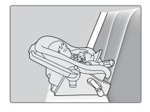
Make sure that there is no contact between the child seat and the seat in front of it. It can also interfere with proper operation of the front passenger's advanced front airbag system If this occurs, we recommend that you install the child seat directly behind the front passenger's seat, move the seat as far forward as needed and leave it unoccupied. Or you may wish to get a smaller rear-facing child seat.
