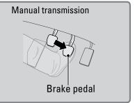
When ABS activates, you may notice vibrations through the brake pedal or the vehicle body, the brake pedal depressing further than usual, or hear a motor noise from the engine compartment. These are all normal.
