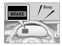
If a vehicle detected ahead of you slows down abruptly, or if another vehicle cuts in front of you, a beep sounds and BRAKE appears on the multi-information display to alert you.
