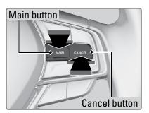
After adaptive cruise control has been canceled, you can still resume the prior set speed by pressing RES/+ when your vehicle speed is over 25 mph (40 km/h).
