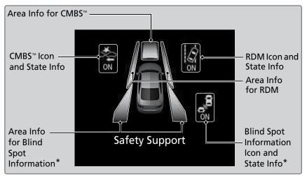
To turn the system on or off, first rotate the left selector wheel to switch displays. From the next display you can select which system to turn on or off. If the system is indicated by the amber color, have your vehicle checked by a dealer immediately. You may also confirm the state of each function by the color of the safety support indicator.
