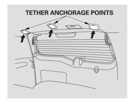
A child seat with a tether can be installed in any seating position in the back seat, using one of the anchorage points shown above.
