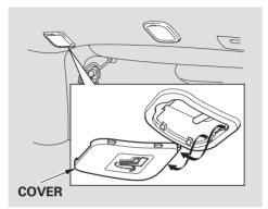
1. After properly securing the child seat (see page 43), remove the head restraint, then route the tether strap over the seat-back.
