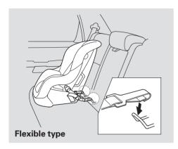
Other LATCH-compatible seats have a flexible-type connector as shown above.
