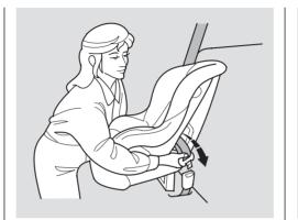
1. With the child seat in the desired seating position, route the belt through the child seat according to the seat maker's instructions, then insert the latch plate into the buckle.
