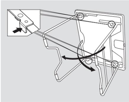
Unfold the legs. Lock them in place by pushing on the middle of the locking arms. Make sure all four are locked.
