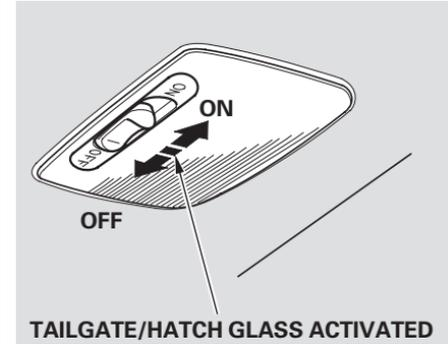
The cargo area light has a three-position switch. In the OFF position, the light does not come on. In the center position, the light comes on when you open the tailgate or the hatch glass. In the ON position, the light stays on continuously.
