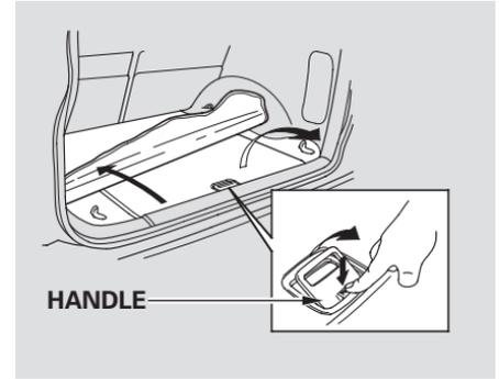
To remove the table, pull up the carpet. Lift and pull on the handle to slide the table out.
