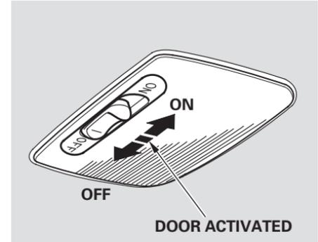
The ceiling light has a three-position switch; ON, Door Activated, and OFF. In the Door Activated (center) position, the light comes on when you:
