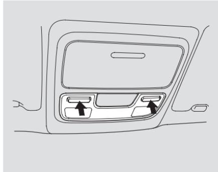
Turn on the spotlight by pushing the button. Push the button again to turn it off. You can use the spotlights at all times.
