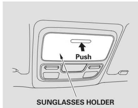
To open the sunglasses holder, push on the front edge. Make sure the holder is closed while you are driving.
