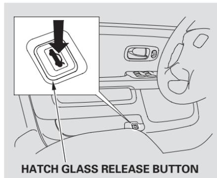
The rear wiper will not operate with the hatch glass open. If you open the hatch glass while the rear wiper is operating, the wiper will stop (see page 65).
