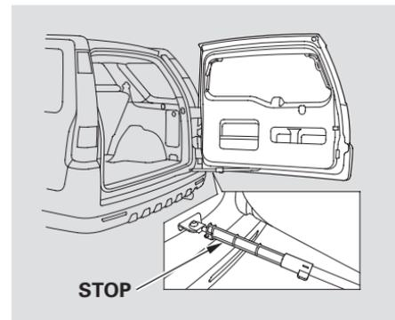
To keep the tailgate door open when facing downhill, use the stop from the tool kit.
