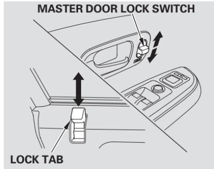
To lock the doors and the tailgate, press the master door lock switch on either front door, press the lock tab down on the driver's door, or use the key on the outside lock on the driver's door.
