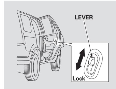
The childproof door locks are designed to prevent children seated in the rear from accidentally opening the rear doors. Each rear door has a lock lever near the edge. With the lever in the LOCK position, the door cannot be opened from the inside regardless of the position of the lock tab. To open the door, pull the lock tab up, and use the outside door handle.
