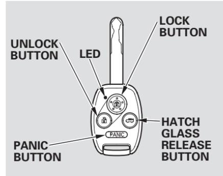
**LOCK** — Press this button once to lock all doors and the tailgate. Some exterior lights will flash once. When you push **LOCK** twice within 5 seconds, you will hear a beep to verify that the doors and the tailgate are locked. You cannot lock the doors and the tailgate if any door or the tailgate is not fully closed or the key is in the ignition switch.
