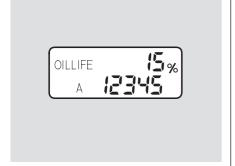
3. Press the Select/Reset knob for about 10 seconds. The engine oil life and the maintenance item code(s) will blink.
