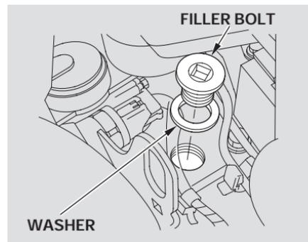
If no fluid comes out, remove the filler bolt. Slowly add Honda Manual Transmission Fluid (MTF) until it starts to run out of the check bolt hole. Let the fluid run out until it stops, then reinstall the check bolt and the filler bolt.
