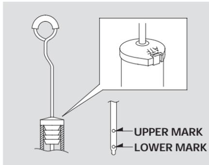
3. Insert the dipstick all the way into the transmission.
