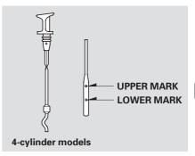
4. Remove the dipstick again, and check the level. It should be between the upper and lower marks.
