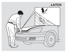
2. Put your fingers under the front edge of the hood near the center. Slide your hand to the left until you feel the hood latch handle. Push this handle up to release it. Lift up the hood.
