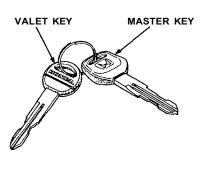
Write down the numbers stamped on both keys and keep the information in your wallet or purse in case you ever need to have duplicates made. Both the master and valet keys are double-edged, so you can insert them in the locks with either side up.
