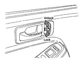
In addition, the passenger doors will lock automatically when the plunger on the driver's door is pushed down, or when the driver's door is locked from the outside with the key.
