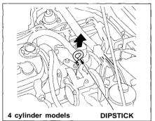
Check the engine oil a couple of minutes after shutting off the engine. This will allow the oil to drain down to the bottom of the engine. Make sure the car is parked on level ground.
