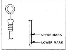
3. Pull it out again and look at the oil level at the end of the dipstick. If it is between the upper and lower marks, the level is correct. Add oil if the level is at or below the lower mark.
