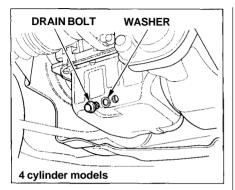
2. Open the hood and remove the engine oil fill cap. Remove the oil drain bolt from the bottom of the engine. Drain the oil into an appropriate container.
