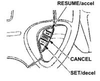
3. Press the SET/decel button on the steering wheel. The CRUISE CONTROL light on the instrument panel comes on. This shows the system is now activated.
