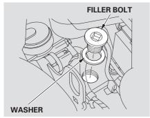
If no fluid comes out, remove the filler bolt. Slowly add Honda Manual Transmission Fluid (MTF) until it starts to run out of the check bolt hole. Let the fluid run out until it stops, then reinstall the check bolt and the filler bolt. Pour the fluid to the filler hole slowly and carefully so you do not spill. Clean up any spills immediately; it could damage components in the engine compartment.
