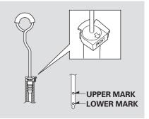
3. Insert the dipstick all the way into the transmission securely as shown in the illustration. Make sure the rubber cap on the dipstick fits in the dipstick guide and that you push the dipstick in all the way.
