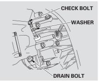
Remove the check bolt and look for transmission fluid coming out of the bolt hole. If a small amount of fluid drips out of the bolt hole, reinstall the check bolt.
