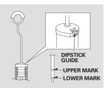
3. Insert the dipstick all the way into the transmission securely as shown in the illustration. Make sure the notch in the rubber cap fits in the dipstick guide and that you push the dipstick in all the way.
