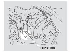
Check the fluid level with the engine at normal operating temperature.
