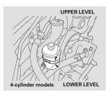
Check the level on the side of the reservoir when the engine is cold. The fluid should be between the UPPER LEVEL and LOWER LEVEL. If not, add power steering fluid to the UPPER LEVEL mark.
