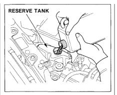
9. Refill the radiator to the base of the filler neck. Start the engine and let it run until it warms up (the radiator cooling fan comes on at least twice).
