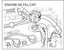
To add oil, unscrew and remove the engine oil fill cap on top of the valve cover. Pour in the oil, and replace the engine oil fill cap. Tighten it securely. Wait a few minutes and recheck the oil level. Do not fill above the upper mark; you could damage the engine.
