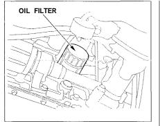
3. Remove the oil filter and let the remaining oil drain. A special wrench (available from your Honda dealer) is required to remove the filter.
