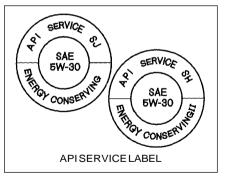
The oil container may also display the API Certification mark. Make sure it says "For Gasoline Engines."
