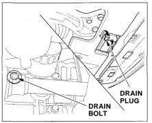
3. Loosen the drain plug on the bottom of the radiator. The coolant will drain through the splash guard. Remove the drain bolt and washer from the engine block.
