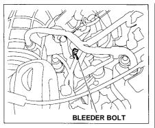
8. Loosen the bleeder bolt on top of the engine. Tighten it again when coolant comes out in a steady stream with no bubbles.
