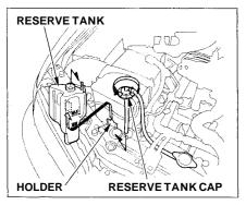
4. Remove the reserve tank from its holder by pulling it straight up. Drain the coolant, then put the tank back in its holder.
