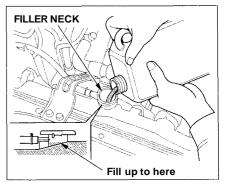
7. Pour coolant into the radiator up to the base of the filler neck.
