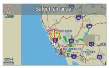
Use the **Interface Dial** to move the crosshairs to the area of the state close to your intended destination. If desired, rotate the **Interface Dial knob** to change the map scale. When you have the crosshairs in the desired area, push in on the **Interface Dial**. The address of the location you have selected will appear at the top of the screen.
