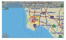
The red arrow indicates your vehicle position. Find your desired destination by moving the **Interface Dial** left, right, up, or down. The map and crosshairs will move in the same direction.
