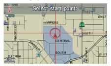
Rotate the **Interface Dial knob** to select the map scale (available scales are 1/20, 1/8, and 1/4 mile scales). Use the **Interface Dial** to move the crosshairs (red circle) to the desired start point and push in on the **Interface Dial** to "set" the start point. Then move the **Interface Dial** in a straight or diagonal direction to encompass the area to be avoided.
