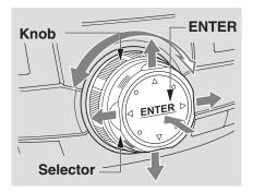
The Interface Dial moves left, right, up, and down. Use the Interface Dial to look around a displayed map. Moving the Interface Dial up or down can also be used to scroll up or down a page in a list. You can also rotate the Interface **Dial knob** to move the highlighting around the display or to scroll through a list. After making a selection in a menu or list, push in on the Interface Dial (**ENTER** button) to enter the selection into the system.
