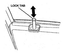
To lock any passenger's door when getting out of the car, push the lock tab down and close the door. To lock the driver's door, pull the outside door handle and push the lock tab down. Release the handle, then close the door.
