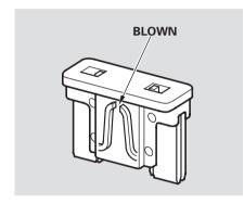
5. Look for a blown wire inside the fuse. If it is blown, replace it with one of the spare fuses of the same rating or lower.
