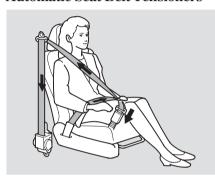
For added protection, the front seat belts are equipped with automatic seat belt tensioners. When activated, the tensioners immediately tighten the belts to help hold the driver and a front passenger in position. The tensioners are designed to activate in any collision severe enough to cause the front airbags to deploy, or if a sensor detects your vehicle is about to roll over (see page 30).
