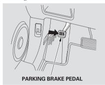
To apply the parking brake, push the pedal down with your foot. To release it, push on the pedal again. The parking brake indicator on the instrument panel should go out when the parking brake is fully released (see page 60).
