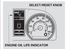
To see the current engine oil life, turn the ignition switch to the ON (II) position, then press and release the Select/Reset knob repeatedly until the engine oil life indicator appears (see page 65).
