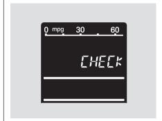
Your vehicle's onboard diagnostic system will detect a loose or missing fuel fill cap as an evaporative system leak. The first time a leak is detected a "CHECK FUEL CAP" message appears on the information display.
