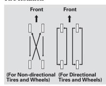
To help increase tire life and distribute wear more evenly, rotate the tires according to the maintenance messages displayed on the information display. Move the tires to the positions shown in the diagram each time they are rotated. If you purchase directional tires, rotate only front-to-back. When the tires are rotated, make sure the air pressures are checked.
