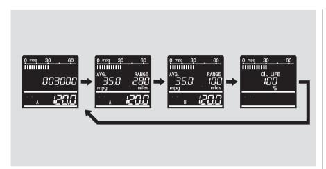
The information display consists of three segments. The upper segment displays current fuel mileage, the second segment displays the odometer, average fuel mileage, range (estimated distance), engine oil life, and the lower segment displays the trip meter, and maintenance item code(s).
