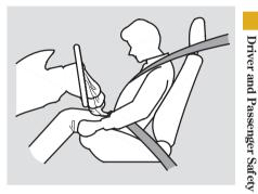
After inflating, the front airbags immediately deflate, so they won't interfere with the driver's visibility, or the ability to steer or operate other controls.
