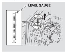
Check the fluid level by removing the cap and looking at the level gauge.
