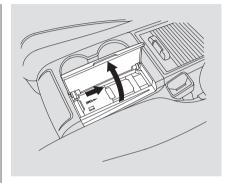
1. Open the center console cover, then slide open the CD changer cover by pulling it rearward.
