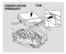
The under-hood fuse box is on the driver's side. To open it, push the tabs as shown.
