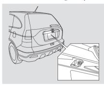
Whenever you shift to reverse (R) with the ignition switch in the ON (II) position, the rear view is shown on the navigation system screen.
