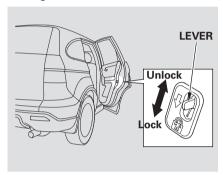
The childproof door locks are designed to prevent children seated in the rear from accidentally opening the rear doors. Each rear door has a lock lever near the edge. With the lever in the LOCK position (lever is down), the door cannot be opened from the inside regardless of the position of the lock tab. To open the door, push the lock tab forward and use the outside door handle.
