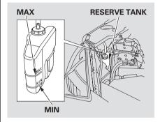
Look at the coolant level in the radiator reserve tank. Make sure it is between the MAX and MIN lines. If it is below the MIN line, see **Adding Engine Coolant** on page 270 for information on adding the proper coolant.
