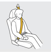
Position the lap part of the belt as low as possible across your hips, then pull up on the shoulder part of the belt so the lap part fits snugly. This lets your strong pelvic bones take the force of a crash and reduces the chance of internal injuries. If necessary, pull up on the belt again to remove any slack, then check that the belt rests across the center of your chest and over your shoulder.
