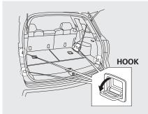
The hooks on the floor of the cargo area enable you to tie down items stored in the back. Make sure all stored items are secured before driving.
