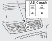
This indicator alerts you that the passenger's front airbag has been shut off because weight sensors detect about 65 lbs (29 kg) or less (the weight of an infant or small child) on the front passenger's seat. It does *not mean* there is a problem with the airbag. Be aware that objects placed on the front seat can cause the indicator to come on.
