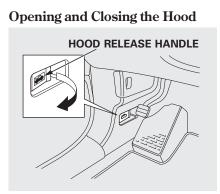
1. Park the vehicle, and set the parking brake. Pull the hood release handle located under the lower left corner of the dashboard. The hood will pop up slightly.
