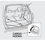
The four hooks on the side panels can be used to install a net for securing items. Each hook is designed to hold up to 50 lbs (23 kg) of weight.
