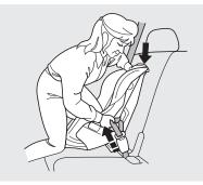
4. After confirming that the belt is locked, grab the shoulder part of the belt near the buckle, and pull up to remove any slack from the lap part of the belt. Remember, if the lap part of the belt is not tight, the child seat will not be secure.
