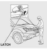
2. Put your fingers under the front edge of the hood near the center. Slide your hand to your left until you feel the hood latch handle. Push this handle up until it releases the hood. Lift up the hood.
