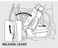
To get into the third row seats, pull up the lever on the side of the passenger's side second row seatback. The seat-back will tilt forward, and then can be slid forward.
