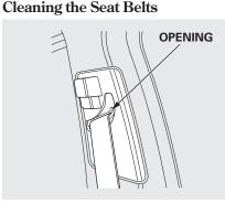
If your seat belts get dirty, use a soft brush with a mixture of mild soap and warm water to clean them. Do not use bleach, dye, or cleaning solvents. Let the belts air-dry before you use the vehicle. Dirt build-up around the openings of the seat belt anchors can cause the belts to retract slowly. Wipe the openings with a clean cloth dampened in mild soap and warm water or isopropyl alcohol.
