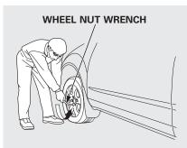
11. Loosen each wheel nut 1/2 turn with the wheel nut wrench.
