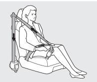
For added protection, the front seat belts are equipped with automatic seat belt tensioners. When activated, the tensioners immediately tighten the belts to help hold the driver and a front passenger in position. The tensioners are designed to activate in any collision severe enough to cause the front airbags to deploy, or if a sensor detects your vehicle is about to roll over (see page 32).
