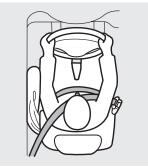
If you ever have a moderate to severe side impact, sensors will detect rapid acceleration and signal the control unit to instantly inflate either the driver's or the passenger's side airbag and activate the seat belt tensioner on the affected side. Only one airbag will deploy during a side impact. If the impact is on the passenger's side, the passenger's side airbag will deploy even if there is no passenger.
