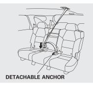
The lap/shoulder belts in the center seat of the second row and both of the third row seats are equipped with a detachable anchor that has two parts: a small latch plate and a buckle.
