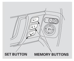
3. Press and release the SET button on the control panel. You will hear a beep. Immediately press and hold one of the memory buttons (1 or 2) until you hear two beeps. The indicator in the memory button will come on. The current position of the driver's seat is now stored.
