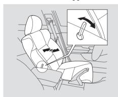
Vary the lumbar support by moving the lever on the side of the seat-back. Move the lever forward or backward to adjust the lumbar support through its full range.
