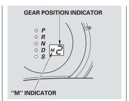
When you move the shift lever from "D" to "S" position and pull either paddle shifter, the gear position indicator displays "M" along with the selected gear number.
