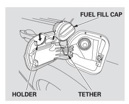
4. Remove the fuel fill cap slowly. You may hear a hissing sound as pressure inside the tank escapes. The fuel fill cap is attached to the fuel filler with a tether. Place the cap in the holder on the fuel fill door.
