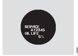
Press the SEL/RESET button on the steering wheel repeatedly to select the engine oil life. The message "SERVICE," along with "5%," and the maintenance item code are displayed on the multi-information display when the calculated engine oil life is 1-5 percent (see page 409).
