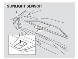
The climate control system has two sensors. A sunlight sensor is in the top of the dashboard, and a temperature sensor is next to the steering column. Do not cover the sensors or spill any liquid on them.
