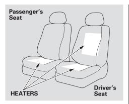
Both front seats are equipped with seat heaters. Because of the sensors for the side airbag cutoff system, there is no heater in the passenger's seat-back. The ignition switch must be in the ON (II) position to use the heaters.
