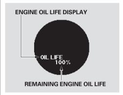
To see the current engine oil life displayed on the multi-information display, turn the ignition switch to the ON (II) position, and press the SEL/RESET button on the steering wheel repeatedly until engine oil life is displayed.
