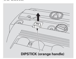
Park the vehicle on a level surface. Wait a few minutes after turning the engine off before you check the oil.
