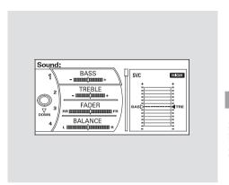
You can also adjust the sound by pushing the \( \)/ \( \) (Sound) button repeatedly. Each mode is shown in the center display as it changes. Turn the VOL/ \( \theta \) knob to adjust the setting to your liking. When the level reaches the center, you will see "C" in the display.
