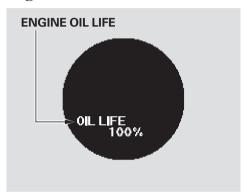
This shows the remaining life of the engine oil. It shows 100% after the engine oil is replaced and the display is reset. The engine oil life is calculated based on engine operating conditions. For more information, see page 409.
