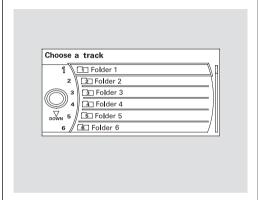
Push up the selector on the interface dial to switch the display to the folder list, then turn the knob on the interface dial to select a folder.
