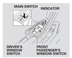
Turn the ignition switch to the ON (II) position to raise or lower any window. To open a window, push the switch down and hold it. Release the switch when you want the window to stop. Pull back on the switch and hold it to close the window.
