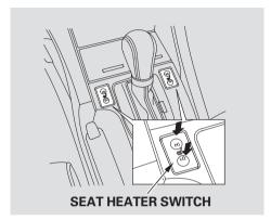
Push the front of the switch, HI, to rapidly heat up the seat. After the seat reaches a comfortable temperature, select LO by pushing the back of the switch. This will keep the seat warm.
