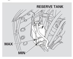
Look at the coolant level in the radiator reserve tank. Make sure it is between the MAX and MIN lines. If it is below the MIN line, see **Adding Engine Coolant** on page 423 for information on adding the proper coolant.
