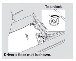
The driver's floor mat that came with your vehicle hooks over the floor mat anchors. To lock each hook, turn the knob clockwise. This keeps the floor mat from sliding forward and possibly interfering with the pedals.
