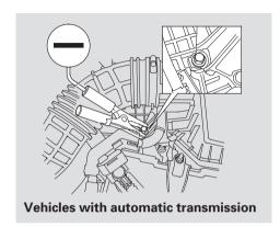
4. Connect the second jumper cable to the negative (—) terminal on the booster battery. Connect the other end to the engine mounting bolt (automatic) or the transmission mounting bolt (manual), as shown. Do not connect this jumper cable to any other part of the engine.
