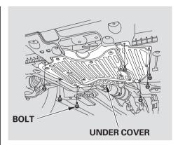
3. Remove the bolts located on the underside of the body with a wrench, then remove the under cover.
