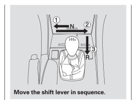
1. With the clutch pedal pressed, move the shift lever to the first/second gear side of the neutral gate, then shift to reverse.
