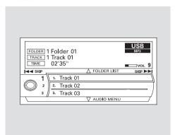
You can select any type of repeat, random and scan modes on the audio menu screen. Press the AUDIO button to show the audio control display on the navigation screen. Push down the selector on the interface dial to display the audio menu items.
