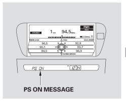
To switch the PS name display function on and off, press and release the TITLE button. With the system on, you will see the "PS ON" message on the center display. If the station you are listening to is an RDS station, the displayed frequency switches to the station name
