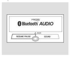
The resume/pause mode can stop playing a file temporarily. Push down the selector on the interface dial to display the audio menu.
