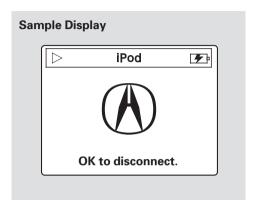
When the iPod is connected and the iPod mode is selected on the audio display, the USB and iPod indicators are shown in the display. After loading, you will see Acura mark\* on the iPod. That means you can only operate your iPod using the vehicle's audio unit.
