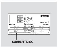
Select the changer by pressing the DISC button. The system will begin playing the last selected disc in the disc changer. You will see the current disc position highlighted.
