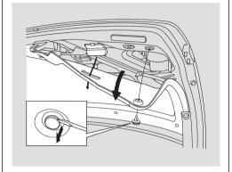
3. Pull back the appropriate corner of the trunk lid lining carefully.
