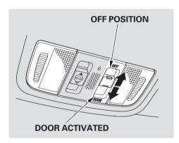
The spotlights have a two-position switch. In the DOOR position, the lights come on when you open any door. The lights fade out in about 30 seconds after the doors are closed tightly. In the OFF position, the lights do not come on.
