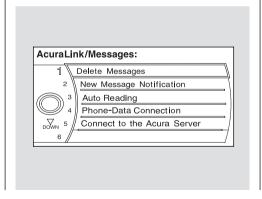
To access the following functions, press the SETUP option, push the interface selector to the right to select Other, then rotate the interface knob to select AcuraLink/ Messages.
