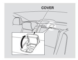
2. Pull up the cover of the tether anchor point on the left side.
