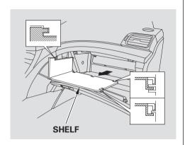
You can remove the shelf to get more space in the glove box. To remove it, open the glove box and pull out the shelf while disengaging its tabs from the glove box frame.
