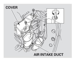
To change a bulb on the left side, remove the two fasteners by turning the head of each fastener with a flat-tip screwdriver, then remove the cover and upper part of the air intake duct.
