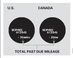
When you press the SEL/RESET button to select the engine oil life, the message "SERVICE," along with the maintenance item code(s) and the total negative mileage after the oil life became 0%, will be displayed on the multi-information display.
