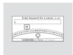
Enter the keyword for a person's name, such as the first name or last name, using the Interface Dial. If the system does not find an exact match, say or select "LIST" when you finish entering the keyword.
