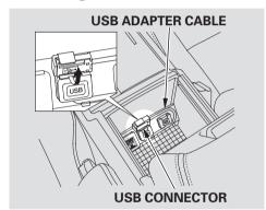
1. Unclip the USB connector by pivoting it, and pull out the USB adapter cable in the console compartment.
