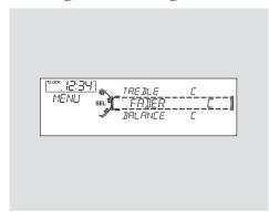
Press the MENU button to display the audio settings. Turn the selector to select a desired sound mode, then press ENTER to set your selection. Turn the selector to your liking (see page 181 for more sound setting information).
