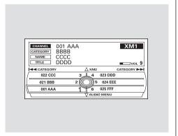
To listen to XM satellite radio, turn the ignition switch to the ACCESSORY (I) or ON (II) position, and press the (('>M')") button. The last channel you listened to will show in the audio screen and the center display. Adjust the volume by turning the VOL/ (b) knob. Push the AUDIO button to display XM information on the screen. You can operate the XM Satellite Radio system with the interface dial.
