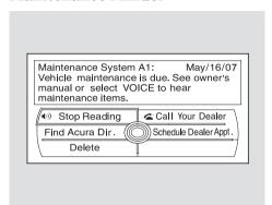
These messages provide detailed information about the service needed for your vehicle. When a maintenance message appears on the multi-information display, a list of needed maintenance items is provided through an AcuraLink message. These messages tell you the exact maintenance needed, helping you to avoid unnecessary maintenance costs.
