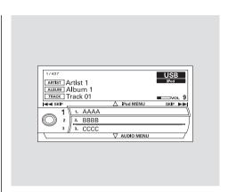
You can also change files with the interface dial. Press the AUDIO button to show the audio control display on the navigation screen. Push the selector to the right side to skip forward and to the left side to skip backward.
