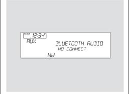
Make sure that your phone is paired and linked to the HFL. Press the AUX button\* with the ignition switch in the ACCESSORY (I) or ON (II) position. The audio display shows the Bluetooth® Audio message and mark. Until the phone is recognized, you will see "NO CONNECT" on the display. This message will go off when the phone is recognized, then the system begins to play.
