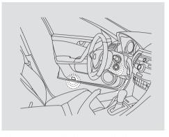
The courtesy light in each door comes on when the door is opened, and goes out when the door is closed.
