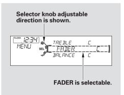
Press the MENU button to display the sound settings. Turn the selector knob to select an appropriate setting: bass, treble, fader, balance, SUBW (subwoofer), SVC (speed-sensitive volume compensation), and CLOCK ADJUST (clock adjustment). Press the selector (ENTER) knob to enter the setting, then turn the selector knob to adjust the setting.
