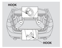
To secure cargo, use the four floor hooks in the trunk. Make sure all stored items are secured before driving.
