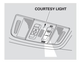
The courtesy light between the spotlights comes on when you turn the parking lights on. To adjust its brightness, turn the instrument panel brightness control knob on the dashboard, with the ignition switch in the ON (II) position (see page 115).
