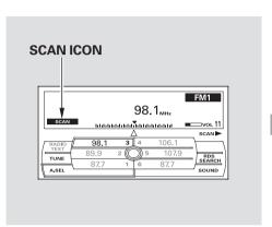
SCAN — The SCAN function samples all stations with strong signals on the selected band. To activate it, press the SCAN side of the SCAN/A.SEL bar, then release it.
