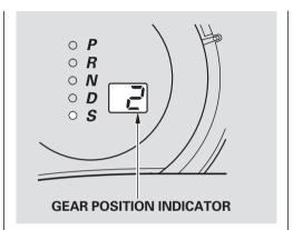
Each time you pull the + (right) paddle, the transmission shifts to a higher gear. Pull the - (left) paddle to downshift. You will see the selected gear number on the instrument panel.
