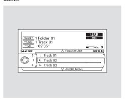
You can also select a folder or file from the list by using the interface dial. Press the AUDIO button to show the audio control display on the navigation screen.
