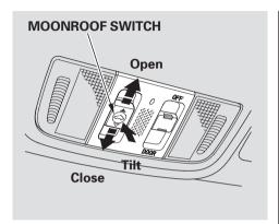
The moonroof can be tilted up in the back for ventilation, or it can be slid back into the roof. Use the switch on the front ceiling to operate the moonroof. You must turn the ignition switch to the ON (II) position to operate the moonroof.
