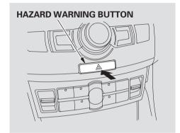
Push the button under the audio controls to turn on the hazard warning lights (four-way flashers). This causes all four outside turn signal lights and both turn signal indicators in the instrument panel to flash. Use the hazard warning lights if you need to park in a dangerous area near heavy traffic, or if your vehicle is disabled.
