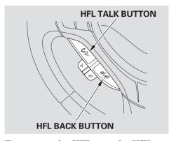
To operate the HFL, use the HFL Talk and Back buttons on the left side of the steering wheel.
