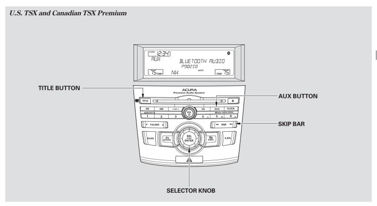
Your vehicle is equipped with a Bluetooth® audio system, which allows you to listen streaming audio from your Bluetooth audio compatible phone. This function is only available on Bluetooth Audio Compatible phones that are paired and linked to the vehicle's Bluetooth® HandsFreeLink® (HFL) system (see page 315).
