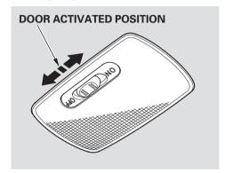
The ceiling light has a three-position switch; ON, Door Activated, and OFF. In the Door Activated (center) position, the light comes on when you:
