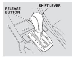
To shift from Park to any position, press firmly on the brake pedal, and press the release button on the front of the shift lever, then move the lever. You cannot shift out of Park when the ignition switch is in the LOCK (0) or ACCESSORY (I) position.
