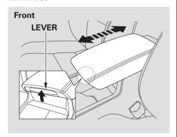
To use the console lid as an armrest, slide it to the desired position while pulling up the release lever. Release the lever to lock it in position where you want it to stop.
