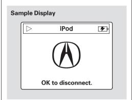
When the iPod is connected and the iPod mode is selected on the audio system, the iPod indicator is shown in the center display. If you selected the audio control display by pressing the AUDIO button, you will see the iPod and USB icons on the screen. After loading, you will see the Acura mark\* on the iPod. That means you can only operate your iPod using the vehicle's audio unit.
