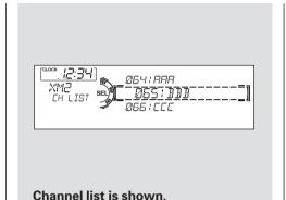
You can also select a channel or category from the list by using the selector knob. Push the selector knob (ENTER) to switch the display to the list displayed with three segments, then turn the knob to select a channel or category. Press the selector knob (ENTER) to set your selection.
