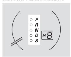
These indicators in the tachometer show which position the shift lever is in.
