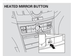
The outside mirrors are heated to remove fog and frost. With the ignition switch in the ON (II) position, turn on the heaters by pressing the rear window defogger button. The indicator in the button comes on as a reminder. Press the button again to turn the heaters and the defogger off.
