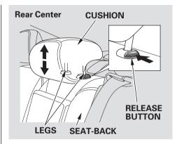
Removing the Head Restraint
