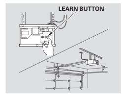
3. Press the learn button on the garage door opener unit until the indicator next to the button comes on. The indicator may blink, or come on and stay on. You then have approximately 30 seconds to complete the following steps.
