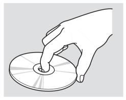
Handle a disc by its edges; never touch either surface. Do not place stabilizer rings or labels on the disc. These, along with contamination from finger prints, liquids, and feltip pens, can cause the disc to not play properly, or possibly jam in the drive.
