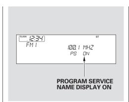
To switch the function between on and off, press and release the TITLE button. With the system on, you will see the "PS ON" message on the display. If the station you are listening to is an RDS station, the displayed frequency switches to the station name.
