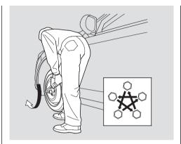
14. Tighten the wheel nuts securely in the same crisscross pattern. Have the wheel nut torque checked at the nearest automotive service facility.
