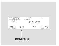
The compass may need to be manually calibrated after exposure to a strong magnetic field. If the compass seems to be continually showing the wrong direction and is not self-calibrating, or the compass display is blinking with the CAL indicator on, do the following.
