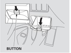
To open the driver's pocket, push the button on the lid. To close it, push the lid up until it latches.
