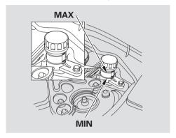
The fluid level should be between the MIN and MAX marks on the side of the reservoir. If it is not, add brake fluid to bring it up to that level. Use the same fluid specified for the brake system. A low fluid level can indicate a leak in the clutch system. Have this system inspected as soon as possible.
