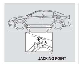
8. Place the jack under the jacking point nearest the tire you need to change. Turn the end bracket clockwise until the top of the jack contacts the jacking point. Make sure the jacking point tab is resting in the jack notch.
