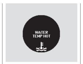
If the pointer of the temperature gauge reaches to or above the red mark, you will also see the "WATER TEMP HOT" message on the multi-information display. This will alert you that the engine should be cooled down.
