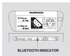
When you are operating the HFL, dialing or receiving calls with the audio system in use, you will see the above screen on the navigation display.
