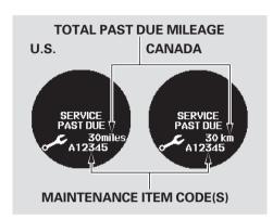
If the indicated required service is not done and the remaining engine oil life becomes 0%, the multi-information display will show a "SERVICE PAST DUE" message, the total mileage after the remaining oil life became 0%, and the maintenance item code(s).
