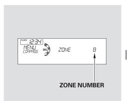
5. Once the correct zone is displayed, press the selector knob. The display then returns to normal.
