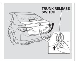
To open the trunk from the outside, push the release switch, then lift up.
