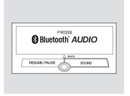
Press the AUDIO button, then push down the selector to display the audio menu. Turn the knob to switch the setting between the resume/pause mode and the sound mode. Select SOUND, then press ENTER to set your selection.
