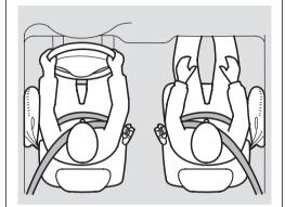
Your vehicle also has side airbags to help protect the upper torso of the driver or a front seat passenger during a moderate to severe side impact (see page 29 for more information on how your side airbags work).
