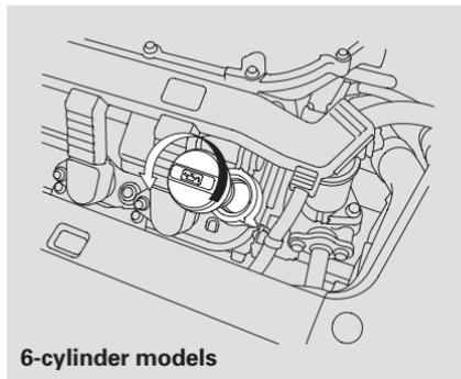
Reinstall the engine oil fill cap, and tighten it securely. Wait a few minutes, and recheck the oil level on the engine oil dipstick. Do not fill above the upper mark; you could damage the engine.
