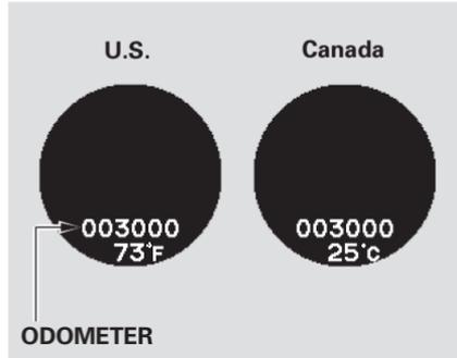
The odometer shows the total distance your vehicle has been driven. It measures miles in U.S. models and kilometers in Canadian models. It is illegal under U.S. federal law and Canadian provincial/territorial regulations to disconnect, reset, or alter the odometer with the intent to change the number of miles or kilometers indicated.
