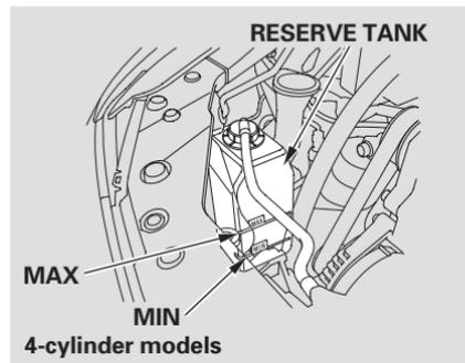
Look at the coolant level in the radiator reserve tank. Make sure it is between the MAX and MIN lines. If it is below the MIN line, see **Adding Engine Coolant** on page [420](#) for information on adding the proper coolant.
