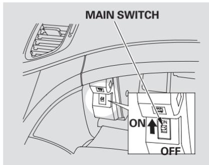
To protect items in the trunk, you can disable the trunk release button on the driver's door and the trunk release switch on the trunk lid by turning off the trunk main switch in the glove box and locking the glove box. Make sure either rear seat is not folded down.
