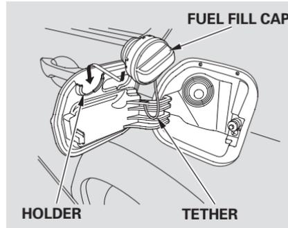
4. Remove the fuel fill cap slowly. You may hear a hissing sound as pressure inside the tank equalizes. The fuel fill cap is attached to the fuel filler with a tether. Place the cap in the holder on the fuel fill door.
