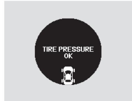
To select the tire pressure monitor, press the INFO button several times with the ignition switch in the ON (II) position.
