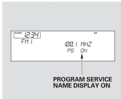
To switch the function between on and off, press and release the TITLE button. With the system on, you will see the “PS ON” message on the display. If the station you are listening to is an RDS station, the displayed frequency switches to the station name.
