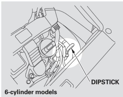
2. Remove the dipstick (yellow loop) from the transmission, and wipe it with a clean cloth.
