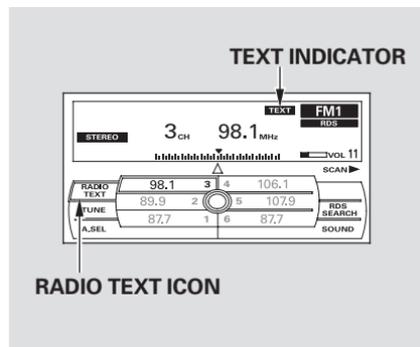
To activate radio text display, use the interface dial. Push the selector down, and turn the knob to select RADIO TEXT icon. Press ENTER on the selector to enter the setting.
