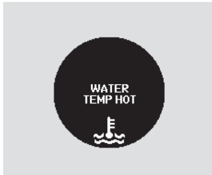
If the pointer of the temperature gauge reaches to or above the red mark, you will also see the “WATER TEMP HOT” message on the multi-information display. This will alert you that the engine should be cooled down.
