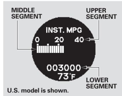
The multi-information display consists of an upper segment, a middle segment and a lower segment.
