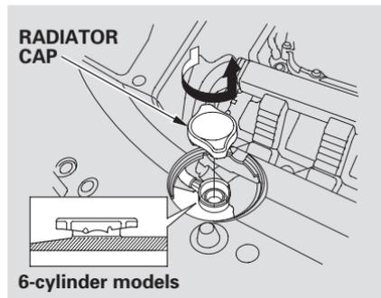
4. Remove the radiator cap by pushing down and turning counterclockwise.
