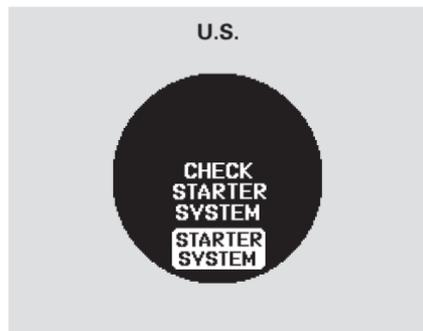
If there is a problem with the starting system, you will see a “CHECK STARTING SYSTEM” message on the multi-information display when the ignition switch is turned to the ON (II) position. You will also see this message when the auto control mode of the starting system has a problem.
