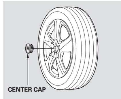
15. Remove the center cap before storing the flat tire in the trunk well.
