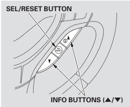
With the ignition switch in the ON (II) position, the multi-information display changes as shown on the next page each time you press the INFO (▲/▼) button or the SEL/RESET button.
