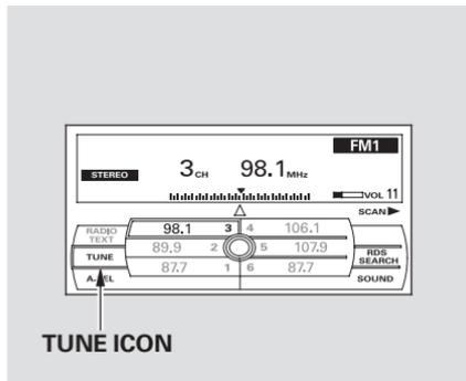
**TUNE** — Use the TUNE bar to tune the radio to a desired frequency. Press the right side of the bar to tune to a higher frequency, or the left side to tune to a lower frequency. To tune with the interface dial, push the selector down, and turn the knob to TUNE icon. Then press ENTER on the selector, and turn the knob to the desired frequency. To exit the TUNE mode, press ENTER on the selector, then push the selector up.
