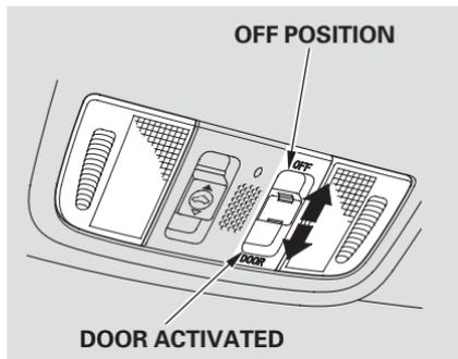
The spotlights have a two-position switch. In the DOOR position, the lights come on when you open any door. The lights fade out in about 30 seconds after the doors are closed tightly. In the OFF position, the lights do not come on.
