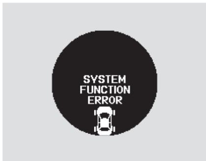
If there is a problem with the TPMS, the tire pressure monitor shows a "SYSTEM FUNCTION ERROR" message and the tire pressure readings are not displayed. If this happens, you will first see a system warning message "CHECK TPMS SYSTEM" on the multi-information display.
