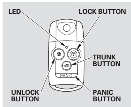
**LOCK** — Press this button once to lock all doors. Some exterior lights will flash. When you push LOCK twice within 5 seconds, you will hear a beep to verify that the doors are locked and the security system has set. You cannot lock the doors if any door is not fully closed or if the key is in the ignition switch.
