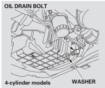
4. Remove the oil drain bolt and washer from the bottom of the engine. Drain the oil into an appropriate container.
