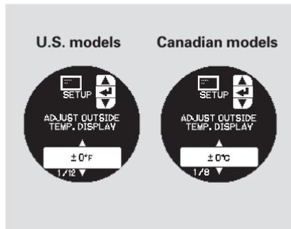
Adjust the outside temperature value by pressing the INFO (▲/▼) button repeatedly. Press the SEL/RESET button to set the desired value.
