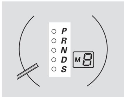
These indicators in the tachometer show which position the shift lever is in.
