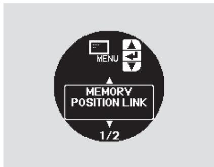
If “MEMORY POSITION LINK” is set to “ON,” the driver’s seat moves to the position stored in the memory (see page 142 ) when you open the driver’s door, using the remote transmitter.
