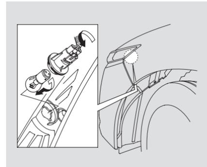
4. Remove the socket from the headlight assembly by turning it one-quarter turn counterclockwise.
