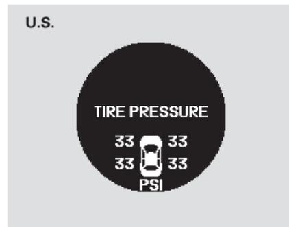
When the tire pressure monitor is shown on the multi-information display, press the SEL/RESET button. The display changes as shown.
