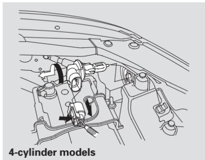
4. Remove the electrical connector from the bulb by pushing on the tab to unlock it, then slide the connector off the bulb.
