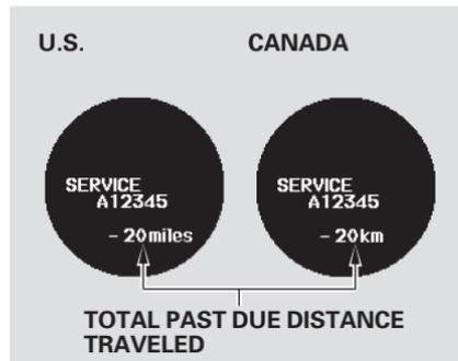
When you press the SEL/RESET button to select the engine oil life, the message “SERVICE,” along with the maintenance item code(s) and the total negative distance traveled after the oil life became 0%, will be displayed on the multi-information display.
