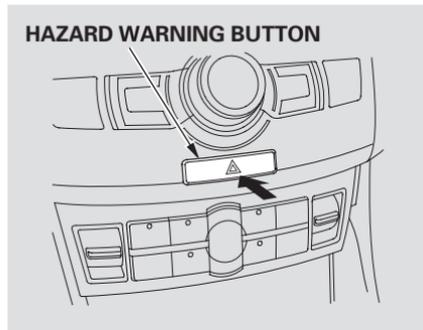
Push the button under the audio controls to turn on the hazard warning lights (four-way flashers). This causes all four outside turn signal lights and both turn signal indicators in the instrument panel to flash. Use the hazard warning lights if you need to park in a dangerous area near heavy traffic, or if your vehicle is disabled.
