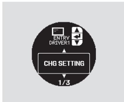
When you want to change the vehicle control settings, press the INFO (▲/▼) button to select CHG SETTING, then press the SEL/RESET button.
