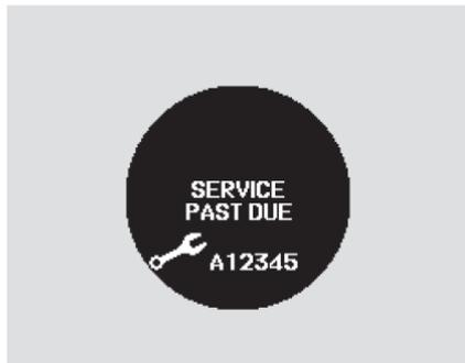
If the indicated maintenance service is not done and the remaining engine oil life reaches 0%, the multi-information display will show the message “SERVICE PAST DUE” and the maintenance item code(s). This message is displayed when the total distance traveled is less than 10 miles (for U.S. models) or 10 km (for Canadian models) after the engine oil life became 0%.
