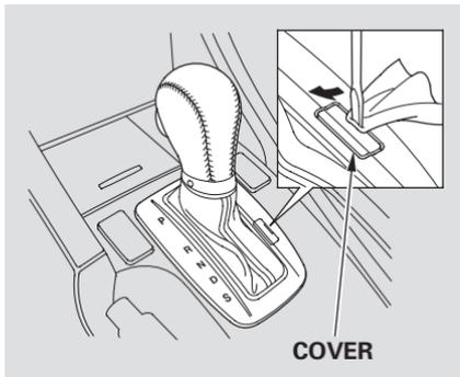
3. Put a cloth on the edge of the shift lock release slot cover to prevent scratches. Use a small flat-tip screwdriver or metal fingernail file to carefully pry up the edge of the cover and remove it from the slot.
