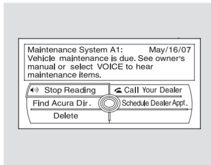
These messages provide detailed information about the service needed for your vehicle. When a maintenance message appears on the multi-information display, a list of needed maintenance items is provided through an AcuraLink message. These messages tell you the exact maintenance needed, helping you to avoid unnecessary maintenance costs.
