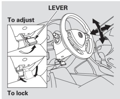
1. Pull the lever under the steering column toward you until it stops.
