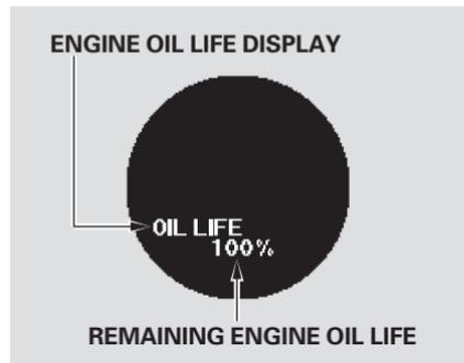
To see the current engine oil life displayed on the multi-information display, turn the ignition switch to the ON (II) position, and press the SEL/RESET button on the steering wheel repeatedly until the engine oil life is displayed.
