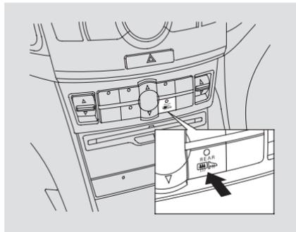
The rear window defogger will clear fog, frost, and thin ice from the window. Push the defogger button to turn it on and off. The indicator in the button comes on to show the defogger is on. It also shuts off when you turn off the ignition switch. You have to turn the defogger on again when you restart the vehicle.
