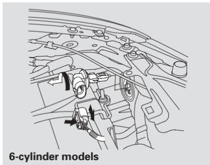
5. Remove the bulb by turning it approximately one-quarter turn counterclockwise.
