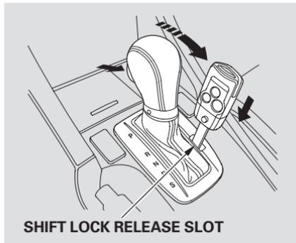
5. Push down on the key while you press the release button on the shift lever and move the shift lever out of Park to neutral.
