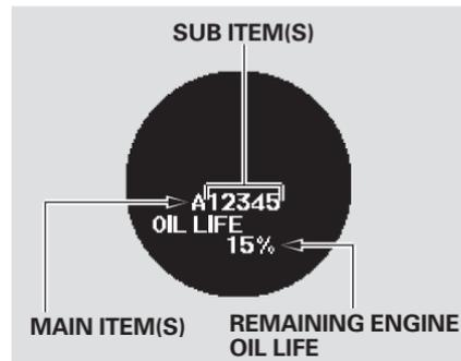
Press the SEL/RESET button on the steering wheel repeatedly to select the engine oil life information. Along with the “OIL LIFE” message, you will see the percentage of the remaining engine oil life and the maintenance item codes on the multi-information display.
