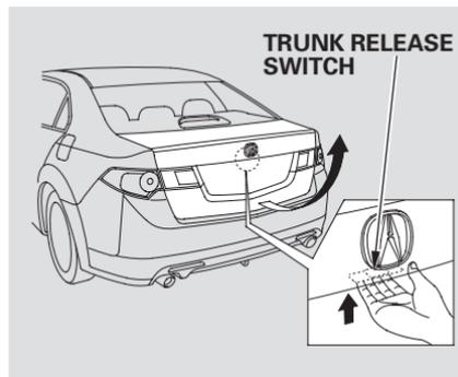
To open the trunk from the outside, push the release switch, then lift up.
