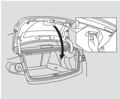
To close the trunk, use the inner handle to lower the lid, then press down on the back edge.
