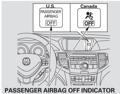
This indicator alerts you that the passenger's front airbag has been shut off because weight sensors detect about 65 lbs (29 kg) or less (the weight of an infant or small child) on the front passenger's seat. It does **not mean** there is a problem with the airbag.
