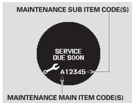
When the remaining engine oil life is 15 to 6 percent, the multi-information display shows a “SERVICE DUE SOON” message along with the maintenance item code(s) indicating the main and sub items required at the time of the oil change. Refer to page 417 for a complete list of the maintenance main items and sub items.
