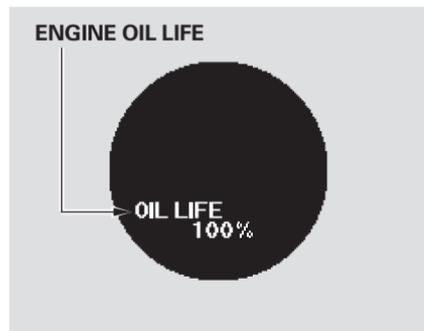
This shows the remaining engine oil life. It shows 100% after the engine oil is replaced and the display is reset. The engine oil life is calculated based on engine operating conditions. For more information, see page [403](#).
