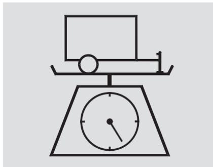
**Total Trailer Weight:** The maximum allowable weight of the trailer and everything in or on it must not exceed 1,000 lbs (450 kg). Towing a load that is too heavy can seriously affect your vehicle's handling and performance. It can also damage the engine and drivetrain.
