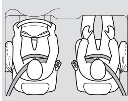
Your vehicle also has side airbags to help protect the upper torso of the driver or a front seat passenger during a moderate to severe side impact (see page [29](#) for more information on how your side airbags work).
