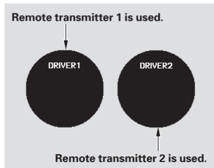
When you unlock and open the driver's door, the display shows "DRIVER 1" or "DRIVER 2" depending on which remote transmitter you use.
