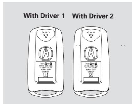
When you unlock the driver's door with your remote transmitter, each remote transmitter activates the customized settings related to that remote.
