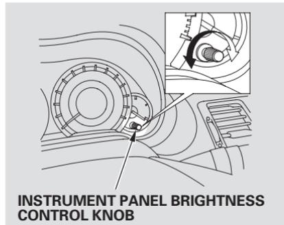
The knob on the instrument panel controls the brightness of the instrument panel lights. Turn the knob to adjust the brightness with the ignition switch in the ON (II) position and the parking lights on.
