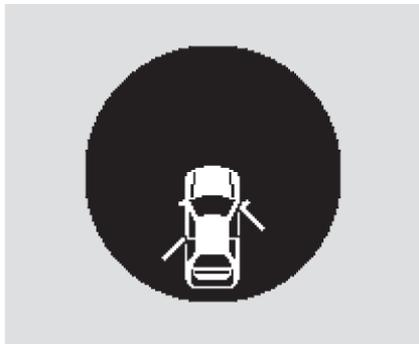
When one or more doors or the trunk lid are not tightly closed, the corresponding indicator for each condition will come on.
