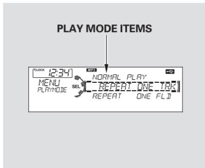
**REPEAT ONE TRK** – This feature continuously plays a file. Select normal play to turn it off. Pressing either side of the SKIP bar also turns off this feature.
