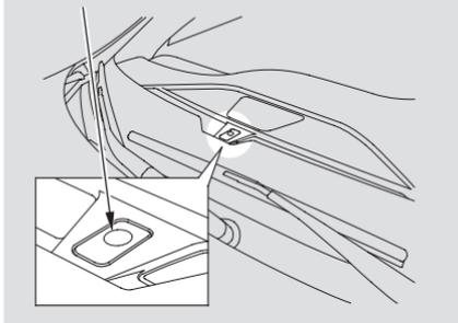
The climate control system has two sensors: a sunlight sensor on top of the dashboard, and a temperature sensor next to the steering column. Do not cover the sensors or spill any liquid on them.
