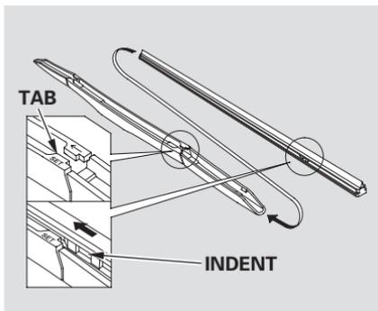
5. Place the top of the wiper blade on the end of the blade assembly, and slide the blade onto the assembly in the direction pointed to by the arrow.
