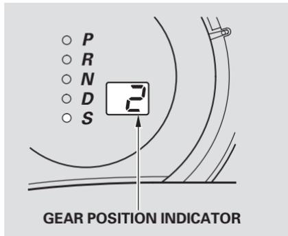
Each time you pull + (right), the transmission shifts to a higher gear. Pull - (left) to downshift. You will see the selected gear number on the instrument panel.
