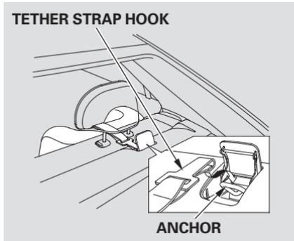
6. Route the tether strap through the legs of the head restraint and over the seat-back, making sure the strap is not twisted.
