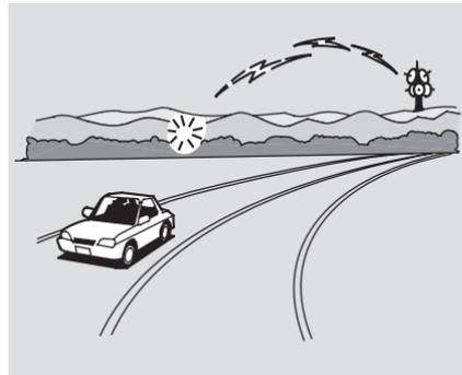
Driving very near the transmitter of a station that is broadcasting a frequency close to the frequency of the station you are listening to can also affect your radio's reception. You may temporarily hear both stations, or hear only the station you are close to.
