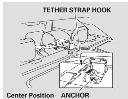
3. Lift the anchor cover, then attach the tether strap hook to the anchor, making sure the strap is not twisted.
