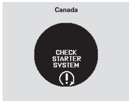
If this message is on, the ignition switch has to be held in the START (III) position manually until the engine starts. The ignition switch can be held in that position up to 15 seconds.
