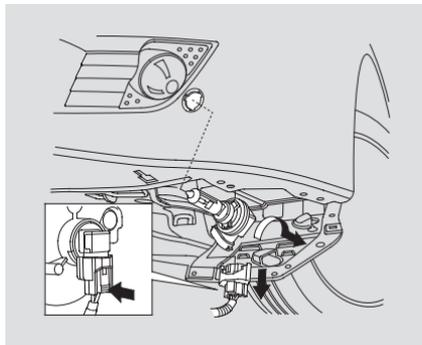
3. Remove the electrical connector from the bulb by pushing on the tab and pulling the connector down.
