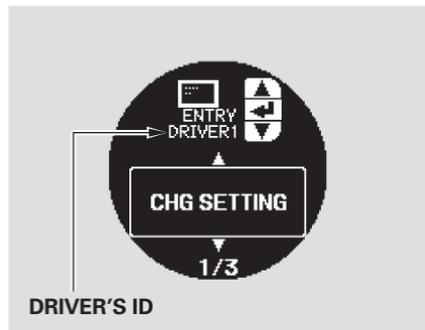
You can customize some vehicle control settings. To enter the customizing mode, press and hold either INFO button (▲/▼) for more than 3 seconds. To change the settings, the ignition switch must be in the ON (II) position, and the vehicle must be stopped with the transmission in Park (automatic) or with the parking brake set (manual).
