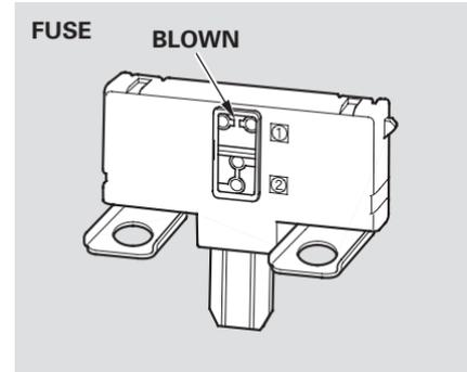
3. Check each of the large fuses in the under-hood fuse box by looking at the wire inside. Removing these fuses requires a Phillips-head screwdriver.
