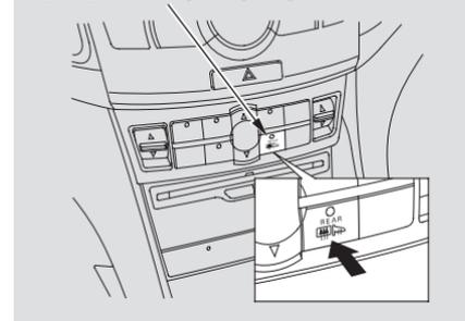
The outside mirrors are heated to remove fog and frost. With the ignition switch in the ON (II) position, turn on the heaters by pressing the rear window defogger button. The indicator in the button comes on as a reminder. Press the button again to turn the heaters and the defogger off.
