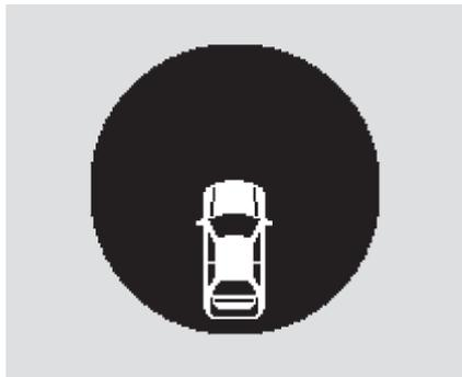
When the trunk is not tightly closed, this indicator will come on.
