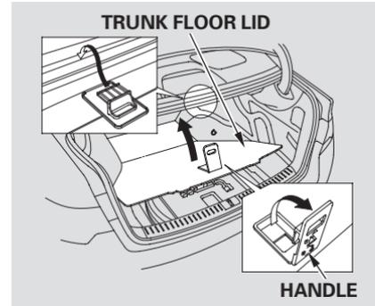
3. Open the trunk. Pull up the handle on the trunk floor lid. Raise the lid by lifting it up with the handle, then hook the handle to the trunk opening to keep the lid open.
