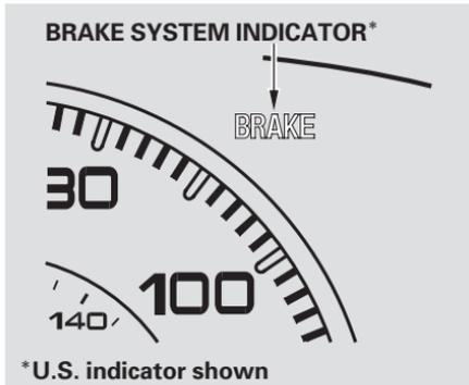
The Brake System Indicator normally comes on when you turn the ignition switch ON (II). It is a reminder to check the parking brake. It comes on and stays lit if you do not fully release the parking brake.
