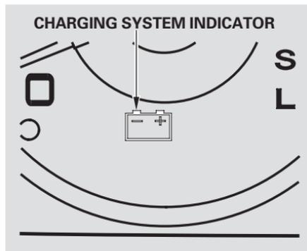
This indicator should come on when the ignition switch is ON (II), and go out after the engine starts. If it comes on brightly when the engine is running, it indicates that the charging system has stopped charging the battery.
