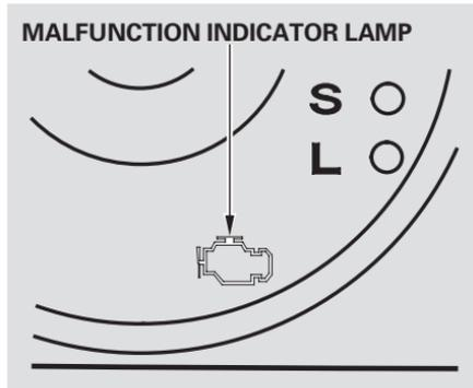
This indicator should light when the ignition switch is ON (II), and go out after the engine starts. If it comes on at any other time, it indicates one of the engine's emissions control systems may have a problem. Even though you may feel no difference in your car's performance, it can reduce your fuel economy and cause your car to put out excessive emissions. Continued operation may cause serious damage.
