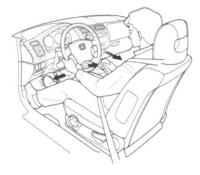
You must also press the release button to shift into Park. To avoid transmission damage, come to a complete stop before shifting into Park. The shift lever must be in Park before you can remove the key from the ignition switch.
