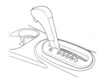
The shift lever has six positions. It must be in Park or Neutral to start the engine. When you are stopped in D, S, L, N or R, press firmly on the brake pedal and keep your foot off the accelerator pedal.
