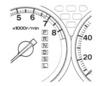
This indicator on the instrument panel shows which position the shift lever is in.
