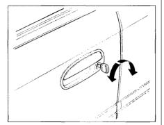
The doors can also be locked and unlocked from the outside with the key.
