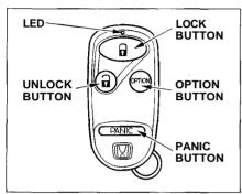
On EX model in the U.S. You can lock and unlock your vehicle with the remote transmitter. When you push the LOCK button, both doors lock.
