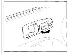
Each door has a lock tab next to the inside door handle. Push the tab in to lock the door and pull it out to unlock.
