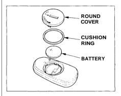
To replace the battery, remove the round cover on the back of the transmitter by turning it counterclockwise with a coin.
