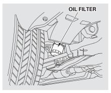
3. Remove the oil filter and let the remaining oil drain. A special wrench (available from your Acura dealer) is required to remove the filter.
