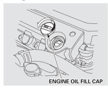
To add oil, unscrew and remove the engine oil fill cap on top of the valve cover. Pour in the oil, and install the engine oil fill cap. Tighten it securely. Wait a few minutes and recheck the oil level. Do not fill above the upper mark; you could damage the engine.
