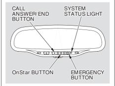
The OnStar buttons and indicator are located in the base of the rear view mirror.
