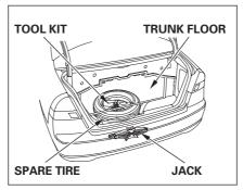
The spare tire is stored in the trunk. To remove the spare tire and the tool kit, open the trunk, and raise the trunk floor by lifting up on the back edge.
