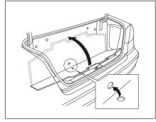
Raise the trunk floor and the lower part of the trunk lining as shown.
