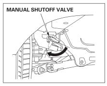
A manual shutoff valve is located underneath the vehicle, near the rear tire on the driver's side. We recommend that you locate this valve so you can find it quickly. To turn off the valve, turn the lever one-quarter turn clockwise. Turn it counterclockwise to turn the valve back on.
