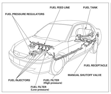
Fuel system components include a fuel tank located in the trunk, an integrated fuel pressure regulator, an in-tank fuel shutoff valve, high pressure fuel lines, electronically controlled multipoint fuel injectors, and other equipment.
