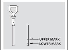
Remove the dipstick again and check the level. It should be between the upper and lower marks.
