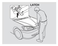
If the hood latch handle moves stiffly, or if you can open the hood without lifting the handle, the mechanism should be cleaned and lubricated.
