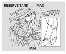
Look at the coolant level in the radiator reserve tank. Make sure it is between the MAX and MIN lines. If it is below the MIN line, see Adding Engine Coolant on page 157 for information on adding the proper coolant.
