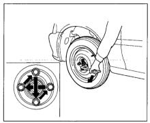
14. Tighten the wheel nuts securely in the same crisscross pattern. Have the wheel nut torque checked at the nearest automotive service facility. Tighten the wheel nuts to:
