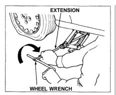
Use the extension and wheel wrench as shown to raise the car until the flat tire is off the ground.
