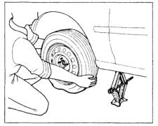
10.Remove the wheel nuts and flat tire. Temporarily place the flat tire on the ground.
