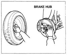
11.Before mounting the spare tire, wipe any dirt off the mounting surface of the wheel and hub with a cloth.
