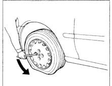
7. Loosen the four wheel nuts 1/2 turn with the wheel wrench.
