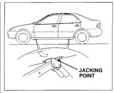
8. Locate the jacking point nearest the tire you need to change. It is pointed to by an arrow molded into the underside of the body. Place the jack under the jacking point. Turn the end bracket clockwise until the top of the jack contacts the jacking point. Make sure the jacking point tab is resting on the jack notch.
