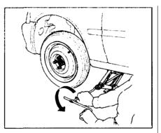
13.Lower the car to the ground and remove the jack.
