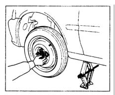
12.Put on the spare tire. Put the wheel nuts back on finger-tight, then tighten them in a crisscross pattern with the wheel wrench until the wheel is firmly against the hub. Do not try to tighten them fully.
