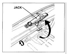
6. Turn the jack's end bracket counterclockwise to loosen it, then remove the jack.
