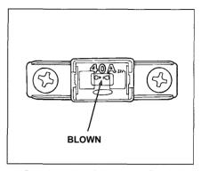
3. Check each of the large fuses in the underhood fuse box by looking through the top at the wire inside. Removing these fuses requires a Phillips-head screwdriver
