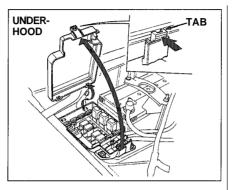
The underhood fuse box is located in the engine compartment next to the battery. To open, push the tab as shown.
