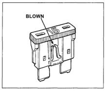
5. Look for a burned wire inside the fuse. If it is burned out, replace it with one of the spare fuses of the same rating or lower.
