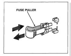
4. Check the smaller fuses in the underhood fuse box and all the fuses in the interior fuse box by pulling out each fuse with the fuse puller provided in the interior fuse box
