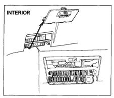
The interior fuse box is underneath the dashboard on the driver's side. Remove the fuse box lid by swinging the lid down and pulling it straight out of its hinges.
