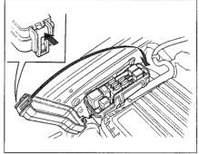
Cars equipped with ABS have a third fuse box for the ABS. It is in the front of the engine compartment on the passenger's side.
