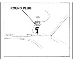
4. Use a screwdriver or coin to remove the round plug in the center of the headliner
