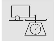
Tongue Load: The weight that the tongue of a fully-loaded trailer puts on the hitch should be approximately 10 percent of the trailer weight. Too much tongue load reduces front-tire traction and steering control. Too little tongue load can make the trailer unstable and cause it to sway.
