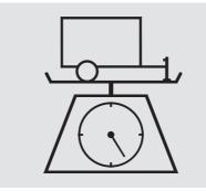
Total Trailer Weight: The maximum allowable weight of the trailer and everything in or on it must not exceed 1,000 lbs (450 kg). Towing a load that is too heavy can seriously affect your vehicle's handling and performance. It can also damage the engine and drivetrain
