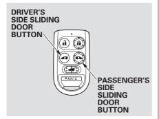
You can open or close each sliding door with the remote transmitter when the doors are unlocked. Push and hold the right button to open or close the passenger's side door, and the left button to open or close the driver's side door.
