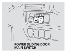
If the power sliding door MAIN switch on the dashboard is in the OFF position, you cannot open or close the sliding doors with the remote transmitter.
