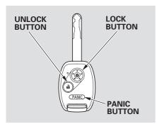
LOCK — Press this button once to lock all doors and the tailgate. Some exterior lights will flash once. When you push LOCK twice within 5 seconds, you will hear a beep to verify that the security system has set. You cannot lock the doors and the tailgate if any door or the tailgate is not fully closed or the key is in the ignition switch.
