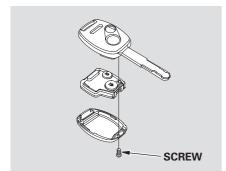
If it takes several pushes on the button to lock or unlock the doors and the tailgate, replace the battery as soon as possible.
