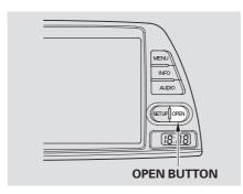
To return the screen to the upright position, press the OPEN button again. Do not use the folded screen as a tray. If you put a cup, for example, on the screen, the liquid inside the cup may spill on the screen when you go over a bump.
