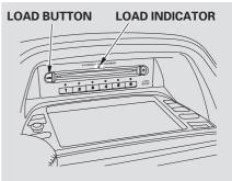
To load multiple CDs in one operation:
