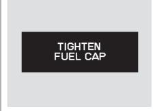
If the fuel fill cap is missing or not tightened properly, you will see "TIGHTEN FUEL CAP." Make sure the fuel cap is installed and tightened at least one click.
