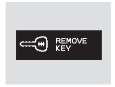
If you leave the key in the ignition switch in the LOCK (0) or ACCESSORY (I) position and open the driver's door, you will see "REMOVE KEY" in the display and hear a reminder beeper.
