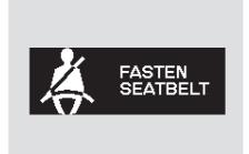
In addition to the seat belt reminder indicator on the instrument panel, the multi-information display interrupts the current display and shows "FASTEN SEAT BELT" if you do not fasten your seat belt while driving. This message remains displayed if you ignore it and do not wear your seat belt while the vehicle is moving.
