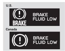
If the brake fluid level is at or below the MIN mark on the side of the brake fluid reservoir in the engine compartment, you will see "BRAKE FLUID LOW." If you see this message, have the brake system checked by your dealer (see page 379).
