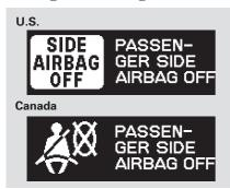
If the passenger's side airbag has automatically shut off, you will see "PASSENGER SIDE AIRBAG OFF" in the multi-information display. See page 33 for more information.
