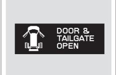
If the tailgate or any door(s) is not closed tightly, the display reminds you to close the tailgate or the door(s) before you start driving. This display continues until you close the door(s) or the tailgate. Pressing the INFO button on the steering wheel momentarily change the display to the normal display, but it will come back after 5 seconds.
