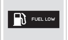
If the level of the fuel in the tank gets low, you will see "FUEL LOW" in the display, and you must refuel soon. The low fuel indicator in the instrument panel will also come on.
