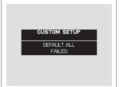
If DEFAULT ALL is not completed successfully, you will see the above display for several seconds, then the display goes back to the normal message mode. Repeat the procedure to select DEFAULT ALL.
