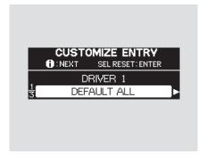
If you want to set the customizable vehicle control settings to the default setting, press the INFO button on the steering wheel until "DEFAULT ALL" is displayed, then press the SEL/RESET button.
