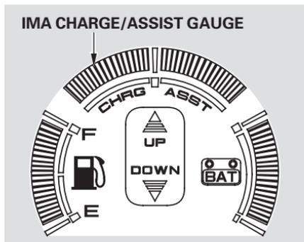
This gauge shows the status of the Integrated Motor Assist. If the indicator is on the left side of the gauge, the IMA battery is being charged. If the indicator is on the right side of the gauge, the IMA is assisting the engine.
