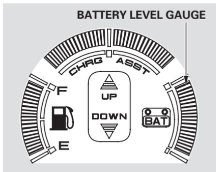
This gauge shows you the state of charge of the battery for the Integrated Motor Assist (IMA). This battery is recharged by the engine, and discharged by the IMA when it is assisting the engine with powering the vehicle.
