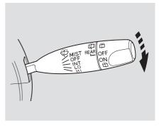
This lever controls the windshield wipers and washers. It has five positions:
