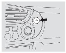
Push the button to the right of the center vents to turn on the hazard warning lights (four-way flashers). This causes all four outside turn signals and both indicators in the instrument panel to flash. Use the hazard warning lights if you need to park in a dangerous area near heavy traffic, or if your car is disabled.
