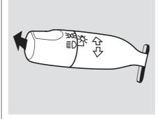
To change from low beams to high beams, push the turn signal lever forward until you hear a click. The blue high beam indicator will light (see page 49). To return to low beams, pull the turn signal lever back.
