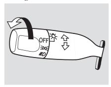
The rotating switch on the left lever controls the lights. Turning this switch to the " FOG " position turns on the parking lights, taillights, instrument panel lights, side-marker lights, and rear license plate lights. Turning the switch to the " ED " position turns on the headlights.
