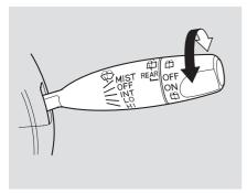
To turn on the rear window wiper, turn the ring clockwise to ON. To also use the rear window washer, turn the ring clockwise past ON. The washer will spray as long as you hold the ring in this position. If you turn the ring counterclockwise from the OFF position, the washer will spray without activating the rear window wiper.
