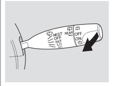
To clean the windshield, pull back on the wiper control lever. The washers spray until you release the lever.
