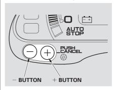
The buttons in the lower left corner of the instrument panel adjust the brightness of the display in six steps. Push the + or - button five times to see the full range.
