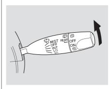
To operate the wipers in mist mode, push the control lever up from the OFF position. The wipers run at high speed until you release the lever. This gives you a quick way to clear the windshield.
