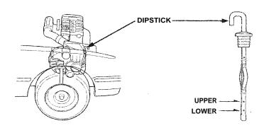
Insert the dipstick and remove it. The fluid level should be between the upper and lower marks.
