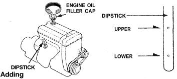
If the level has dropped close to the lower mark, add oil until it is even with the upper mark.
